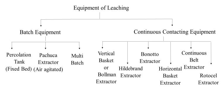
Now we will be discussing about the equipment for leaching, so there are two different types of leaching equipment like we can say extraction units also like batch equipment and we can say this continuous contacting equipment. In batch equipment say we can say percolation tank is there that is fixed bed one then Pachuca extractor unit that is air agitated one then Multi batch system also is there.
