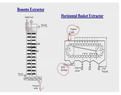
And then we have this Bonotto type extractor where we can say this one solids will be entering from here and then we can say this one extracted solid will be separated from this one bottom of this one through this conveyor belt like horizontal basket extractor also say suppose seeds will be or we can say this one feed will be entering from here and then we can say this one and or inert material will be discharged from the bottom of this we can say basket extractor.
