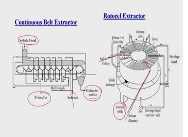
And like continuous extractor we can say this one belt type extractor, suppose this using this belt actually suppose solid feeds will be entering from here and then we can say this solvent will be supplied from this bottom of this we can say this one belt extractor and then extracted solid or we can say inert material will be separated from here.
