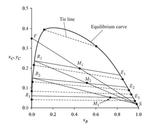
(1) Stage 1 receives the fresh feed which does not contain any solvent.
