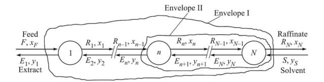
Extract and raffinate streams flow from stage to stage in countercurrent and provide two final products, Raffinate,  $R_{NP}$  and extract  $E_1$ .For a given degree of separation, this type of operation requires.Fewer stages for a given amount of solvent or loss solvent for a fixed number of stages than cross current method.
