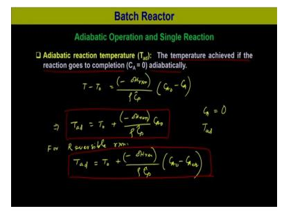
Now, from this relation, from this second relation this relation we can derive the adiabatic reaction temperature, the adiabatic reaction temperature T adiabatic if we define this is the temperature which is achieved if the reaction goes to completion that is  $C_A$  is equal to 0 adiabatically that means the temperature achieved if the reaction goes to completion
