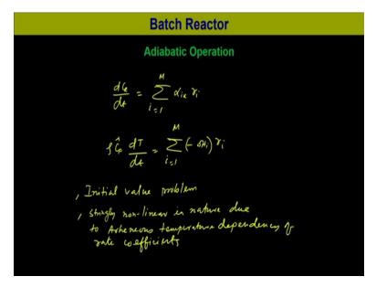
So, most of the reactors are non isothermal reactors and this is the important case which we need to consider because for adiabatic reactor when there is no heat in or heat out the adiabatic operation is often desirable because there is little utilities we need to know incorporate and it should be very easy to know operate during its normal operation.
