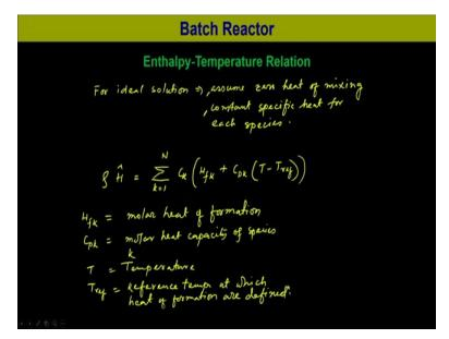
Now, if we consider 0 heat of mixing as we have considered ideal solution, so for ideal solution we can assume 0 heat of mixing and also assume constant specific heat for each
