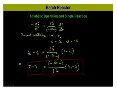
Now, if we integrate this relation, so we have  $-\frac{dC_A}{dt} = \frac{\rho C_p \frac{dT}{dt}}{(-\Delta H_{rxn})}$ , initial conditions  $T = T_0$
