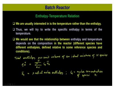
So, let us see how the enthalpy is related with the temperature, so enthalpy temperature relation. So we are ussually intrested is in the temperature rather than enthalpy and we will try to write the specific enthalpy in terms of the temperature and then we would see that the relationship between enthalpy and temperature will depend on the composition in the reactor, that means different species have different enthalpies, which is defined relative to some reference species and conditions.
