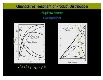
Now this can be seen, the product distribution can be seen graphically for a plug flow reactor, if
