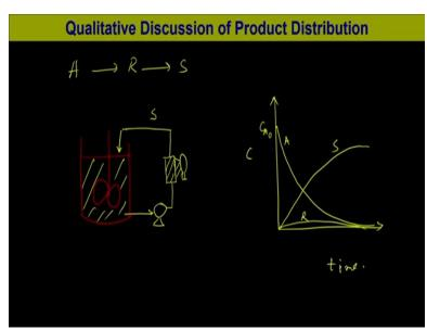
Now, if we treat this system in a different way we take a CSTR and then the content of the reactant is taken out and it is pumped through another cell where the light is put on, so light
