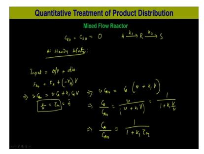
Now, let us look into the mix flow reactor, in a mixed flow reactor let us develop the concentration time curve and we start with no reactant or product presents no intermediates or product present that means  $C_{Ro} = C_{So} = 0$ . Now, if we do the material balance at steady state input would be equal to output plus disappearance due to the reaction.
