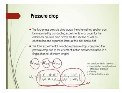
And also pressure drop is also one of the important aspect of that design of that micro channel-based reactor because based on this pressure drop there will be energy dissipation and based on that energy dissipation how that mixing is happened inside the micro channel. This is one of the important aspects there. So that is why you have to know that what should be the frictional pressure drop inside the micro channel and how to analyze and how to predict that frictional pressure drop.
