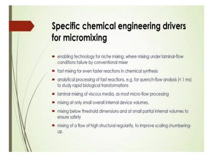
Now specific chemical engineering drivers for micro-mixing like it enables that mixing, where mixing will be under laminar flow conditions and that is failure by conventional mixer. And also in this case chemical engineering drivers for micro-mixing it will give you fast mixing for even faster reactions in chemical synthesis. Mixing at only small overall internal device volume. Mixing of a flow of high structural regularity, where that you can improve scaling and numbering up also.
