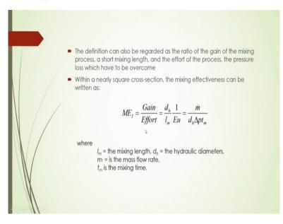
Again if you know that mass flow rate based on that mass flow rate also you can calculate with that frictional pressure drop there. So based on which you can also calculate this mixness of this effect of this micro channel mixer. And if you are having less mixing time there of course the mixness will be effectiveness of the mixing will be increased. If you have
