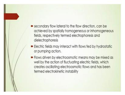
Secondary flow lateral to the flow direction can be achieved by in this case especially homogenius or inhomogeneous feelings, respectively termed as electrophoresis and dielectrophoresis. And electric fields may interact with flows fed by hydro static or pumping action. Flows driven by electro osmotic means may be mixed as well by the action of fluctuating electric fields, which creates oscillating electro osmotic flows and has been termed electro kinetic instability.
