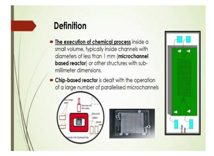
Also told that the execution of chemical process in the micro channel based reactor will be in a small volume, typically inside a channel with diameter less than 1 mm and chip based reactor is dealt with the operation of a large number of parallelized micro channel in a compact volume. (Refer Slide Time: 2:10)
