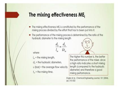
So according to the Engler et al. 2004, the mixing effectiveness is constituted by the performance of the mixing process that is divided by the effort that has been actually put into it. The performance of the mixing process is determined by the ratio of the hydraulic diameter to the mixing length as shown in the slide by this equation you can have this what should be the hydraulic diameter and mixing. And what should be the ratio of hydraulic diameter to the mixing length.
