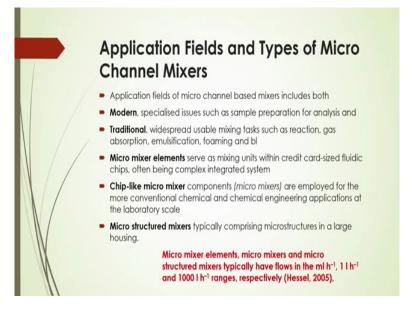
Now what are the application fields and types of micro channel based mixers there. So application field of micro channel based mixer includes both modern and traditional you can say and also you can have that micro-mixer element chip like micro-mixer, micro-structured mixers there. And chip like micro-mixer components that micro-mixers are employed for the more conventional chemical and chemical engineering applications at the laboratory scale.
