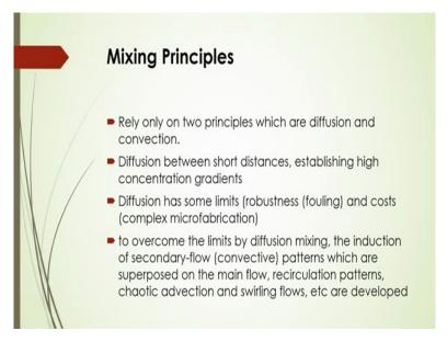
Now what are the mixing principles that in a channel whenever fluid will be flowing that two phase flow will be there? What should be that principle of mixing by different mechanism?
