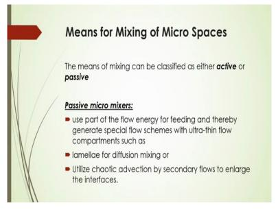
So there are two means of mixing that can be classified as either active or passive. Now passive micro-mixers means use part of the flow energy for the feeding and thereby generate special flow schemes with ultra-thin flow compartments such as Lamellae for diffusion mixing or utilize chaotic advection by secondary flows to enlarge the interfaces.
