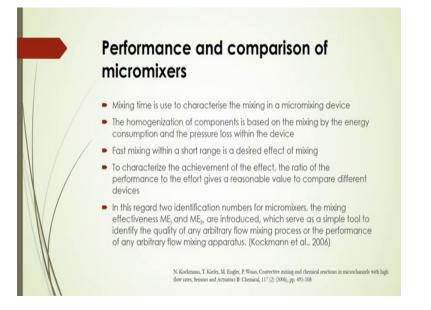
Now performance and comparison of micro-mixer of course there are several types of micromixers there. Now you have to analyze that performance or comparison of the micro-mixer and how to analyze that. So in this case mixing time is used to characterize the mixing in a micro-mixing device and the homogenization of the components that will be based on the mixing by the energy consumption and the pressure loss within the device.
