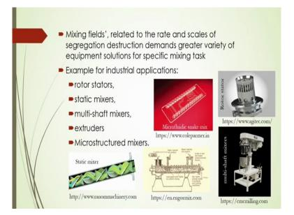
Now one important term it is called mixing fields that is related to the rate and scales of the segregation destruction demands that greater variety of equipment solutions for specific mixing task. Example for industrial applications like rotor stators type mixing equipment, static mixers, multi-shaft mixers, extruders, micro-structured mixers. So these are the different to know that device based mixing equipment for the micro-mixing in a particular devices.
