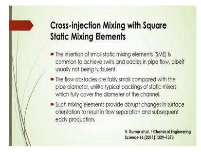
And also cross injection mixing with square static mixing elements.
