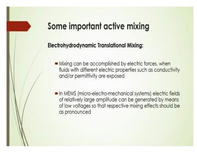
Some important active mixing like electro hydrodynamic translational mixing can be accomplished by electric forces here. When fluids with different electric properties such as conductivity and permittivity are exposed there. In micro-electromechanical systems the electric fields of relatively large amplitude can be generated by means of low voltage so that respective mixing effects can be improved or you can have that more influence to get that mixing phenomena.
