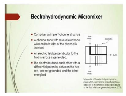
So electro hydrodynamic micro-mixer is also one of the important development of that micro-mixer for that intensification of this mixing process. In this case it generally comprises of a simple T-channel structure. In this case electric field perpendicular to the fluid interface
