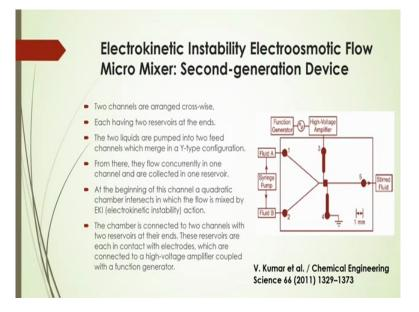
And electro kinetic instability electro osmotic flow micro-mixer this can be also enhance there. In this case channels are arranged crosswise there and while see that each having two reservoirs at the ends as shown in the figure here according to that Kumar et al. 2011 and in this case two liquids are pumped into two feed channels which merged in a Y-type configuration. And from there they flow co-currently in one channel and are collected in one reservoir.
