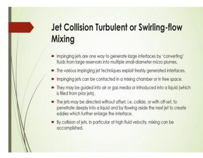
Jet collision turbulent or swirling flow mixing.
