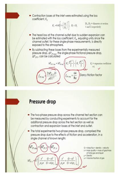
Now contraction losses at the inlet actually is estimated using the loss coefficient that is  $K_c$ . That  $K_c$  will be equal to 0.42 into 1 minus  $D_1$  by  $D_2$  the whole square.
