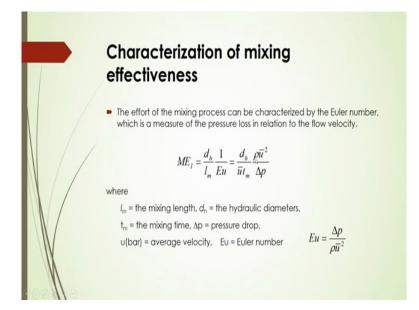
And then if that hydraulic diameter and the mixing length, effort of the mixing process can be characterized by the Euler number and with this ratio of this hydraulic diameter to the mixing length. This is a measure of the pressure loss in relation to the flow velocity. So this mixing effectiveness can be calculated by this equation if you know that pressure drop and velocity and also this hydraulic diameter and mixing time there.
