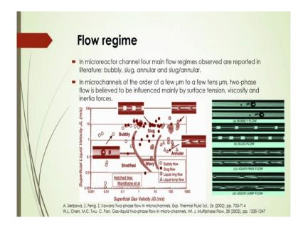
Now what are the Flow regimes in micro-reactor channel, you will see as per the reported in literature that four main regimes are generally observed: bubbly, slug, annular and slug annular flow and in micro channels of the order of a few micro-meter to a few tens micro-meter. Two phase flow is believed to be influenced mainly by surface tension, viscosity and inertia forces.
