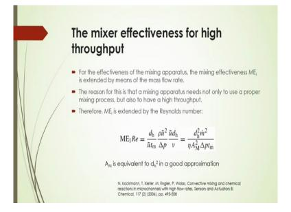
Also for high throughput devices that how to calculate that mixer effectiveness there. In this case that mixing effectiveness for that particular mixer can be extended by the Reynolds number here, as per this  $ME_1$  into Re that will be divided as  $ME_2$ . So it will be calculated by this equation as shown here in the slides there.
