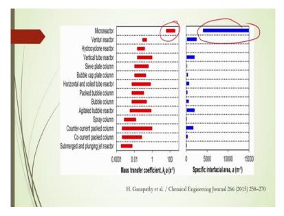
And these are some other comparison of that micro-reactor with the different mixing devices. This case you will see that very high specific interfacial area you can get for the microreactor and also mass transfer coefficient there.
