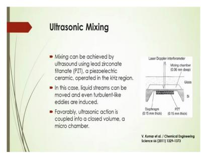
Ultrasonic mixing is also one of the important of that micro-mixing that can be achieved by ultrasound using lead Zirconate, Titanate or a piezoelectric ceramic operated in the kilo hertz region as given or reported by Kumar et al. in 2011. In this case, the liquid streams can be moved and even turbulent like eddies are induced. Favorably you can say that ultrasonic action is coupled into a close volume, a micro-chamber.
