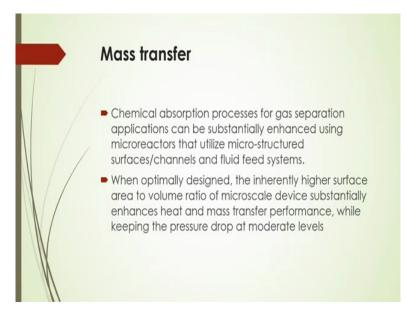
And then Mass transfer. Mass transfer of course based on this mixing characteristic that you can analyze that mass transfer, higher mixing will be of that more diffusion more that effectiveness of the mass transfer there because in this case there is no back mixing that may sometimes hindered that mass transfer efficiency but in the micro-Channel based reactor there will be no back mixing. So in that case you can increase the mass transfer by this channel.
