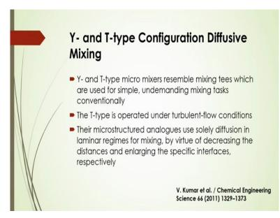
Y- and T type configuration diffusive mixing.
