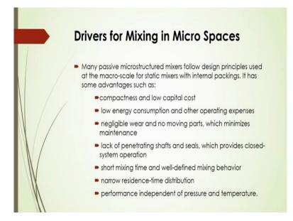
Now what should be the drivers for that mixing in micro spaces? We are talking about the micro channel based reactor, suppose in that very small volume or micro spaces you can say that many passive micro-structured mixers that follow design principles used at the macro scale for static mixers with internal packings. It has some advantages, some compactness and low capital cost, low energy consumption and other operating expenses, lack of penetrating shafts and seals there.
