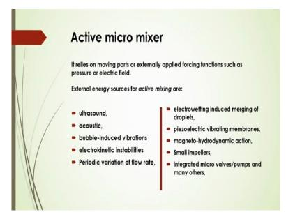
So other also principles of having that micro-mixing like it is called as active micro-mixing process. And it relies on moving parts externally applied force that will give fluctuations in that fluid elements based on which there will be intensified mixing in the fluid device. So that is why external energy gives you that micro-mixing and that is why it is called as active micro-mixing process.
