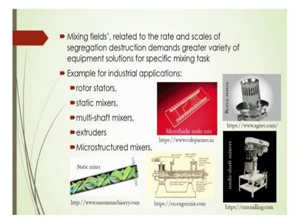
That we have discussed in the field like rotor stators, static mixers, multi-shaft mixers, extruders, micro-structured mixers so in this industrial application of different type of micromixers based on different principles how it will be working that we have to know.
