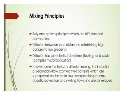
Because if you are considering different types of micro-mixers that whether this diffusion process will be enhanced or not. Whether that limits of the diffusion mixing will be improved or not. Whether there will be other types of flow produced or not. Whether it will be that secondary flow or convective flow patterns are imposed on that channels or not, what will be the superposed capacity of the flow on the other flow of this other liquid-liquid, is there any recirculation patterns or not?
