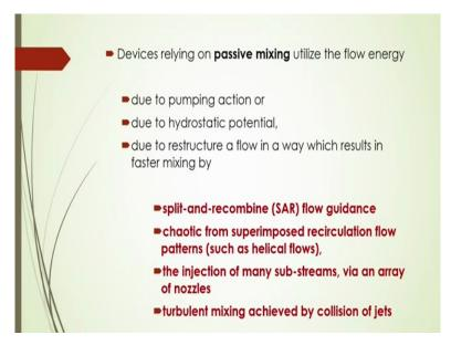
Now devices that rely on passive mixing utilize the flow energy may be due to the pumping action, due to hydro static potential, due to restructure a flow in a way which results in faster mixing by some different means like you can get passive mixing by split and recombine of the flow and also you can have that by chaotic from the superimposed recirculation flow pattern. You can have that mixing by the injection of many sub streams, via an array of
