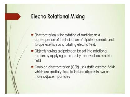
Also electro rotational mixing is one of the important other mixing principles thereby which you can have that micro-mixing inside the micro-reactor. In this case electro rotation is done as a consequence of the induction of dipole moments and torque exertion by rotating electric field. And in this case the coupled electro rotation uses static external feeds which are spatially fixed to induce dipoles in two or more adjacent particles there.
