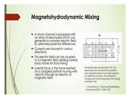
Also magneto hydrodynamic mixing also another important mechanism by which you can have that micro-mixing. In this case a micro channel is equipped with an array of electrodes which can generate a complex electric field, by alternate potential differences. In this case the currents are induced in various directions. And the electric field that can be coupled to a magnetic field that will yield you that some Lorentz body forces for the liquid mixing.
