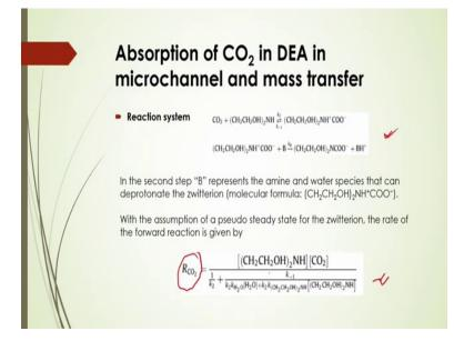
So here some reaction systems of the absorption of carbon dioxide in a diethylamine in micro channel and its mass transfer here as per reactions how that reactive mass transfer will happen with that carbon dioxide to that diethylamine and in this case, based on this you can say what will be that absorption rate there that can be calculated by this equation.
