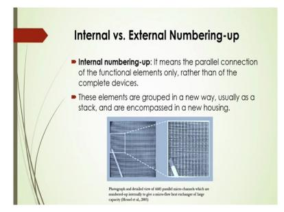
Whereas internal numbering up it will give you functional elements only rather than of the complete devices that will be connected parallel. In this case the functional elements are grouped in a new way, usually as a stack encompassed in a new housing there. So here you see, as shown figure in the slide that is there that how you will see the internal numbering up is there.
