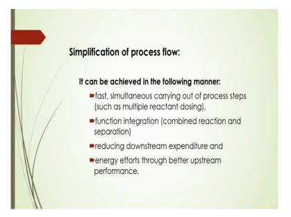
And also the simplification of the process flow you can get by the following manner like this here given in the slides. First you have to consider the simultaneously carrying out of the process steps such as multiple reactant dosing even how it will be function whether it will be integrating way or only single just entity there. So generally integration process is more favorable for that process intensification.
