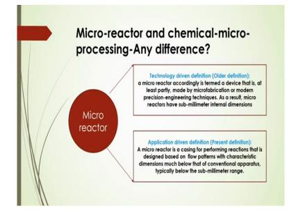
Now question is that is there any difference of micro reactor and the chemical micro processing or not? In earlier stage there is that, as per earlier definition that micro processing actually it is regarded as Technology driven definition of micro reactor. In that case micro reactor accordingly is termed a device that is at least partly made by micro fabrication or you can say that modern Precision engineering techniques. As a result that micro reactors have some millimeter internal dimensions.
