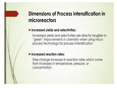
Now what are the dimensions of process intensification in micro-reactors? There are several aspects of process intensification in micro-reactors. Now it may be that increased yields and selectivities based on increase reaction time. Maybe based on reaction rate, maybe based on some safety issues, some economic consideration whether it is eco-friendly or not, different aspects of process intensification in the micro-reactor that is to be considered.
