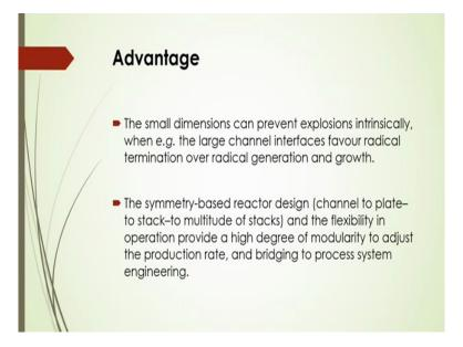
Also other advantages like the small dimensions can prevent explosions intrinsically and also you can say that the symmetry-based reactor design that is channel plate to stack to multitude of stacks and the flexibility in operation that provide a high degree of modularity to adjust the production time and also production rate and bridging to the process system engineering.
