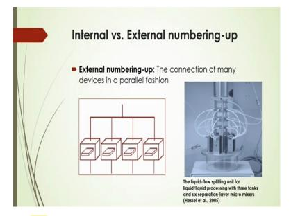
Now there may be two types of numbering up, one may be that internal another maybe external numbering up. In case of external numbering up the correcting of many devices in a parallel fashion that will give you external numbering up but in a single reactor there may be more than one channels will be arrayed but this external means there are connections of many devices here they are in a parallel fashion.
