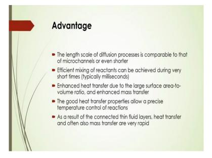
Now what are the advantages of that micro-reactor that we have to know that based on which that maybe interest is growing up day by day? Now the length scale of the diffusion processes is comparable to that of micro-channels or even shorter, so this is one aspect. Even you can get the efficient mixing of the reactants that can be achieved during very short times typically milliseconds.
