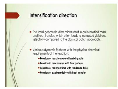
Now the small geometric dimensions that may result in an intensified mass and heat transfer which often leads to increase that yield and selectivity that is compared to the classical batch operation. Now various dynamic features to be considered when you will apply this micro-reaction technology. Now what are those dynamic features with the physicochemical requirements of the reaction that should be considered?
