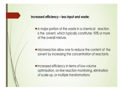
Now this micro-process technology for the process intensification, another important dimensions to be considered like how to increase that efficiency less input and waste. So in that case the major portion of the waste in a chemical reaction is a solvent, which typically constitutes 90 percent or more of the overall mixture and this micro-reactors that also allow one to reduce the content of the solvent by increasing the concentration of reactance.
