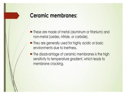
And also we can have other type of materials like ceramic type of membranes and these are made of metals like aluminum or titanium and also non-metal oxides like oxide, nitride and Carbide, this type of nonmetals are being used along with aluminum and titanium. So this is called that ceramic membranes they are generally used for highly acidic or basic environments due to inertness.
