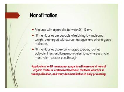
And also we will see another type it is called Nanofiltration. It is a more reduced pore size of the membrane and in that case it is procured with a pore size between 0.1 to 10 nanometers and this type of membranes are capable of retaining very low molecular weight compound and it is also used for retaining uncharged solutes like sugars and other organic molecules.
