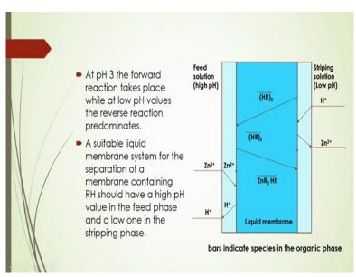
And in that case that at pH 3 the forward reaction that takes place while at low pH values the reverse reaction predominates as per shown in the figure in the slides and in that case a suitable liquid membrane system for the separation of a membrane containing RH should have a high pH value in the feed phase and a low one in the stripping phase should be there.
