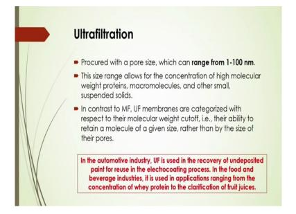
And we procured with a pore size which can range from 1 to 100 nanometer that is called Ultra filtration and this size range allows for the concentration of high molecular weight proteins, even macromolecules and other small suspended solids. So this type of ultrafiltration are being used for this type of separation processes and in contrast to microfiltration this ultrafiltration membranes are actually categorized with respect to their molecular weight cut-off.
