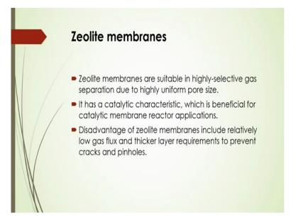
Another one important membrane it is called Zeolite membrane this type of membranes are generally used for highly selective gas separation due to highly uniform pore size and it has a catalytic characteristic which is beneficial for catalytic membrane reactor applications but there is a disadvantage like it includes relatively low gas flux and thicker layer requirements to prevent cracks and you can say that it is called Pinholes.
