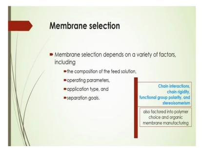
Now there are several different types of membranes, how to actually select that membrane? It can be actually based on several factors like the composition of the feed solution, even operating parameters, application type and the separation goals. In that case chain interactions, chain rigidity, functional group polarity and you can say that stereoisomerism also factored into polymers choice and organic membrane manufacturing system.
