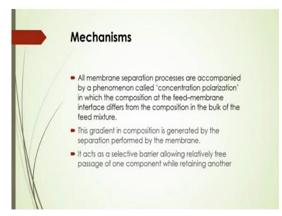
So what is the mechanism for that? So all the membrane separation processes are accompanied by phenomenon that is called concentration, polarization in which the composition at the feed membrane interface that will differ from the composition in the bulk of the feed mixture and the gradient that is in the composition is generated by the separation that is performed by the membrane.
