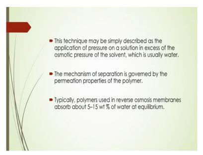
And this technique may be simply described as the application of pressure on a solution in excess of osmotic pressure of the solvent which is usually water and this mechanism of separation by reverse osmosis membrane is governed by the permeation properties of the Polymer and different types of polymers actually are being used for procuring this type of reverse osmosis membranes.
