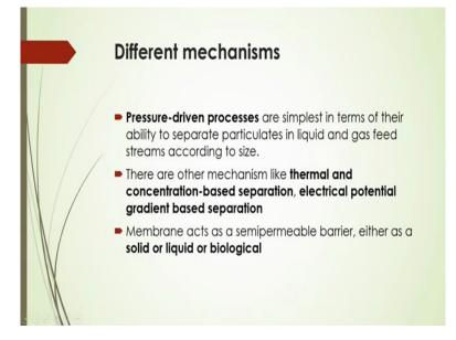
So in this way we can say that not only this concentration or gradient there will be other mechanism of having this transfer of molecules from feed to the permeate side of this membrane. So pressure driven process are the simplest in that case which in terms of their ability to separate particulates in the liquid and gas feed stream is according to size.
