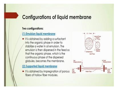
And there are also two types of configuration of this liquid membrane like it is called emulsion liquid membrane, it is obtained by adding a surfactant into the organic phase in order to stabilize water in oil emulsion and also this emulsion is then dispersed in the feed so that the organic phase which is continuous phase of the dispersed like globules that becomes the membrane as shown in figure here.
