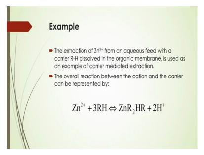
Example like that extraction of zinc ion from an aqueous feed with a carrier **RH** dissolved in the organic membrane which is used as an example of Carrier mediated extraction and the overall reaction between the cation and the carrier that can be represented by this equation that is given in the slide.
