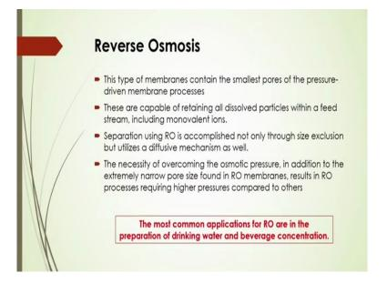
And another important aspects of that membrane separation it is called reverse osmosis. In this case you will see that this type of membrane contain the smallest pores of the pressure driven member processes and in this case you will see the separations will be based on that reverse osmosis which is accomplished not only through the size exclusion but utilizes a diffusive mechanism there.
