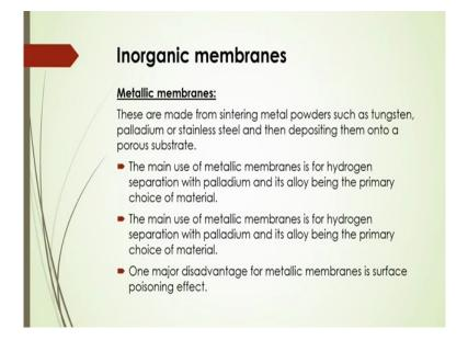
And in organic membranes like metallic membranes, in this case this type of membranes are being made from sintering metals such as tungsten, Palladium or stainless steel and then depositing them into a porous substrate and the main use of metallic membranes is for hydrogen separation with palladium and its alloy which is being the primary choice of material there.
