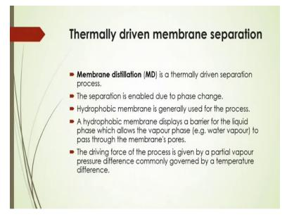
Another driving force based membrane it is called thermally driven membrane separation. And in that case membrane distillation is one of the important membrane processes where it is actually operated based on the thermally driven separation process. And the separation is enabled due to the phase change. In that case we will see that hydrophobic membrane is generally used for the process.
