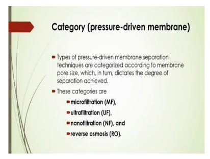
Now if we consider that the pressure driven membrane that is where that membrane separation techniques are categorized according to membrane pore size. In that case you will see it will dictates the degree of separation based on the size of the pore of this membrane. So in that case those membranes based on their pore size it will be classified as microfiltration, ultra filtration, nano filtration and also reverse osmosis.
