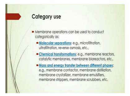
And what are the different that uses categorically by having that process intensification by this membrane. So in that case this Membrane operations can be used to conduct the operations or chemical processes categorically as like for the molecular separations even in the case of chemical transformation in the case of mass and energy transfer between different phases.
