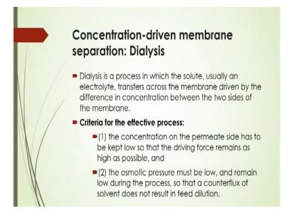
And another very important and mostly used membrane separation is called concentration driven membrane separation which is called Dialysis and Dialysis is a process in which that solute usually an electrolyte transfers across the membrane that is given by difference in concentration between the two sides of the membrane. And in this case what should be the criteria for the effective process.
