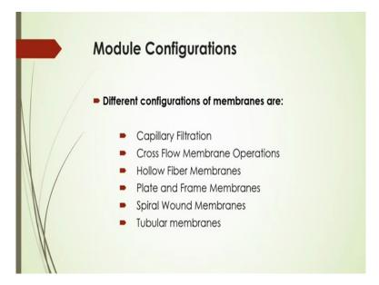
And of course different types of membranes will be applied for specific applications and of course based on the pore size ultrafiltration, Nano filtration, even microfiltration whatever it is and of course this type of membranes that is being procured based on that what the mechanism of that separation whether it is the pressured driven whether it is thermally driven or electrically driven or not that things.
