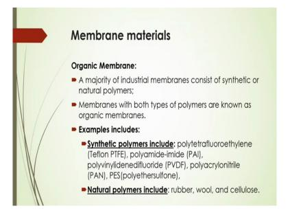
So as per that organic membrane, a majority of industrial membranes that consist of synthetic or natural polymers there. And in that case membranes with both types of polymers are known as organic membranes whether it is synthetic or natural polymers for example like synthetic polymers that will include that Polytetrafluoroethylene that is Teflon PTFE type material which is being used for membrane procurement. Polyamide membrane also it is called PAI membrane.
