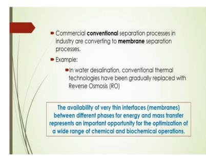
And you will see that, commercial conventional separation processes in industry generally converting to membrane separation processes because of course it has several advantages that we have discussed that it is energy-efficient process and also it may give that sometimes around 100 percent efficiency for the separation process. We will see that as an example we can say that in water desalination.
