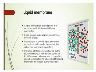
Other category out of that metal or chemical, ceramic or organic, chemicals or metal-based membrane, nowadays for specific application of solvent extraction or you can say that separation of the organic molecules in a solution without using that solid material the membranes are being procured which is called that liquid membrane. In this case a liquid phase that separates 2 liquid phases of different compositions.
