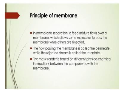
And you know that, whenever you are going to use this membrane process of course that, you have to know some principles of that membrane. So in membrane separation, a feed mixture flows over a membrane which actually allows some molecules to pass the membrane while others are rejected and then flow passing the membrane is called the permeate while the rejected stream is called the retentate.
