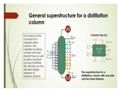
And here in this slides says general superstructure for the distillation column is shown. You will see that this superstructure is basically based on the concept of a you know, variable reflux column, the variable locations of the feed and side stream trays as well as reflux and boil-up trays that facilitates the decision on the discrete design and also design degrees of freedom. You see in this figure here there are maybe several feed streams will be there and
