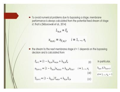
And to avoid the numerical problems due to the bypassing stage in that case membrane performance which allows the calculation from the potential feed stream of stage that is here given by Skiborowski et al. 2014, as per their you know suggestion that should be in let flow rate of this liquid should be is equal to you know,  $F_{st}$  that is at the stage what is the feed
