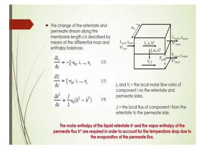
And in that case you have to you know, assist the change of retentate and permeate stream along the membrane lengths and that can be described by means of the differential mass and enthalpy balance here given, as in equation number 12, 13 and 14.
