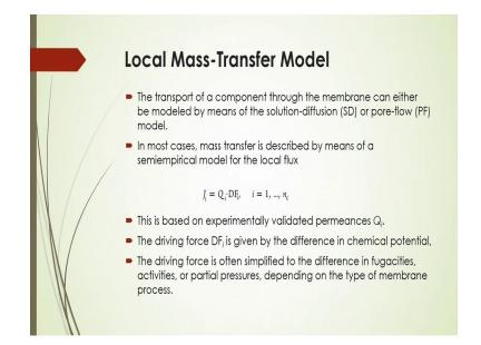
And also for assessment of this membrane performance you have to you know that, consider that local mass transfer model in that case the transport of that component through the membrane can either be modelled by means of that solution diffusion or pore flow model. In most cases mass transfer is described by means of a semiempirical model for the local flux as shown in equation here in the slides
