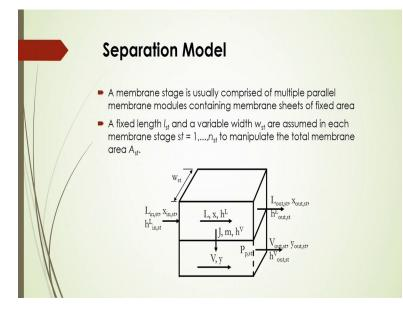
Now for that if you are considering that membrane that will be used for separations after distillation, so what should be modelled to be used for that membrane separation? So a membrane stage which is usually comprised of multiple you know, parallel membranes modules that contains membrane sheets of fixed area, a fixed length lst and a variable with wst are shown figure in the slides are assumed in each membrane stages to you know, manipulate the total membrane area are that is denoted by AST.
