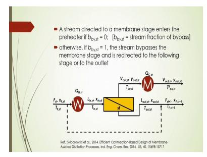
And a stream that is directed to the membrane stage that is enters the preheater in this case, if this bypass you know that fraction, bypass stream fraction if it is 0 then the stream directed to the membrane stage that is enters to the preheater. If suppose bypass stream fraction is equal to 1, so in that case the stream bypass, the membrane stage is redirected the following stage or to the outlets\ here in this figure as shown in the slide.
