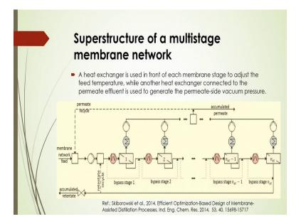
Superstructure of a multistage membrane network is shown here in a slide, in this case you will see that a heat exchanger is used in front of each membrane stage to adjust the feed temperature, while another heat exchanger connected to the membrane, the permeate side in that case it is used to generate the permit side vacuum pressure.
