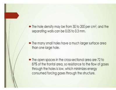
The whole density may be from 30 to 200 per centimetre square and the separating walls can be you know that sometimes 0.05 to 0.3 millimetre there. Many small holes have a much larger surface area then large hole, so in that case more reaction performance will be there because that surface area matters there, so more interfacial area will get between the phases and then you can get the better performance of the reaction in that direction the intensification of the process will be there.
