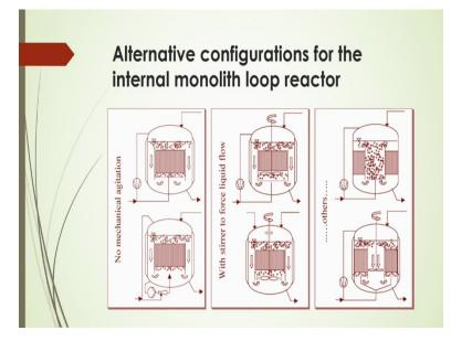
And also, you are getting alternative configurations for the internal monolithic loop reactors like sometimes where you will see that sometimes that mechanical agitation may not be required for that particular process, so through the monolithic structure there will be a flow of fluid, it may be laminar way that laminar flow condition and it may be the flat flow phenomena will be there through which that reactions will be actually occurred.
