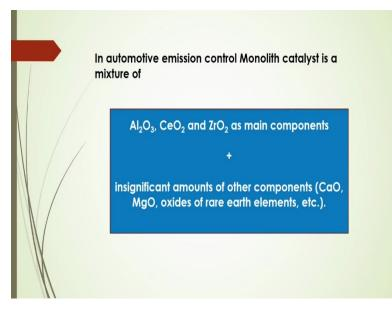
And mostly use this type of catalytic reactors or catalytic converter in automobile where the control of emission in the monolithic catalytic converter. In that case that monolithic catalyst will be mixture of aluminium oxide, cerium oxide and zirconium oxide as a main components, and also insignificant amounts of other components like calcium oxide,
