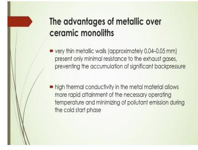
Whereas, the advantages of metallic over ceramic monoliths also will be there because there are two types of monolithic reactors are being developed; one is ceramic monoliths and another is the metallic monoliths. So in case of metallic walls, in that case very thin metallic walls approximately you can say that 0.04 to 0.05 millimetre presents only minimum resistance to the exhaust gases that prevent the accumulation of significant back pressure there.
