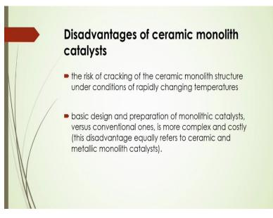
Also the risk of cracking of the ceramic monolith structure under conditions of rapidly changing temperature are there. Basic design and preparation of the monolithic catalyst versus conventional ones is also more complex and also it should be cost-effective, so that is why the disadvantage equally refers to ceramic and metallic monolithic catalyst are there, so these are some disadvantages you can say.
