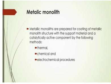
And metallic monolith are prepared for coating of metallic monolith structures with support material and catalytically active components by the following methods like thermal, chemical and electrochemical procedures are there.
