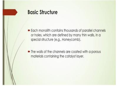
And each monolith actually contains thousands of parallel channels or holes which are defined by many thin walls in a special structure example, honeycomb there. And the walls of the channels are coated with a porous material that contains the catalytic or catalyst layer there.
