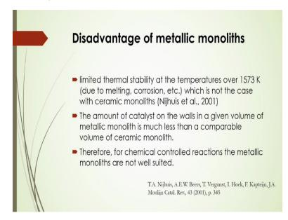
Some disadvantages also will have this metallic monoliths. In this case, limited thermal stability at the temperatures over 1573 K due to melting, corrosion, et cetera even which may not the case which ceramic monolith there. And amount of catalyst on the walls in the
