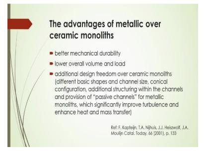
Also you will see that the metallic monoliths also have better mechanical durability, lower overall volume and load, additional design freedom over ceramic monoliths will be there. There may be additional structuring of channels and provision of passive channels for metallic monoliths will be there so that may significantly improve the turbulence and enhance heat and mass transfer in the case of metallic over ceramic monoliths there.
