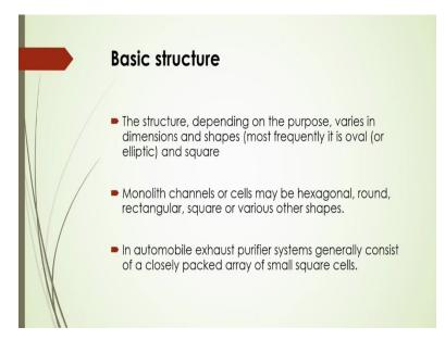
And what are the basic structure for that? The structure that depends on the purpose varies in the dimensions and shapes, most frequently it is oval or elliptical and also square you can say. And monolith channels or cells may be you know that hexagonal, round, rectangular, square or various other shapes there. In automobile exhaust purifier systems generally consists of a closely packed array of small square cells there.
