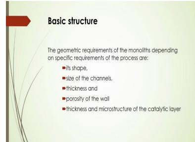
And the geometric requirements of the monoliths that depends on some specific requirements of the process like it is shape, size of the channel, even what should be the thickness and also what should be the porosity of the wall that is also important and whether you are going to make it a micro structure layer or not, so the thickness of the microstructure in a catalytic is also important there.
