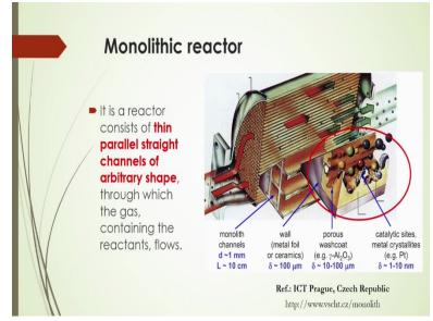
Now, what is that monolithic reactors, you will see the typical reactors are there as per ICT Prague Czech Republic, they are actually procuring these types of reactors, this is called honeycomb-based channel based monolithic reactor. And in this case the reactor as shown in figure here, you will see that this reactor consists of thin parallel straight channels of arbitrary shape through which the gas containing the reactance that will flows through that channel gap.
