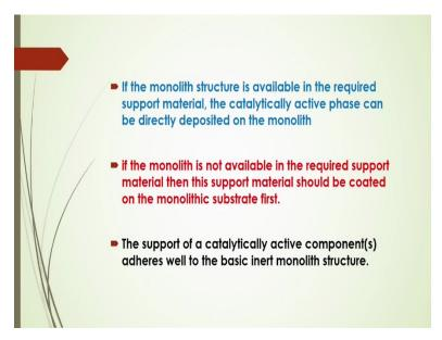
If the monolithic structure is available in the required support material, the catalytically active phase can be directly deposited on the monolith. And if the monolith is not available in the required support material then of course this support material should be coated on the monolithic substrate first. And support of a catalytically active components adheres well to the basic inert monolithic structure there.
