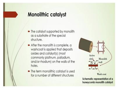
Now, the catalyst that is supported by monolith as a substrate of the special structure there. And after the monolith is complete, wash coat is to be applied there as per the picture shown here that deposit oxide and catalyst, and in that case mostly you know that platinum, palladium or rhodium on the walls of the holes there.
