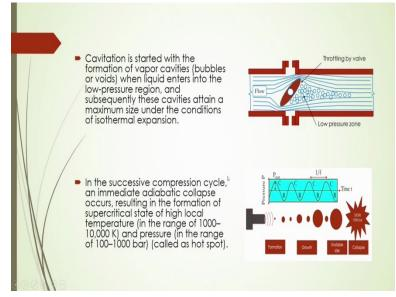
After then we can say that that cavity or cavitation process is started with formation of vapour cavities is that is called bubbles or voids or cavities sometimes it will be named, when liquid enters into the low-pressure region and subsequently these cavities attain a maximum size under that condition of isothermal condition or isothermal expansion.
