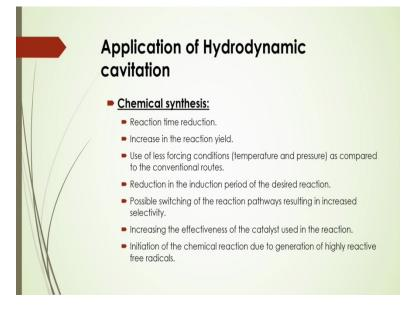
And what are the different applications of hydrodynamic cavitation? In that case you can increase that reaction time, for the chemical synthesis to reduce that reaction time instead of increase that reaction time so that cavitation process will be helpful for the reduction of reaction time because it is very faster to create that formation of hydroxyl radicals and the first reactions will be there.
