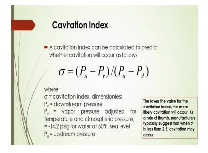
Now, you will see one parameter, it is called the cavitation index. This cavitation index can be calculated to predict whether the cavitation will occur or not. So that cavitation index can be defined as or it is denoted by Sigma and which will be calculated based on that pressure here in this equation given,
