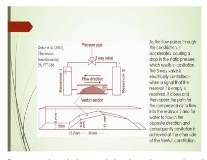
And here as the flow passes through the constriction, it accelerates and causing a drop in the static pressure which results in cavitation and the three-way valve is electrically controlled when a signal that the reservoir 1 is empty is received and it closes and then opens the path for the compressed air to flow into the reservoir 2. And for water to flow in the opposite direction and consequently cavitation is achieved at the other side of the venturi constriction.
