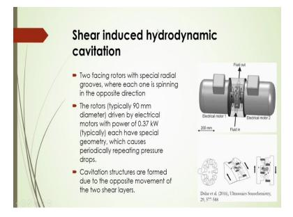
Another important is called shear induced hydrodynamic cavitation, in this case two facing rotators will be used to create this cavity. In that case special radial grooves are generally procured in these rotors where each one will be speeding in the opposite direction and in that case the rotors typically size will be 90 millimetre diameter it will be driven by electrical motors with power of around 0.37 kilowatt typically as per Dural et al. 2016.
