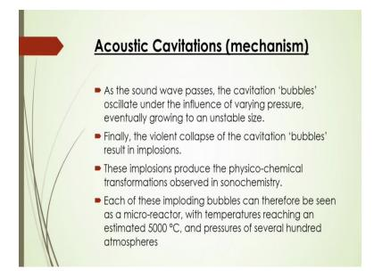
Now in the case of acoustic cavitation, as the sound wave passes, the cavitation bubbles oscillates under the influence of varying pressure, eventually growing to an unstable size. Finally, we can say that the violent collapse of the cavitation bubbles result in implosions, and also these implosions produce the physicochemical transformation that will observe in sonochemistry. And each of these you know imploding bubbles can therefore, be observed as
