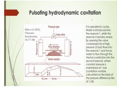
Now, pulsating hydrodynamic cavitation is also another one type of cavitation, so it is generally operated in cycles. Water is actually introduced into the reservoir, here as shown in figure, we have reservoir 1 and while the reservoir 2 remains here empty during that cycle. By opening the valve here you will see that the compressed air at high-pressure that is at
