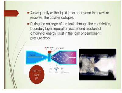
In this case as the liquid jet expands and the pressure recovers, in that case the cavities will collapse. And during the passage of the liquid through the constriction, boundary layer separation will occur and substantial amount of energy will be lost in the form of it is called permanent pressure drop, so that is why there will be a multi-number, or it is called that
