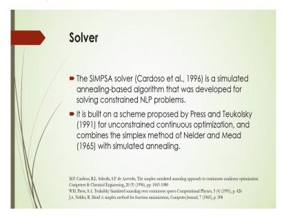
What are the solver that you can use that for the optimisation of that particular problem of this reactive distillation column? In this case this SIMPSA solver, that suggested by Cardoso et al in 1996 can be used and it is a solver simulated annealing based algorithm that was
