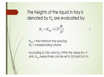
And here the heights of the liquid entry K, that will be denoted by  $\frac{H_{K}}{H_{K}}$ , that are calculated by
