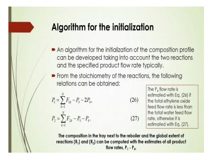
Now, algorithm for the initialisation, in that case the algorithm for the initialisation of the composition profile can be developed taking into account the two reactions and the specified product flow rates typically from the stoichiometry of the reactions, the following reactions can be obtained, that is in equation number 26 and 27.
