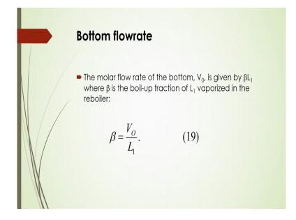
And if you are considering the bottom flow rate, the molar flow rate of the bottom denoted by  $V_0$  can be calculated by this beta into L, where beta is called boiler fraction of liquid stream  $L_1$ , that is vaporised in the reboiler, so beta should be equal to
