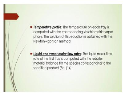
And the temperature on each tray can be computed with the corresponding stock metric vapour phase. The solution of this equation can be obtained with the Newton Raphson method. And also liquid and vapour molar flow rates also of the tray can be calculated with the reboiler material balance for the species that will correspond to the specified product.
