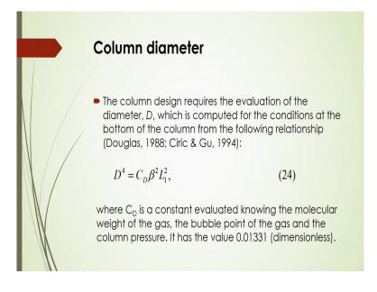
And then how to calculate that column diameter? The column design that will be required for the evaluation of the diameter D, which is computed or calculated for the conditions at the bottom of the column from the following equation, denoted by equation number 24,
