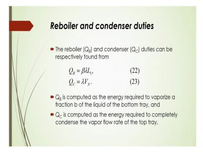
And this reboiler and condenser duties, how to calculate that, it can be calculated from this equation number 22 and 23.
