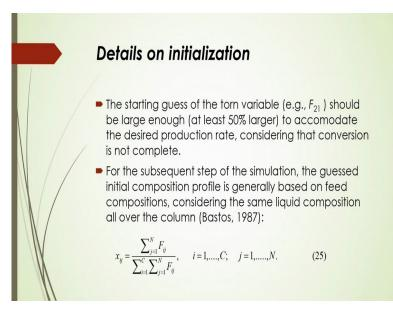
And in this case initiation is a very important one, that how to initiate that case of the torn, in that case it cannot be large enough but at least 50 percent larger to accommodate the desired
