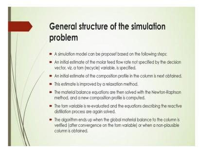
Now, general structure of the simulation problem, a simulation model can be proposed based on the following steps. Like this that an initial estimate of the molar feed flow rate, not specified by the decision vector, like a torn recycle or variable specified there. An initial estimate of the composition profile in the column to be next to be obtained and then this estimate can be improved by a relaxation method.
