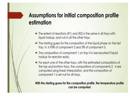
And assumptions for initial composition of profile estimation here in this case the extent of reactions that is R1 and R2 that has been given in earlier slides, that is should be is the same in all trays with liquid hold-up and null in all the other trays in that case. And the starting guess for the composition of the liquid phase on the last tray end is to be 95 percent of the component 2 and 5 percent of the component 3.
