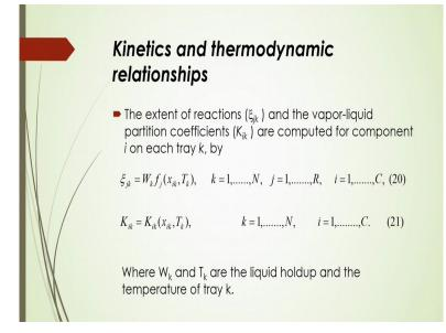
Now, after that you have to consider the kinetic and thermodynamic relationships. The extent of reactions  $\xi_{ik}$  and the vapour liquid partition coefficients or that is  $K_{ik}$  should be considered
