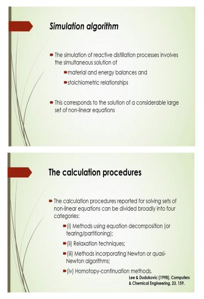
And in this case for simulation purpose you have to use that simulation of reactive distillation process which will involve simultaneous solution of material and energy balances and stoichiometric relationships. This corresponds to the solution of a considerable large set of nonlinear equations.
