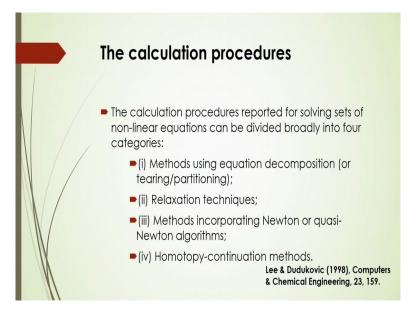
And for the calculation procedure that you have to know that consider this category is given in the slides like methods using equation for decomposition or tearing or partitioning relaxation techniques, methods in calculating Newton or quasi Newton algorithm homotropic continuation methods like this.
