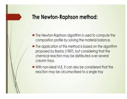
Now, so what is this actually Newton Raphson method? The Newton Raphson method is used to compute that composition profile by solving the material balance. The application of this method is based on the algorithm proposed by Bastos in 1987 but considering that the chemical reaction may be distributed over the several column trays. And with non-ideal
