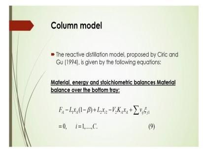
And column model, how actually that column model is developed as per that Ciric and Gu. They have given the following equations from the material, energy and stoichiometric balances, that the material balance over the bottom tray, they have given this
