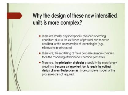
Now, why the design of this new intensified units is more complex whenever we are talking about that chemical engineering process intensification, of course, any process intensification we are talking that maybe that unit operations to be designed in such a way that will be more complex in some extent. So, why the design of those new intensified units should be more complex? In that case there are smaller physical spaces sometimes required in your process intensification.
