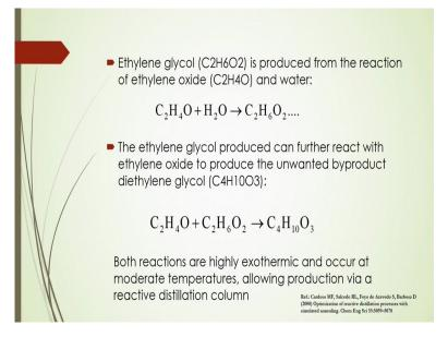
Now, what are the reactions actually being taken place here, in this particular reactive distillation column. So, in this case ethylene glycol is produced from the reaction of ethylene oxide and water there. So,
