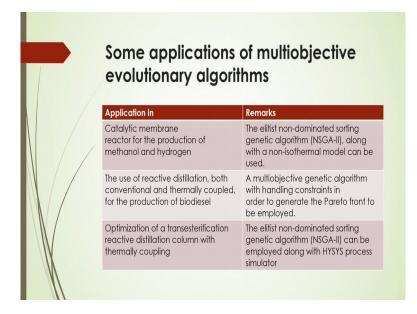
Some applications of multi-objective evolutionary algorithms are given here. You will see of course any process identified phenomena has different objectives whenever it will be executed any particular process synthesis there. So, in that case you have to solve those multi-objective operating conditions by those evolutionary algorithm. So, what are those special applications where you can apply the evolutionary algorithms based on that multi-objective function?
