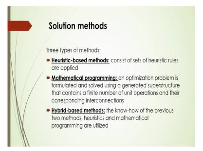
Now, what are the different solution methods to get that optimised, you know that process design. There are generally 3 types of methods, one is called heuristic based methods, it generally consists of sets of heuristic rules and also mathematical programming are one of the important you know that solution methods among the 3 methods of this given in the slides.
