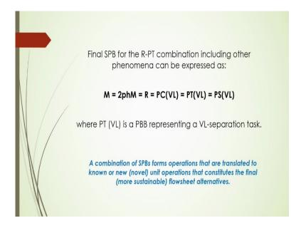
Final, that SPB for the RPT, that is you know the reaction and phase transition combination, that including other phenomena also can be expressed as this, by mathematics like, you know that M will be equal to 2phM, that is 2 phase mixing, that is equal to reaction that PC (VL) and PT(VL) and PS(VL), VL means vapour liquid, PC means phase contact between these vapour and liquid.
