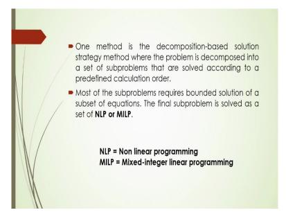
And also, one method is the decomposition-based solution strategy for this, you know where the problem is decomposed into a set of some problems that are solved according to the predefined calculation order. Most of the sub problems require a bounded solution of a subset of equations. The final sub problem is solved as a set of NLP or MILP. What is NLP? NLP is called Nonlinear Programming, whereas M ILP is called Mixed Integer Linear Programming.
