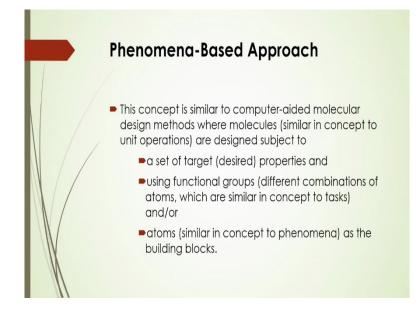
And based on that concept it is actually similar to the computer aided molecular design methods where molecules, that is similar in concept to unit operations are designed. That is subject to a set of you know target properties and using functional groups that is different combinations of the items which are similar in concept to task or you can say that atoms, that is similar in concept to phenomena as the building blocks.
