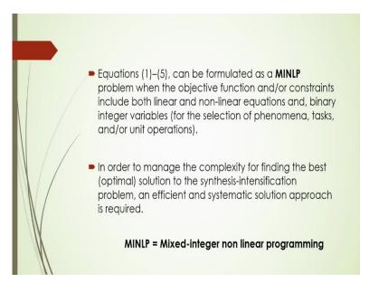
Now, equation 1 to 5, that I do not that in the beginning, that what are the equations can be formulated as a, you know that MINLP problem, when the objective function and/or constraints include both linear and nonlinear equations. And binary integers are variables for the selection of phenomena, tasks and unit operations.
