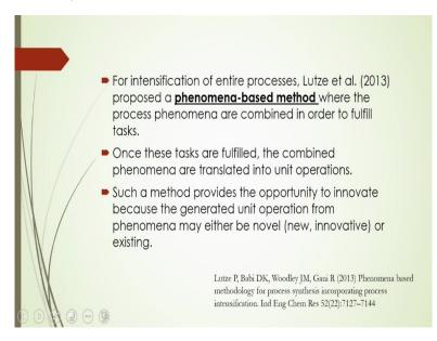
And for intensification of entire process Lutze et al. In 2013, they have proposed a phenomena-based method, where the process phenomena are combined in order to fulfil tasks. Like once these tasks are fulfilled, the combined phenomena are translated into unit operations. Such a method that will provide the opportunity to innovate because the generated
