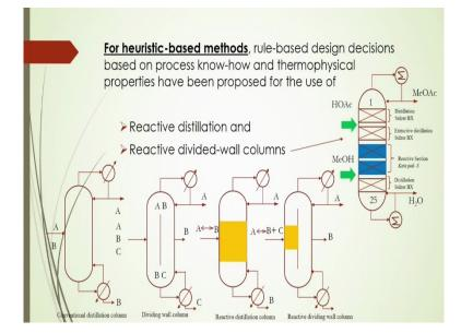
So, for heuristic based methods, it is generally rule-based, you know or design, decision based on process know-how and Thermo physical properties that have been proposed for the use of reactive distillation and reactive divided wall columns as shown in the figure in the
