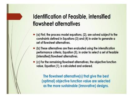
Now, what are the, you know that alternatives for the feasible, intensified flow sheet. 1st of all you have to consider the process model equations and which will be actually solved subject to the constraints that is defined in equation number 3 and 4 that earlier I have given in order to generate a set of flow sheet alternatives. These alternatives are then evaluated using the intensification performance criteria.
