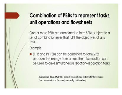
So, one or more PBBs are combined to form that SPBS, it is called Simultaneous phenomena-based building blocks, subject to asset of combination rules, that fulfil the objectives of any tasks there. Example, suppose if you are considering that reaction and also the phase transition, so this reaction and phase transition phenomena-based building blocks can be combined to form this simultaneous phenomena-based building blocks.
