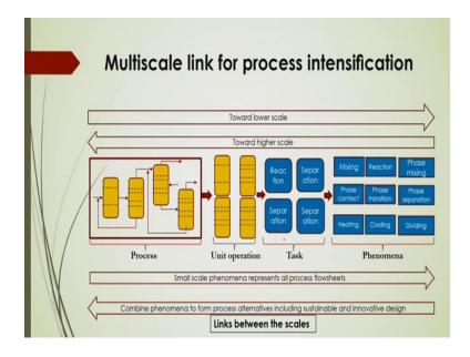
Now, let us have this links between the scales by this process diagram here, you will see if we divide it a certain process into different scales like processes scales, unit operations scale, task scales and phenomena scales. So, in this case, you will see that in the process scales, there may be you know, that reactions, there may be you know, that some other chemical synthesis process and the reactor.
