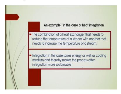
As an example, if we consider the case of heat integration. So, in that case, we have to consider the combination of heat exchanger as an example, that needs to reduce the temperature of the stream with another that needs to increase the temperature of the stream that means, from the one unit whatever fluid steam is coming, if its temperature is higher and that temperature, if you are going to utilize for the second operation, second stream like sub unit one and unit two.
