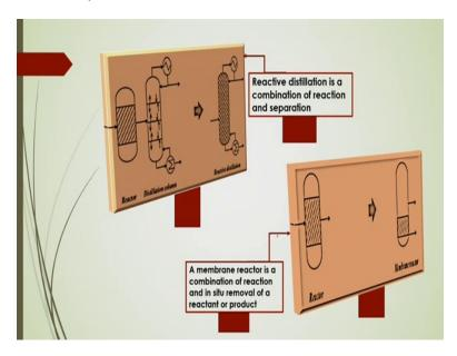
Now, reactive distillation is a combination of the reaction and separation in that case, what are the efficiency of that you know integrating system of reactive distillation based on you know that reactor size, distillation column size and different operating parameters. And if you are conjugating this unit operation, you will get the one single unit and that single unit will give you the better way of that process designed to get the better yield.
