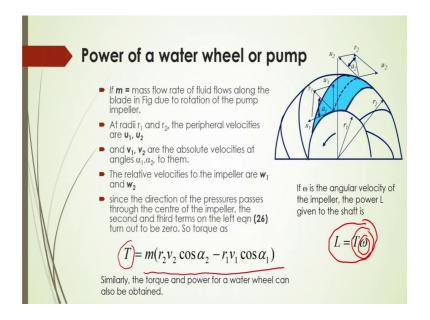
And what should be the power? There will be if there is a wheel or pump there that also you can apply the momentum equation here. And based on the if you are considering here that what should be the torque whenever fluid is actually discharging by the pump, then how what amount of actually torque is applied by this wheel of the pump then you can calculate from this equation.
