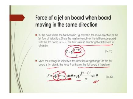
Now, the case where the board now is not in the rest in condition, it will be moving in the same direction at some other velocity. Now, in the case where the flat board it is shown in the figure here, in the same direction if it is the flat board is a flowing in the same direction at new velocity. Then what should be the effective mass that acts on the surface of the board? So, that you have to calculate.
