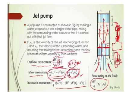
Another example of momentum equation like jet pump. See here, this is one jet pump, in this case one jet will be produced by changing the cross section of the pipe at this location here, just the liquid will be passing through this smaller cross sections and then it will be moving over this through this pipe.
