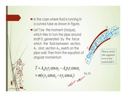
So, and also these are the some application of this angular momentum. And here from this equations also whenever fluid is flowing through this can do it at a certain angle at a with a certain angular momentum, then what should be the force acting over there you can easily calculate from this.
