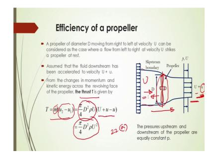
Now, another example of momentum equation that is called if to how to calculate the efficiency of a propeller. Now, this is one propeller like Aeroplan here. So, one it is propeller and this by this movement of this propeller the liquid will be moving from this section to this section.
