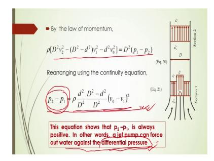
Now, balancing these two equations we can get by law of momentum simply by balancing this two. So, we can have after rearrangement p 2 minus p 1 will be is equal to what. So, from this jet what will be the pressure creating by the jet pump that will be is equal to p 2 minus p 1. So, this will be your as per equation number 21.
