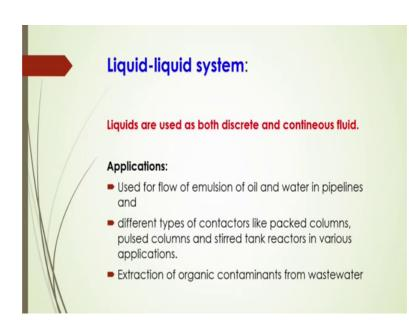
Now, let us have an example of liquid-liquid systems. Suppose liquids are used as a both discrete and continuous liquid here. Suppose one example, I am giving suppose; if you want to extract or remove what is that acetic acid or propionic acid from the waste water or some water where this acetic acid or reached there. So, you have to extract those acetic acid what to do.
