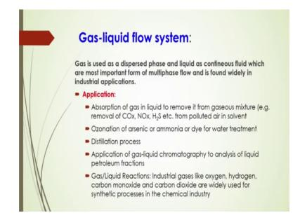
Now, some applications like here you know that absorption of gas in liquid to remove it from gases mixture and removal of carbon dioxide, removal of nitrogen dioxide even hydrogen sulfide from the polluted air in solvent that is one important operations for the absorption. So, this is one type of gas liquid flow operations that is multiphase flow operation.
