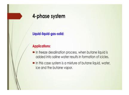
Suppose in freeze desalination process what will happen? The when butane liquid is added into the saline water that will results the icicles; so, in that is this type of operation is called what is that liquid liquid gas solid. In this case system is a mixture of butane liquid, water, ice and the butane vapor. So, this four phases will be there in the what is that systems. So, that is why this is called that four phase system.
