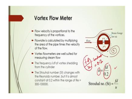
Now, in this case how that this flow velocity will be related to that frequency of the vortices that is given as per Karman equation. Now, this flow velocity since it is proportional to the frequency of the vortices we can say that, this f will be is equal to sum that is what is that f as a function of what is that velocity will be there? So, in that case not only that velocity it may sometime should be happen that what should be the area of the pipe.
