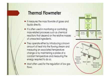
Now, another important flow meter it is called thermal flow meter this is one of the widely used flow meter and it measures the mass flow rate of the gases and liquids directly here. And in this case you will see the as per figure shown here, there is a pipe how this there are different part of this devices are given here and it is often used in monitoring or controlling mass related process such as chemical reactions that depend on the relative masses of unreacted ingredients.
