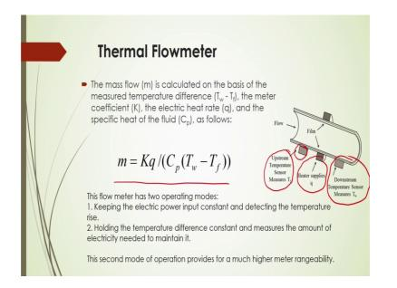
Now, the mass flow can be calculated on the basis of this measured temperature differences of these T w and T f here it is shown here this; this probe will give you the up stream temperature sensor as T f and this would be downstream temperature sensor which will give you the temperature of the downstream fluid.
