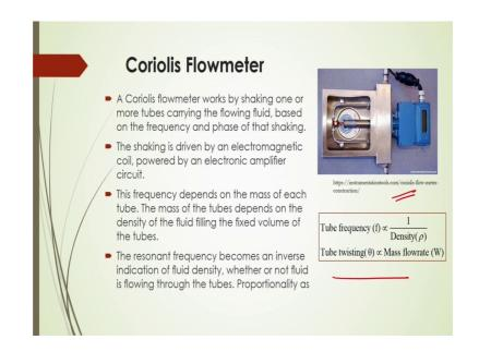
Another one important that Coriolis flow meter, it generally works of based on the shaking of one or more tubes and in this case whenever tubes will be a shaking based on the fluid energy that is supplied at a particular velocity of the fluid it will be give you
