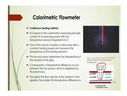
So, let us consider here the basic principles of the calorimetric flow meter, this is one of the important a flow measuring device it is generally being used in what is that based on the calorimetric measuring principles. And, in this case it consist of a measuring probe with two temperature sensors and we shall be integrated into this device.
