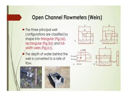
Another already we have discussed that channel flow meters that is weirs and there are three principles weir are generally at configured to measure the flow rate in open channel, those are actually triangular, rectangular and also full width weirs as shown in figure a b c respectively and the depth of the water behind the weir is converted to a rate of the flow.
