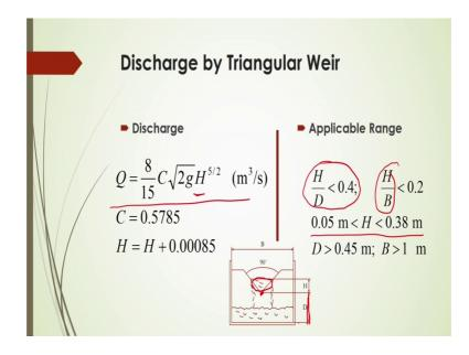
Now, what would be that flow rate or it is called discharge from the open channel for the triangular weir, this discharge will be calculated based on this what is that open height of the channel here it is depth of the water behind the weir. And this weir already we have discussed in the earlier lecture, so what is that weir design of the weir all this things.
