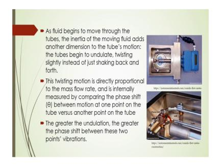
And, in that case the inertia of the moving fluids that adds the dimension that is to vibrate or shake to the tubes motion in the other direction and that case the tubes begin to undulate, twisting slightly instead of just shaking back and forth. And this twisting motion is directly proportional to the mass flow rate and is internally measured by the
