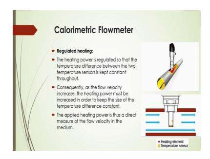
Now, so this is the basic principle for that, so the heating power is regulated so that the temperature difference between the two temperature sensors should be kept constant throughout the operation and in that case as the flow velocity increases, the heating power must be increased in order to keep the size of the temperature difference are constant.
