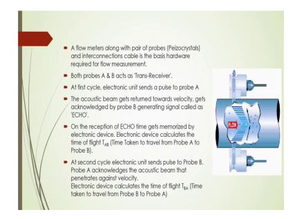
Now, a flow meters along the pair of this probes generally and interconnections cable is the basis hardware required for this flow measurement. Both probes A and B you can say acts as trans receiver and also at the first cycle you will see there will be some electrical condition and where the electronic unit sends a pulse to probe. And the acoustic beam that case gets returned towards the velocity gets acknowledged by the probe B and it will generate the signals we should be called as echo.
