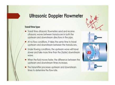
So, for those operations this type of flow meter will be used generally for Doppler type and also another important type is for this transit time type, here in this case this device will send and receive the ultrasonic waves between the transducer in both the upstream and downstream directions in the pipe. And, also you will see there will be no flow conditions there and it will takes the same time to travel upstream and downstream between the transducer there yet to transducer will be placed.
