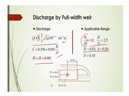
And in the case of full width weir you can calculate that or measure the discharge by this equation and again here the C is on constant that is called weir constant here and this weir constant you can get it based on the geometry that would be depends on that, that it will depends on H and D here that H will be calculated by this equation.
