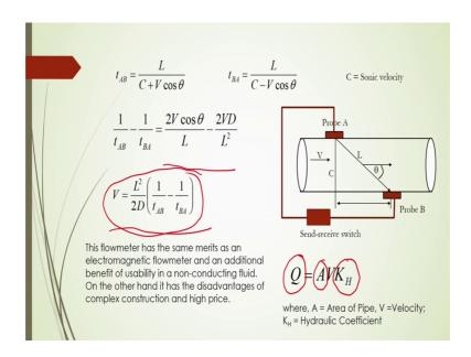
Once you know that time like that T AB which will be L by C plus V cos theta one equations by this formula you can calculate where C is called sonic velocity and V is the fluid velocity. And theta is the angle of this, what is that probe A and B where you are substituting or you are attaching and what would be the angle with that flow that is given theta as it is shown in the figure. And similarity T BA that will be L divided by V minus V cos theta.
