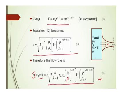
Now, using this isentropic flow condition of T is equal to m into rho to the power k minus 1 that will be is equal to m into p to the power k minus 1 by k; where m is constant in that case equation twelve becomes. So, after simplification it will be u will be equals to root over 2 k by k minus 1 into p 0 by rho 0 into one minus p by p 0 to the power k minus 1 by k.
