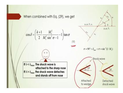
Similarly, if we combine with that equation number 29 we get that cos delta will be is equal to this as equation number 32 it is shown. So, based on which you can have an assessment for the shockwave whether if it will be sharp nose or it will be stands off from the nose or not.
