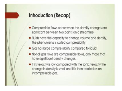
So, as we have already discussed the definition of a compressible flows which occurs when the density changes are significant between two points on a stream line. Fluids have the capacity to change volume and density the phenomena is called compressibility and also we have discussed that the gas has large compressibility compared to liquid as per definition.
