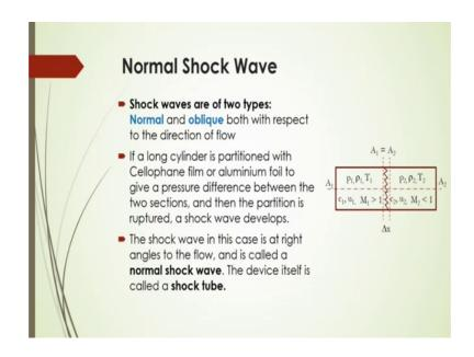
And then you will have these two types of shocks in this flow condition; one is called normal another is called oblique type of that is shockwave. And if you are having that long cylinder in a partitioned with the cellphone film or aluminuim foil to give a pressure difference between the two sections and then the partition will be called as a shockwave. In that case the shockwave will be at the right angles to the flow and it will be called as normal shockwave.
