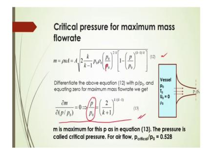
Now, what should be the critical pressure for the maximum mass flow rate? Here the mass flow rate is given in equation number 12. So, after differentiation of this equation twelve with p by p 0 p by p 0 in this case and equating 0 for maximum mass flow rate we get this here equation number 13.
