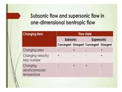
Now, here some characteristics feature for the subsonic flow and supersonic flow in one dimensional isentropic flow. If we change the item like this changing area changing velocity or MAC number and changing density pressure or temperature; then what should be the flow state?.
