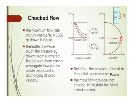
Now, if we consider that this maximum flow rate occurs when p by p 0 is equal to 0.528 as shown figure here. If we plot this p by p 0 with respect to the position in the nozzle of this convergence section here, then we can have at this value of p by p 0 is equal to 0.528; there will be a constant pressure; that means, the pressure which will be almost equals to the 52.8 percent of the total pressure of the vessel.
