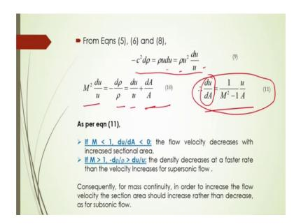
Now, from equation number 5, 6 and 8 after simplification you can write here, this minus c square into d rho that will be is equal to rho u d u is equal to rho u square into d u by u.
