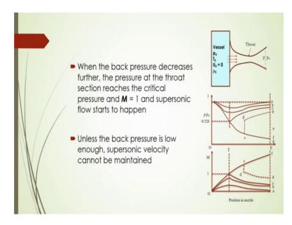
Now, when the back pressure decreases further; the pressure at the throat section reaches
