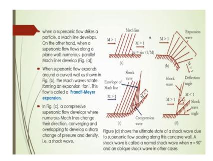
Now, another important that the how this Prandtl Meyer expansion can be formed based on this subsonic and supersonic criteria of this compressible flow. So, in that case if you have a supersonic flow that will strikes a particle a MAC number line develops on the wave.
