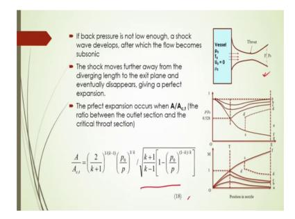
Also if back pressure is not low enough a shock wave develops in there and after which the flow becomes subsonic. And the shock waves further away from the diverging length to be exist and in that case the exit plane and eventuality disappears and giving a perfect expansion there as shown in figure here.
