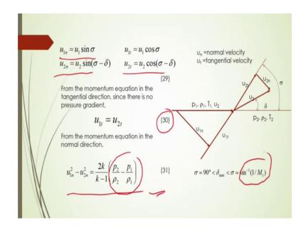
And also for this what should be the tangential flow and also the normal flow and how to calculate that type you know that the angle of this tangential and the normal velocity happened at this direction here are shown in figure. So, you can calculate what will be the velocity at this normal flow condition and at the tangential flow condition this shown in equation number 29.
