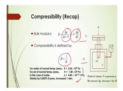
Now, we have already given the definition of the compressibility; it depends on bulk modulus which is defined as that is the delta p by del V by V; that means, here ratio of the change of pressure drop per unit volume change of a system. So, in that case this bulk modulus is defined as given in equation number 1 and then compressibility is defined by that is inverse of this bulk modulus, this will be here beta and it will be 1 by K and this is given in equation number 2.
