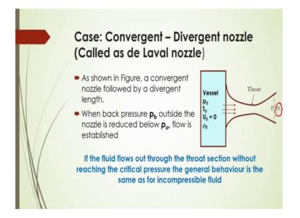
And in that case sometimes this condition is called that the de Laval nozzle. So, as shown in figure in the slide a convergent nozzle followed by a divergent length. So, this geometry it is called as de Laval nozzle geometry. And when that back pressure pb here outside the nozzle is reduced below p 0 flow will be established.
