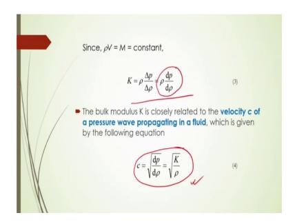
And also if you substitute this gas equation here rho b is equal to m then in that case K should be is equal to in terms of that is density change then it will be rho into d p by d rho that will be again that bulk modulus in terms of this density change how it will be happen.
