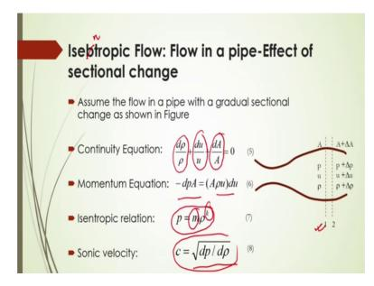
Let us consider here that isentropic flow here isentropic flow; so flow in a pipe that effect of sectional change. Now let us assume the flow in a pipe of a gradual sectional change as shown in here. In this case what should be the continuity equation? That continuity equation it is given as that d rho by rho plus du by u plus dA by A that should be is equal to 0 and momentum equation for this compressible flow it will be minus d p into A; that will be A into rho u into du.
