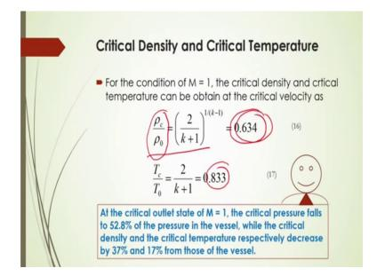
Now, again based on this critical velocity or this condition of this critical pressure at the condition of MAC number is equal to 1, you can calculate the; what should be the critical density there. So, the critical density and the critical temperature can be obtained at the critical velocity as by this equation rho c by rho 0 that will be is equal to 2 by k plus 1 to the power 1 by k minus 1 from which you can calculate what is should be the rho c.
