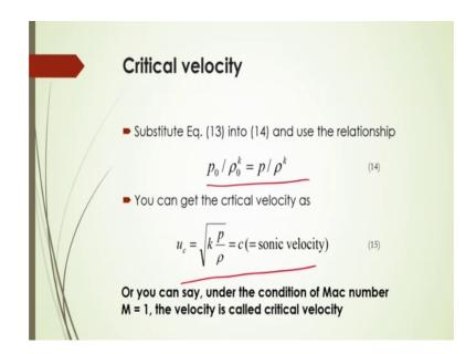
Whereas substituting this equation number 13 that here given here at this condition p by p 0 is equal to 2 by 2 k plus 1 to the power k by k minus 1 in equation number 14 and use the relationship of this p 0 by rho 0 to the power k is equal to p by rho to the power k; then you can get the critical velocity of uc as root over k into p by rho. So, that will be is equal sonic velocity.
