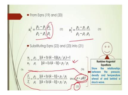
Now, from these equations 19 and 20 here it is given and based on these equations; you can calculate what should be the velocity at the sections 1. So, u 1 square will be is equal to that is after simplification it will become 2 minus p 1 by p 1 by rho 2 minus rho 1 into rho 2 by rho 1. And similarly u 2 will be again as per this equation number 23.
