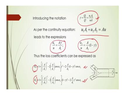
Now, if I introduce the notation as gamma as Q 1 by Q that will be is equal to u 1 A 1 by u A based on the mass conservation equation and we can write this u 1 A 1 plus u 2 A 2 that will be is equal to A into u and defining this gamma and substitute this equations then we are getting this u 1 by u that will be equals to A gamma by A 1 after simplification. Similarly for the ratio of u 2 by mainstream u that will be equals to A by u A 2 into 1 minus gamma.
