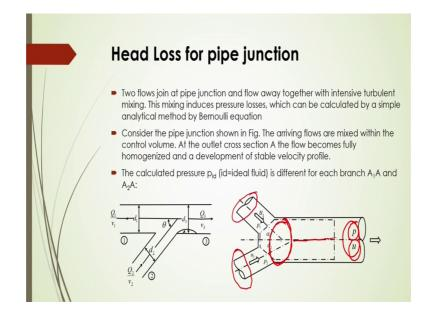
And if the two flows join at pipe junctions and flow away together with intensive turbulent mixing that is here two pipes are coming together and joining and forming one pipe cross section. So, in this case the mixing induces pressure losses which can be calculated by a simple analytical method by Bernoulli's equation here.
