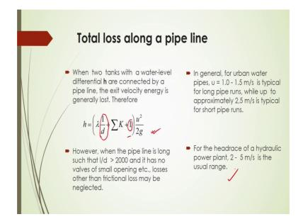
When two tanks with a water-level different height of h are connected by a pipeline, then the exit velocity energy of course, will be lost. So, therefore, in that case you have to consider that exit loss coefficient also in this case. So, it will be lambda into 1 by d plus summation of K plus 1 into u square by 2g.
