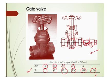
Now, if we consider the gate valve as shown here figure see this gate valve this is the main junction through which this flow will be getting struck or getting controlled here. So, in this to know such there here this is your cross sectional area through which this pipe of cross section area and this is the nose by which the flow will be controlled. Now, in this case what will be that diameter of the pipe and what will be the gap between these nose to this pipe valve this is denoted by d dashed.
