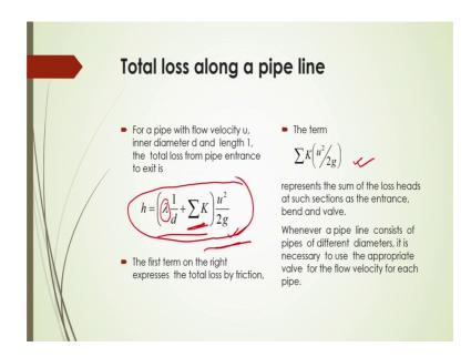
Now, what should be the total loss along a pipe line? If we are considering that a flow through a pipe with a velocity u of inner diameter d and the length l then total loss from the pipe entrance to exit entrance to exit that will be calculated by this in this case you
