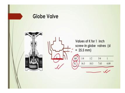
Similarly, the globe valve what should be the minor energy loss there if we know the loss coefficient as given here. Like this 16.3 for l by d, if it is 1 by 4 as shown in here figure. This d is this diameter of this valve and here in this case this l is like this gap. So, based on this as per represented here in this figure we can have for different ratio of l by d we can have this a minor loss coefficient here.
