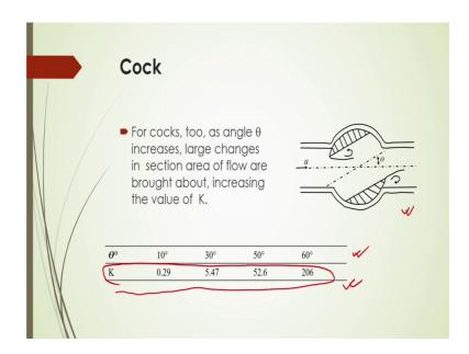
Now, similarly for cocks, in this case as shown in figure here, for cocks as angle theta again increases the then large changes in section area of the flow are brought about increasing the value of K. So, if we increase the theta here the respective value of K are shown in table here accordingly.
