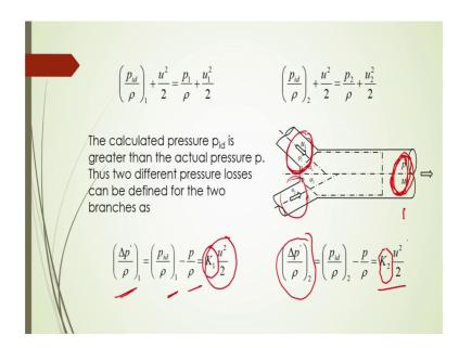
Now, if we consider the Bernoulli's equation here for this pipe then we can write here p id by rho; that means, here at the sections of p that is pipe then what should be the p pressure let it be pressure p id or p. So, you can say here p id by rho at this directions 1 plus here in this angle here p i d here this p id this pipe initial pipe p id by 1 plus u square by 2 that will be is equal to p 1 by rho plus u 1 square by 2.
