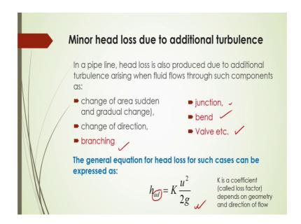
Now, we know that this minor head loss is generated due to the additional turbulence created by this fluid flow whenever it will be flowing through the bend or junction or through valve or by change of direction of the fluid or any sudden expansion or contraction of the pipe or not. So, we have already discussed the minor loss coefficient for the change of area sudden area change and also gradual change and also change of direction in the previous lecture.
