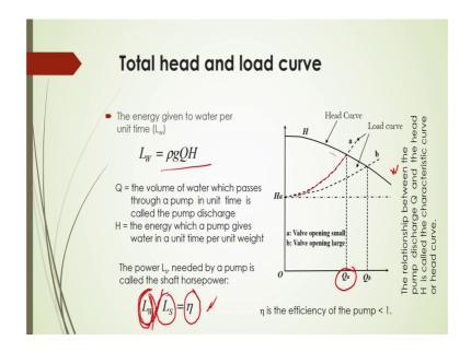
And again what should be the total head and load curve for this pump. Now, the energy given to the water per unit time L W that will be is equal to rho g into Q into H; where Q is the volume of water which passes through a pump in unit time that will be called as pump discharge and H that is denoted for the energy which a pump gives water in a unit time per unit weight. And the power denoted by L S needed by a pump to deliver this fluid that will be called the shaft horsepower.
