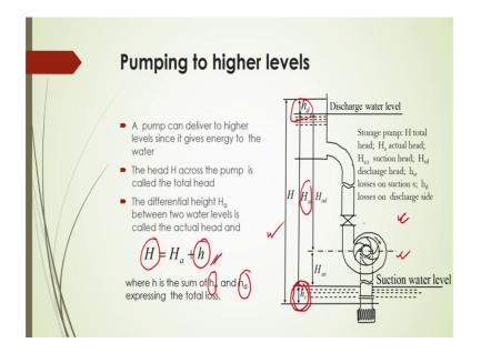
Now, if we consider a pumping a fluid to higher levels. So, in that case a pump can deliver the liquids to higher levels and it gives some energy to the water for which it will be flowing up to a certain location. The head H across the pump then it will be called as total head as shown in figure here. The differential height H a this height between two water levels is called the actual head here and H will be equals to total height will be equals to this H a plus h.
