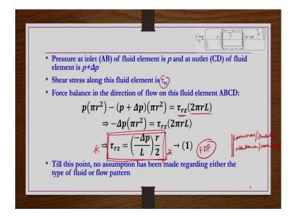
The same picture is shown here again the pressure at inlet AB is p and then pressure at outlet CD is the p +  $\Delta$ p. So, that you know we can do the balance subsequently the shear stress along this fluid element is only  $\tau_{rz}$  is existing that we have seen right.
