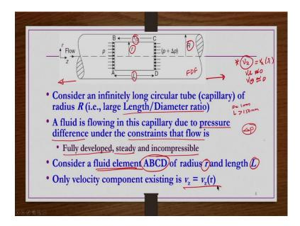
So, now, within this flow geometry consider a fluid element and then name it ABCD, the fluid element is having radius r and length L right pictorially if you see. So, it is an infinitely long cylinder.
