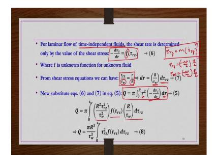
So, for laminar flow of time independent fluid. So, this is all we are doing for the time independent fluids analysis from this point onwards, the shear rate is determined by the value of the shear stress something like this  $\frac{-dv_z}{dr} = f(\tau_{rz})$ .
