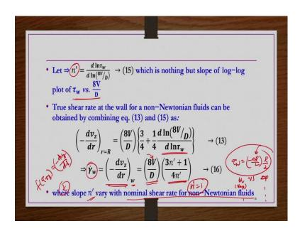
So, now further what we do whatever  $\frac{d \ln \tau_w}{d \ln \left(\frac{8V}{D}\right)}$  is say that we take it as n' which is nothing but the slope of  $\tau_w$  versus  $\frac{8V}{D}$  plot on a log log graph sheet, on a log-log graph sheet if you plot out w versus  $\frac{8V}{D}$  whatever is there.
