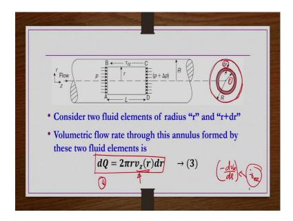
Consider two fluid elements of radius r and r + dr. So, the volumetric flow rate through this annulus formed by these two fluid elements would be  $dQ = 2\pi r v_z dr$ ,  $v_z$  is function of r.
