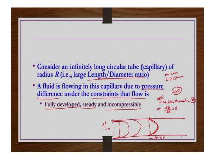
Now, what we do? We try to develop you know working principles for these capillary viscometers, developing working principles or equations for this capillary viscometer is nothing but you are going to develop a relation for shear stress in terms of measurable property something like pressure drop or volumetric flow rate or average velocity something like that.
