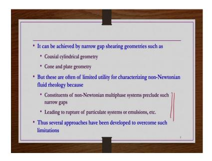
But the problem is that these are often of limited utility for characterizing non-Newtonian fluids because as mentioned constituents of non-Newtonian fluids non-Newtonian multiphase systems precludes such narrow gaps leading to rupture of particulate systems or emulsions etcetera.
