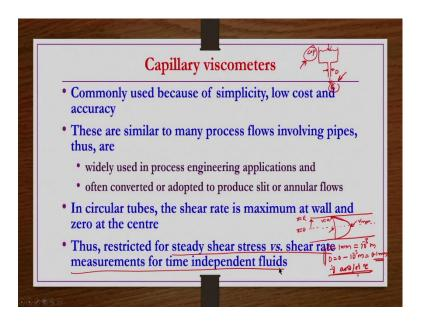
So, now we start with capillary viscometers ok. So, what is a capillary? Capillary is a straight tube of a very small diameter compared to the length of the tube right. So, that is large length by diameter ratio tubes whatever circular tubes are there those things we can regard as a capillaries.
