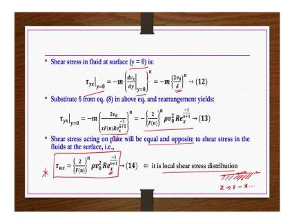
So, now shear stress in fluid at surface y = 0 if you wanted to find out. Why you wanted to find out? Because you wanted to find out the drag force and then finally, drag coefficient as well. So, for that you need to know what is the shear stress at the solid surface that is at y = 0 ok. So,  $\tau_{yx}$  at y = 0 is nothing but  $-m\left(\frac{dv_x}{dy}\right)^n$  at y = 0.
