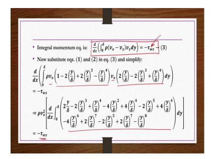
So, integral momentum equation is this one which is same for the fluid whether it is Newtonian or non-Newtonian it does not change ok because it has been developed a generalized one. It is not so, specific to any fluid ok the nature of the fluid will come into the picture through this  $\tau_{wx}$  information ok.
