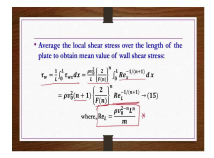
Now, if you wanted to find out the average shear stress over the length of the plate then what you have to do? You have to take the integral of a  $\tau_{wx}$  from 0 to L and then divide by L. So, that  $\tau_w$  that is the average shear stress along the length of the plate is integral  $\tau_{wx}$  dx divided by integral dx limits 0 to L.
