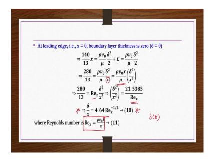
So, we have  $\frac{140}{13} = \frac{\rho v_0}{\mu} \frac{\delta^2}{2}$  that is what we are having, because C is 0. Now, this 2 I take to the left hand side. So,  $\frac{280}{13}$  and then this x I have taken to the right hand side. Next step I am multiplying and dividing by x in the right hand side. So, that I have  $\frac{\rho v_0 x}{\mu} \frac{\delta^2}{x^2}$ . So, this is nothing but Reynolds number local Reynolds number Re<sub>x</sub>.
