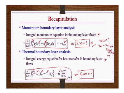
So, this integral momentum equation we have developed for the case of a fluid which is incompressible and flowing steadily. So, this equation whichever we developed that is integral momentum equation is valid for both Newtonian as well as non-Newtonian fluids.
