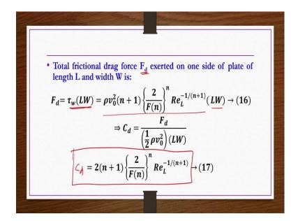
Now, total frictional drag force  $F_d$  exerted on one side of plate of length L and width W is nothing but  $\tau_w$  (LW) because width of the plate in the z direction is W and then frictional force if you wanted to find out that  $\tau_w$  should be multiplied by the surface area of the plate on which it is this frictional force is acting.
