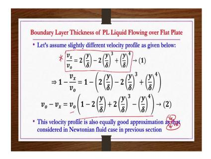
So, now we take boundary layer thickness of power law liquid flowing over flat plate. So, let us assume slightly different velocity profile. So, now, rather obtaining the velocity profile by taking 4th degree polynomial and then applying boundary condition and all that, we already assume the velocity profile is having this form and this is consistent with some of the experimental results. In fact, this results has been taken from one of the experimental research work ok.
