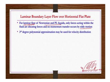
So, laminar boundary layer flow over horizontal flat plate we are considering that is the same scenario that we have consider in the previous lecture, where we developed integral momentum equation. Then for laminar flow of Newtonian and power law liquids, only force acting within the fluid are shearing forces and no momentum transfer occurs by eddy motion because we are assuming the laminar flow.
