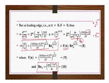
So, then finally, what we have? We have only this term right. Now next step what I am trying to do? I am taking this n + 1 of left hand side to the that whatever n + 1 term in the left hand side that I have taken to the right hand side and then both sides I have divided by  $x^{n+1}$  both sides.
