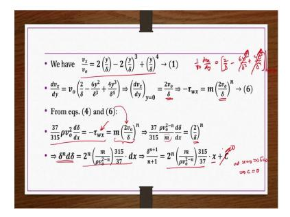
So, now what you have to do? You have to find out what is  $\frac{dv_x}{dy}$  from  $v_x$  expression and then substitute y = 0. So,  $v_x$  is this one. Now from here  $\frac{1}{v_0} \frac{dv_x}{dy} = \frac{2}{\delta} - \frac{6y^2}{\delta^3} + \frac{4y^3}{\delta^4}$ . And then now you substitute y = 0 in these two equations. So, you get this term is gone this term is gone because of y terms are there. So, you get  $\frac{2v_0}{\delta}$  as  $\frac{dv_x}{dy}$  at y = 0.
