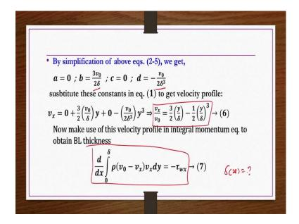
When you do that you get  $b = \frac{3v_0}{2\delta}$  and  $d = -\frac{v_0}{2\delta^3}$ . Now, these constants you substitute in equation number 1. So,  $v_x = 0 + \frac{3v_0}{2\delta}y + 0 - \frac{v_0}{2\delta^3}y^3$  that is  $\frac{v_x}{v_0} = \frac{3}{2}\frac{y}{\delta} - \frac{1}{2}\left(\frac{y}{\delta}\right)^3$ .
