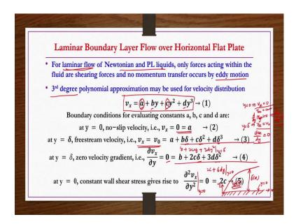
So, this region the thickness of boundary layer is nothing but  $\delta$  it is function of x right. So, this is all  $\delta$  which is varying with x. As x increasing  $\delta$  is increasing. So, this velocity profile can be best approximated by higher degree polynomial. So, then what we are assuming?
