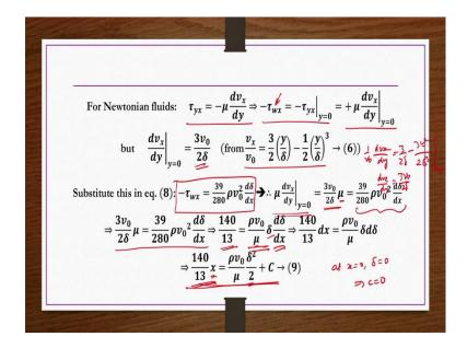
For a Newtonian fluid we take a simple case of. Now, what we do? Before going into the details of a complicated case of a momentum boundary layer thickness of a non-Newtonian fluids, we take simple Newtonian fluids as a starting problem. So, for Newtonian fluids  $\tau_{yx}$  is nothing but  $-\mu \frac{dv_x}{dv}$ .
