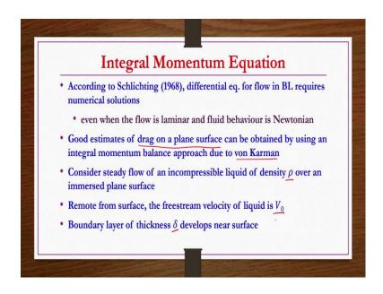
Now, we are going to develop integral momentum equation for this boundary layer flow, laminar boundary layer flow only right. According to Schlichting differential equation for flow in boundary layer requires numerical solutions even when the fluid is Newtonian and the flow is laminar.
