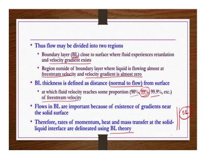
So, that is the flow may be divided into two regions; the boundary layer close to the surface where the fluid experiences retardation and velocity gradients exist and then region outside of boundary layer where the liquid is flowing almost at free stream velocity and velocity gradient is almost zero.
