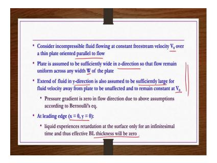
So, whatever we discussed here I have provided as a notes here right. So, considering incompressible fluid flowing at constant free stream velocity  $V_0$  over a thin flat plate oriented parallel to flow and then plate is assumed to be sufficiently wide in z direction. So, that flow remain uniform across any width W of the plate; in the z direction width of the plate is W.
