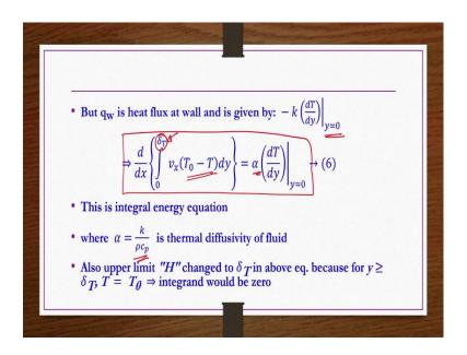
So, you get this x equation as integral energy equation integral form of the energy equation. Here also the upper limit of integration has been changed from H to  $\delta_T$ ; because we wanted to have this integral energy equation for the boundary layer region only within the boundary layer region only which is encapsulated between y = 0 to  $y = \delta_T$  and it is function of x.
