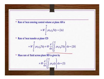
The pictorially I have explained whatever there, so, the same thing I have written here. Rate of heat entering control volume at plane AB is this one rate of heat transfer at plane CD is nothing but this one  $+\frac{d}{dx}$  of that whatever 2 b expression right. And then mass rate of fluid a cross plane BD that we have already seen that is nothing but  $W \frac{d}{dx} \left\{ \int_0^H \rho v_x dy \right\} dx$  that we have seen.
