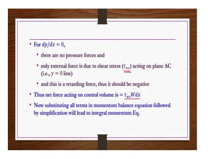
For  $\frac{dp}{dx} = 0$  there are no pressure forces and only external force is due to shear stress that acting on plane AC that is at y = 0 line that we are calling  $\tau_{wx}$ . So, and this is retarding force thus it should be negative. So, both at BD and then AC planes whatever the momentum is there that they are negative. So, thus net force acting on control volume would be  $\tau_{wx}$  W dx as described in the figure.
