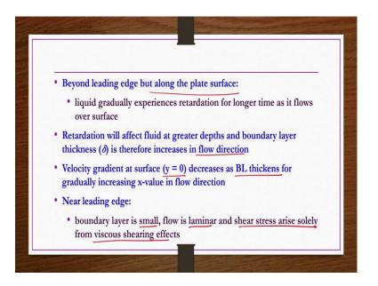
But beyond the leading edge, along the solid surface or plate surface liquid gradually experiences retardation for longer time as it flows over surface, thus boundary layer thickness increases in the flow direction. So, that is  $\delta$  is function of flow direction now here in this case it is x.
