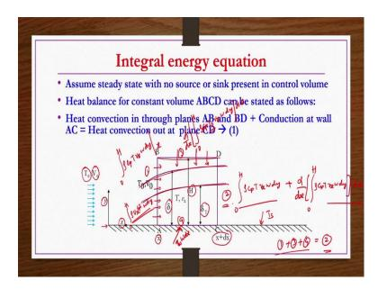
So, now we develop integral energy equation, here the same equilibrium of control volume we are taking. Now, here in addition to  $V_0$  free stream velocity the temperature of free stream fluid is  $T_0$  and the surface temperature is  $T_s$  right. So, flow direction is x direction vertical direction is y direction.
