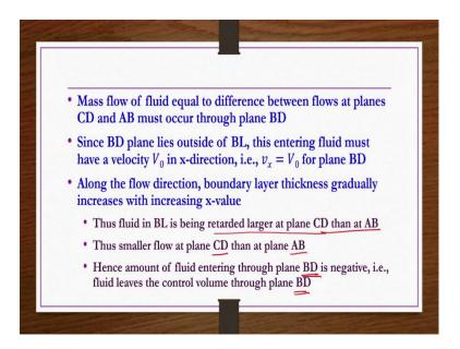
So, now mass flow of fluid equal to difference between flow at plane CD and AB must occur through plane BD. So, since BD plane lies outside BL this entering fluid must have a velocity  $V_0$  in x direction. Along the flow direction boundary layer thickness gradually increases with increasing x value. So, because of that one fluid in BL is being retarded larger at plane CD than plane AB.
