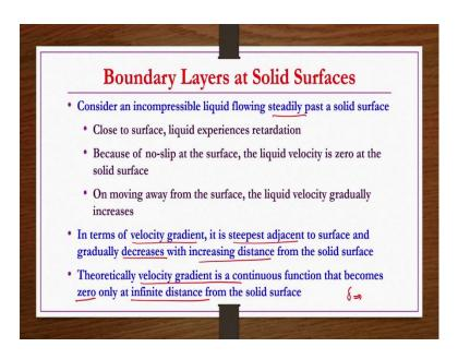
So, first we see a few basics of a boundary layers at solid surface. Let us consider an incompressible liquid flowing steadily past a solid surface. Then what happens, what we understand because of the no slip at the surface will be having 0 velocity right. And then as we move away from the surface gradually the velocity increases. Further the velocity
