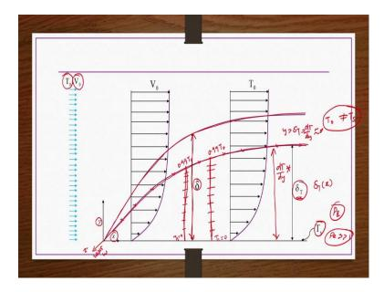
So, that case only we are taking. So, pictorially it is shown here. So, again the horizontal direction is x direction vertical direction is y direction and then z direction in the z direction width is nothing but w right. So, surface temperature  $T_s$  we are taking right; a free stream fluid a fluid moving with a free stream velocity  $V_0$  at temperature  $T_0$ .
