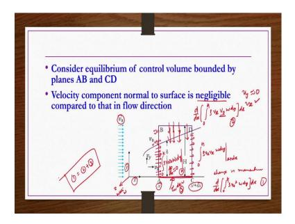
So, now, let us say what is the rate of mass in this control volume let us say AB phase is the inlet phase of the control volume. So, that is nothing but  $\rho v_x$  multiplied by the width multiplied by the area of the plate that is in the z direction since we are taking in the x direction normal to x direction or z and y direction, in the z direction size of the plate or width of the plate is W.
