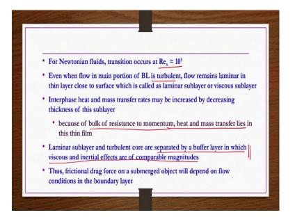
So, for Newtonian fluids, transition from laminar boundary layer to turbulent boundary layer occurs approximately at  $R_{ex}$  = approximately 10<sup>5</sup>. Even when flow in main portion of boundary layer is turbulent flow remains laminar; in thin layer close to surface which is called a laminar sub layer or viscous sub layer. Interface heat and mass transfer rates may be increased by decreasing the thickness of the sub layer.
