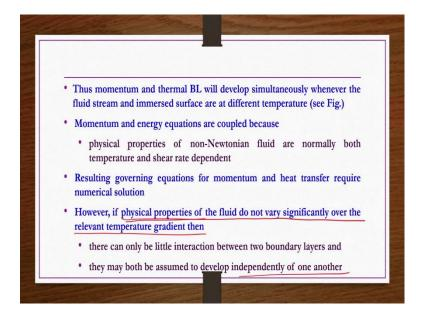
Thus, momentum and thermal boundary layer will develop simultaneously whenever the fluid stream and the immersed surface are at different temperatures, we are going to see the picture also. Momentum energy equations are coupled in general especially for non-Newtonian fluids.
