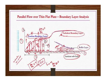
So, we have a flat plate in x direction this slanted lines whatever are shown here you know these lines so, that indicates the solid surface like this right. So, here the coordinate system we have taken such a way that horizontal axis is x axis vertical axis is y axis. And there is a fluid which is coming or flowing at a free stream velocity  $V_0$  right and then velocity component in the horizontal is  $v_x$ , velocity component in the vertical y direction is  $v_y$  ok.
