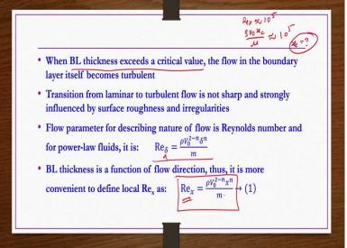
However, when boundary layer thickness exceeds a critical value at x c the flow in the boundary layer itself becomes turbulent. So, this transition from laminar to turbulent boundary layer occurs at Re<sub>x</sub> approximately 10<sup>5</sup>. So, that is if the fluid is Newtonian ok for Newtonian fluid  $\frac{\rho V_0 x_c}{u}$  is approximately 10<sup>5</sup>.
