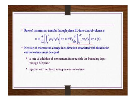
So, the rate of momentum transfer through BD plane into control volume would be nothing but  $\frac{d}{dx} \left[ \int_0^H \rho v_x V_0 \, dy \right] dx$ . So, net rate of momentum change in x direction associated with fluid in the control volume must be equal to rate of addition of momentum from outside the boundary layer through BD plane, together with the net force acting on control volume.
