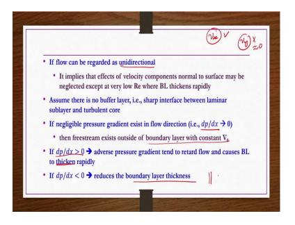
If we can regard as unidirectional flow; that is now we are going to develop integral momentum equation. So, that we are doing for unidirectional flow where we have only  $v_x$  that is in the flow direction velocity component  $v_x$  is there that is predominating. Whereas the other direction  $v_y$  is not there or approximately 0 because it is very small compared to the  $v_x$  right.
