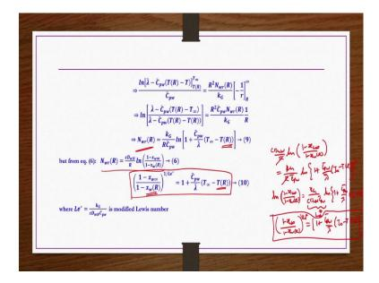
Then you get this expression  $\frac{k_G}{R\bar{C}_{pw}} ln \left[ 1 + \frac{\bar{C}_{pw}}{\bar{\lambda}} (T_{\infty} - T(R)) \right]$  right. So, left hand side right hand side after substituting the limits this is what we get for the  $N_{wr}$ . Now,  $N_{wr}(R)$  we got as function of surface temperature T (R) right.
