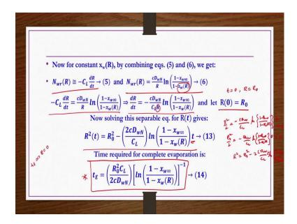
So, now equation number 5 this is there and then this is there. So, all these analysis after the equation number 6 we did in order to find out what is this  $x_w$  (R). We found that it is independent of R that is independent of the size of the droplet so then we can directly equate these two equations and then do the integration to find out R as function of time.
