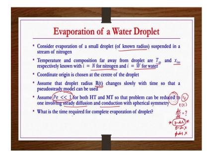
So, consider evaporation of a small droplet of known radius suspended in a stream of nitrogen. Temperature and composition far away from droplet are  $T_{\infty}$  and then  $x_{i\infty}$ . Now,
