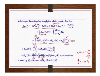
So, what we do? This combined flux we go back to the basics of combined flux so we write a combined flux equation right. When we write combined flux equation that is  $N_{wr}(r) = -cD_{wN}\frac{dx_w}{dr} + x_w(N_{wr} + N_{Nr})$  right. Here  $D_{wN}$  is nothing, but diffusivity of water vapour in the nitrogen gas ok.
