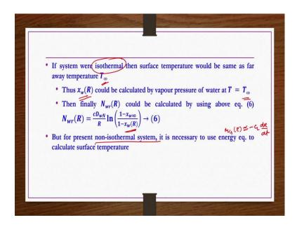
Now, if system were isothermal then surface temperature would be same as far away temperature  $T_{\infty}$  then; obviously,  $x_w$  we could have got it by vapour pressure of water evaluating at  $T = T_{\infty}$ . And then that  $x_w$  (R) we could have substituted in this equation number 6 and then also we could have found what is this  $N_{wr}$  (R) and then equate to the equation number 5 that is  $N_{wr}$  (R) = or approximately equals to  $-C_L \frac{dR}{dt}$ .
