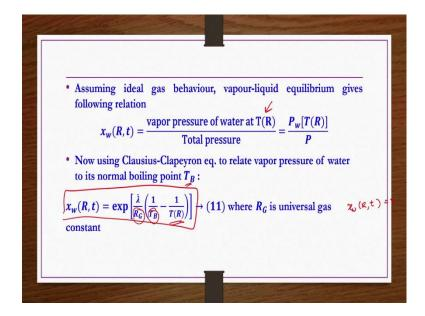
Assuming ideal gas behaviour and then vapour liquid equilibrium gives as the following relation  $x_w$  (R, t) is nothing, but vapour pressure of water at T (R) divided by the total pressure ok. And now using the Clausius-Clapeyron equation to relate vapor pressure of water to its normal boiling point  $T_B$  we can have this expression.
