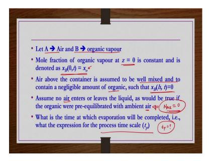
Additional details if you see we are taking air as A and then organic vapour as B. Mole fraction of organic vapour at z = 0 is constant and it is  $x_0$  actually it should be time of actually it should be function of time as well not only position. So,  $x_B$  (0, t) is  $x_0$  ok.
