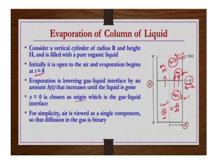
So, first problem we will be discussing evaporation of column of liquid right. So, here we have a cylindrical column whose radius is R and then height is H right. So, in this one initially a liquid which is organic in nature so, that is filled in so, that we are designating with B and then outside there is air.
