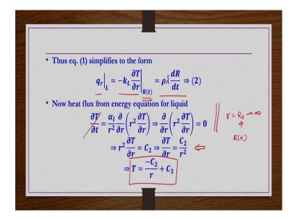
And then this  $q_r|_L$  is nothing but  $-k_L \frac{\partial T}{\partial r}$  at r = R (t). So, now, we have to find out what is  $\frac{\partial T}{\partial r}$  for the liquid side. So, similar energy equation we have to write for the liquid side. So, that heat flux from energy equation for liquid for the liquid side also the energy equation is nothing but having only conduction terms.
