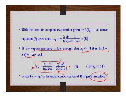
So, that if you substitute here you get  $t_p = -\frac{C_L}{2c} \frac{H^2}{D_{AB}} \frac{1}{\ln(1-x_0)}$  ok. Now, if the vapour pressure is low enough then  $x_0$  would be usually very very smaller than 1 under such conditions we can write  $\ln(1-x_0) \approx -x_0$ .
