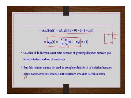
When you substitute the limits and then simplify you get  $N_{Bz}$  is equals to this and then finally,  $N_{Bz}$  at some given t time t is  $-\frac{cD_{AB}}{h(t)}\ln(1-x_0)$  right. So, now this is the final flux equation for component B if you simplify this equation you can get the probably required time to get the complete evaporation done. So, that we can do only when this h(t) is known right so, otherwise we cannot use this equation that we are going to do anyway.
