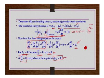
So, now the question is that determine R as function of time and then melting time  $t_p$  assuming pseudo steady conditions right. So, the interfacial balance if you do. The  $q_r$  in the crystal side. So, that is what we are having here also we have a crystal and then there is a surrounding liquid.
