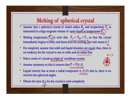
Now, we take another problem melting of spherical crystal ok we have a spherical crystal it is having the initial radius  $R_0$  it is gradually you know melting. So,  $R_0$  whatever initial radius is there that gradually decreases. So, R is function of time ok. So, how much time it required for the complete melting of the spherical crystal that is what we are going to see in this problem ok.
