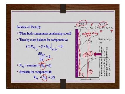
Same horizontal axis is y axis and then condensable vapors are coming in this direction. And then they are reaching the cold surface upon reaching the cold surface they are condensing on the cold surface. At cold surface that is at y=0 T is  $T_0$   $x_A$  is  $x_{A0}$  and then at  $y=\delta$  T is  $T_\delta$   $x_A$  is  $x_{A\delta}$  because the film thickness is  $\delta$  now both A and B are coming and condensing on the vapors.
