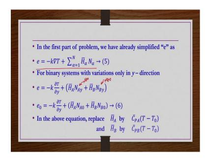
Now, here e up to this point we have simplified in the part a right. So, it is same here also exactly same right now what we do? This one we write for the binary component then we have  $-k\frac{\partial T}{\partial y} + \overline{H}_A N_{Ay} + \overline{H}_B N_{By}$  right.
