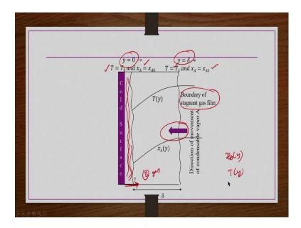
So, pictorially we have a cold surface here which is designated as y = 0 and then close to this one there is a boundary of stagnant gas film made up of B right. So, now the direction of diffusion or you know condensable vapor is coming in this direction and then reaching this cold surface and then condensing like this here right fine.
