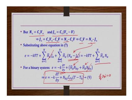
But we know that  $N_{\alpha} = C_{\alpha}V_{\alpha}$  and  $J_{\alpha} = C_{\alpha}(V_{\alpha} - V)$  this we have already seen in the beginning in the first lecture of mass transfer part right. Now, this  $J_{\alpha}$  if I expand  $C_{\alpha}V_{\alpha} - C_{\alpha}V$ .
