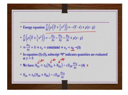
So, now energy equation simplification of energy equation is exactly the same as we have done previously right so, but that  $\frac{\partial e_y}{\partial y} = 0$  and then  $e_y = e_0$  at constant we do not know we are calling it  $e_0$ . Now, the combined flux equation is given here. So, now, here in place of  $N_{Ay}$  you have to write  $N_{A0}$  and then in place of  $N_{By}$  you have to write  $N_{B0}$  right. So, when you write you get this equation.
