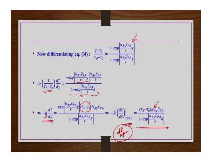
Now, differentiating with respect to y so, in the left hand side  $\frac{1}{T_{\delta}-T_0}$  is you know constant then  $\frac{dT}{dy}-0$  =. And then in the right hand side except this particular term all other terms are independent of y. So, in the denominator we are keeping as it is numerator when you are differentiating this term exponential of x is exponential of x on differentiation.
