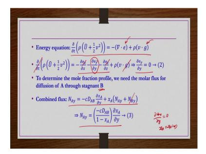
Energy equation we have derived in an equation we have derived in week number 4. So, this is what we have got. Whereas this e is there in all 3 direction x y and z direction and then each e and it consist of a contribution from the conduction convection work done because of the pressure you know viscous dissipation etcetera all those terms are included in all three directions right.
