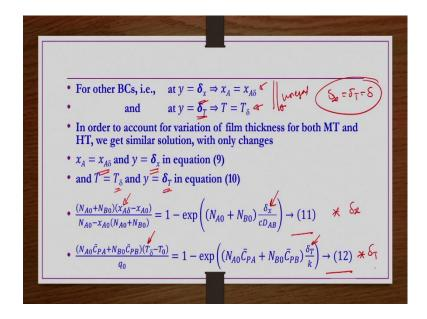
Now, what we do? The limiting conditions of you know unequal film thickness if the film thickness are unequal then at  $y = \delta x x_A = x_{A\delta}$  this is for the mass transfer part right. So, film thickness for the mass transfer part whatever is there  $\delta x$ .
