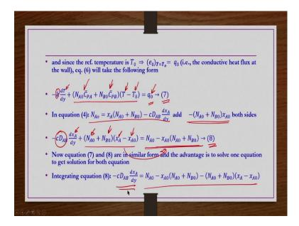
So, that is  $-k\frac{\partial T}{\partial y} + N_{A0}\bar{C}_{PA} + N_{B0}\bar{C}_{PB}$  multiplied by  $\delta T = e_0$  that  $e_0$  we are evaluating it  $T = T_0$ . So, then at that point we have only conductive heat flux at the wall there is no mass transfer so, that we calling  $q_0$  ok.
