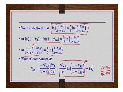
Now, what we do? We differentiate this equation with respect to y because we wanted to know the flux also, we have to find out the mass flux also for that we need to know  $\frac{dx_A}{dy}$ . So, that is the reason we are differentiating this equation with respect to y. So, so this from this term what we have  $\frac{1}{1-x_A}\left(-\frac{\partial x_A}{\partial y}\right)$  this is constant. So, 0 derivative of constant is 0.
