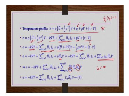
Now, we try to get the temperature profile. So, what we got by simplifying the energy equation we got  $\frac{\partial e_y}{\partial y} = 0$ , but what is the  $e_y$  we have not simplified in that slide. So, that we are doing here. So, the e is having the contribution from the conduction convection then any work done because of the pressure. And then any molecular stress you know energy because of the molecular stresses like you know viscous dissipation etcetera those terms are included.
