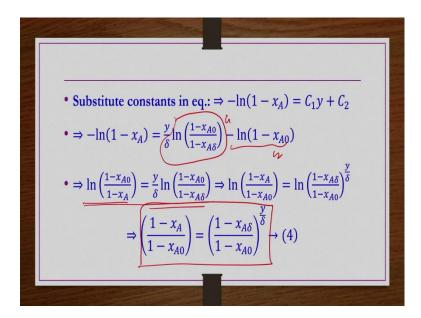
In this term is  $C_1$  and then this term is  $C_2$  right then if you further simplify in the sense what we do we take this  $-\ln(1-x_{A0})$  to the left-hand side. So, that we can write  $\ln\left(\frac{1-x_{A0}}{1-x_A}\right) = \frac{y}{\delta} \ln\left(\frac{1-x_{A0}}{1-x_{A\delta}}\right)$ .
