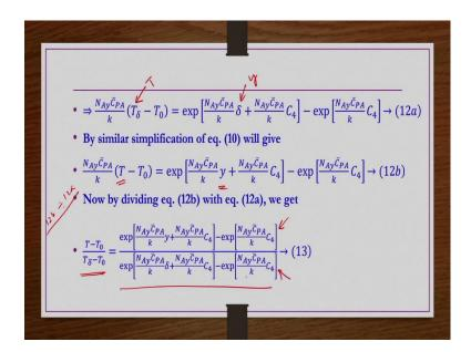
So, now what we do? We need to have  $(T - T_0)$  also. So, that in place of  $T_\delta$  we write T and in place of  $\delta$  we right y right. Because at  $y = \delta T = T_\delta$  and then at y is equals to some unknown y T is equals to some unknown T right so, that if you do you get this equation.
