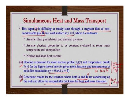
So, consider a hot vapor A is diffusing at steady state through a stagnant film of non-condensable gas B to a cold surface at y = 0 where A condenses. So, hot vapor A is condensing on a cold surface, but when it reaches the cold surface in between there is a stagnant film of non-condensable gas B and this A is diffusing into B when it reaches to the cold surface and condenses in that process ok.
