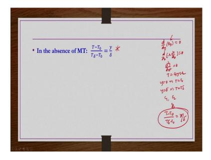
But if there is no mass transfer, if there is no mass transfer then in the absence of mass transfer temperature profile is linear that is this one how do you get? So, if there is no mass transfer  $\frac{\partial e_y}{\partial y} = 0$  and then  $e_y$  would be having only  $-k\frac{\partial T}{\partial y}$  term only we will be having right.
