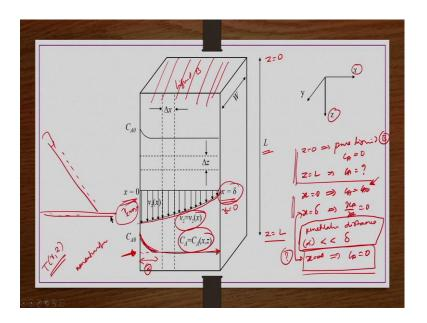
So, now pictorially if you see three-dimensional projection is shown here, so the horizontal axis is x, vertical axis is z right. So, the height of the column is L, width of this column is W through which along which the material is flowing down. So, there is A, this material whatever is there that B liquid is there. So, that is falling like a film here right. And now into this film the diffusion of component A is gas component A is taking place.
