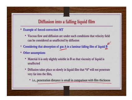
So, this is an example of forced convective mass transfer as explained. Where viscous flow and diffusion are under such condition that velocity field can be considered as an affected by the diffusion. That is momentum transfer is not affected by the mass transfer, but mass transfer is affected by the momentum transfer, ok.
