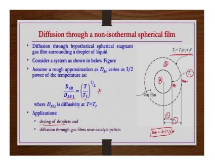
Diffusion through hypothetical spherical stagnant gas film surrounding a droplet of liquid; that is the problem you know statement. So, consider this system as shown here in the picture. So, we have a droplet which is made up of the component A and then gas film component B is there, the radius of droplet is  $r_1$ , the radius of gas film surrounding this droplet is  $r_2$ , ok.
