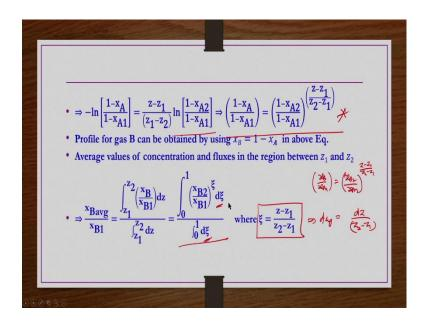
So, that we have  $-ln\left[\frac{1-x_A}{1-x_{A1}}\right] = \frac{z-z_1}{(z_1-z_2)}ln\left[\frac{1-x_{A2}}{1-x_{A1}}\right]$ . So, the same thing we can write like this equation. So, this is the concentration profile that we suppose to obtain between locations  $z_1$  and  $z_2$ .
