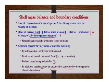
Now, shell balance and then boundary conditions in general that are useful to solve the mass transfer problems associated with the diffusion for as well as the bulk motion and chemical reaction that is what we are going to see. Because, now we see the basics and then after that we can take different types of problems associated as per you know problem.
