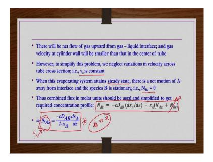
So, there will be net flow of gas upward from gas liquid interface and gas velocity at cylinder wall will be smaller than that in the center of the tube, because flow through pipes or tubes what we have seen you know there is a velocity profile developed across the cross section even if the L/D is very large.
