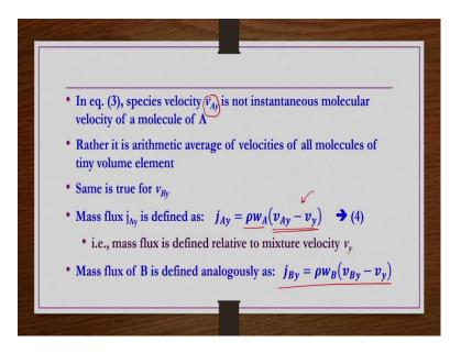
Then in equation 3 species velocity  $v_{Ay}$  is not instantaneous molecular velocity of molecule A as mentioned, rather it is arithmetic average of velocities of all molecules of tiny volume element. Within the tiny element whatever we are doing this analysis, whatever the A component you know moving in y direction, all the velocities have been taken as a kind of consideration and then their arithmetic average is reported as  $v_{Ay}$  same is true for  $v_{By}$  as well.
