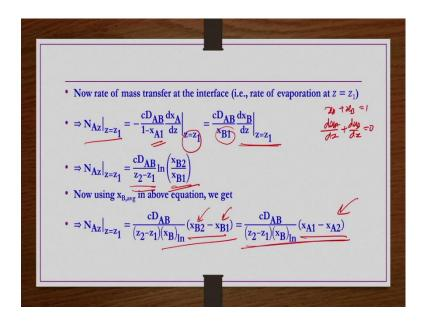
So, now rate of mass transfer at the interface that is rate of evaporation at  $z = z_1$  if you wanted to find out that is  $N_{Az} = \text{ or } N_{Az}$  at  $z = z_1 = -\frac{cD_{AB}}{1-x_A}$ , but now we are evaluating it at  $z = z_1$ . So, this  $x_A$  should be replaced by the  $x_{A1}$  multiplied by  $\frac{dx_A}{dz}$ . And then this  $-\frac{dx_A}{dz}$  is nothing but  $+\frac{dx_B}{dz}$  because it is a binary system only where  $x_{A+} x_B = 1$ .
