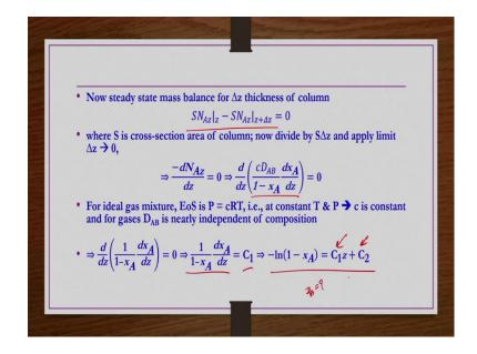
So, that we can get by the balance. And now steady state mass balance for  $\Delta z$  thickness of column we do  $SN_{Az}$  at  $z - SN_{Az}$  at  $z_{+}\Delta z = 0$ , S is nothing but the area through which; area of the column or the very area of the thickness of the column through which diffusion is taking place. And then luckily and then in our system the area is not changing across the column height ok.
