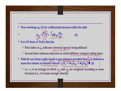
Now the same equation if you write for a differential element within this slab. So, then how we can write? You can write  $-\rho D_{AB} \frac{dw_A}{dy}$  why this minus is coming? Because we know this mass transfer occurring from higher concentration region to the lower concentration region and then the as the y increases the concentration is decreasing. So, that is the reason negative concentration gradient is there. So, we have to have a minus here right.
