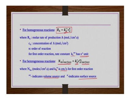
So, let us say for homogeneous reactions rate of production we can represented; we can represented by this expression  $R_A = k_n^{\prime\prime\prime} c_A^n$ . Where  $R_A$  is the molar rate of production of A, c<sub>A</sub> is concentration of A, n is the order of reaction. If first order reaction then rate constant  $k_n^{\prime\prime\prime}$  has second inverse of units ok.
