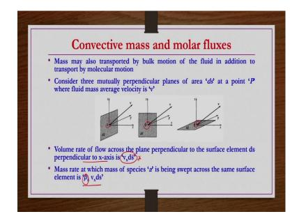
So, now expression for convective mass and molar fluxes. The flux is by convection, but we are going to write it in both mass and molar units. That is the reason it is convective mass flux and then convective molar flux. Mass may also be transported by the bulk motion of the fluid in addition to the transport by molecular motion. That we understand.
