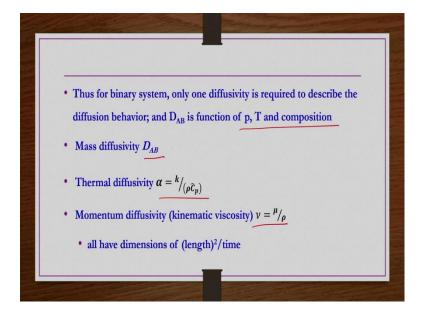
Thus for a binary system only one diffusivity is required to describe the diffusion behavior and then  $D_{AB}$  is function of temperature pressure and composition. So, what we have this mass diffusivity  $D_{AB}$ ? Earlier we have thermal diffusivity  $\alpha$  that is  $k/\rho \hat{C}_p$  and then before that we have the momentum diffusivity or kinematic viscosity  $\nu = \mu/\rho$ . So, all of them are having the units you know length square per time right.
