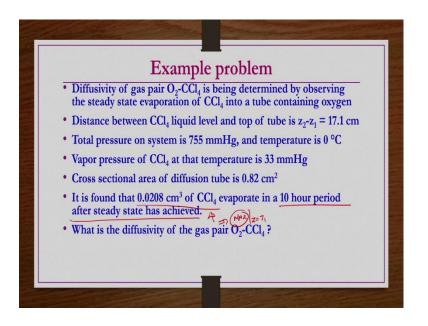
Now, we wind up today's class with a simple example problem using the previous expression that we have taken diffusion through non-stagnant gas film. So, diffusivity of gas pair O<sub>2</sub> CCl<sub>4</sub> is being determined by observing the steady state evaporation of CCl<sub>4</sub> into a tube containing oxygen. Distance between liquid level and top of the tube is 17.1 centimeter that is  $(z_2 - z_1)$  is given.
