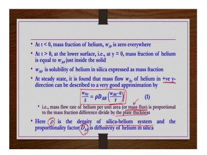
So, finally, at steady state it is found that mass flow  $w_{Ay}$  of helium in positive y direction can be described to a very good approximation by  $\frac{w_{Ay}}{s}$  this is nothing but the flux and then it is proportional to the concentration gradient that is given by  $\frac{w_{A0}-0}{y}$ . Why 0 here? Because  $w_A = 0$  at y = Y ok and then at y = 0  $w_A = w_{A0}$ . So, the concentration gradient is given by this expression, right.
