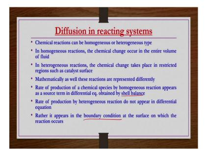
So, now what if diffusion in reacting system? So, if there is a mass transfer <sub>+</sub> there is a reaction also taking place. So, then reactions can be categorized in different ways, but now with respect to the problems that we are dealing with the mass transfer combined with
