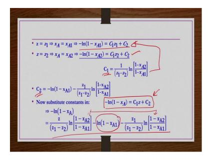
So, we already have two boundary condition at  $z = z_1 x_A = x_{A1}$ . So, this equation you get now  $z = z_2 x_A = x_2$ . So, then this equation you get. Now if you subtract this equation second equation from the first equation you get  $C_1 = \frac{1}{(z_1 - z_2)} ln \left[ \frac{1 - x_{A2}}{1 - x_{A1}} \right]$ .
