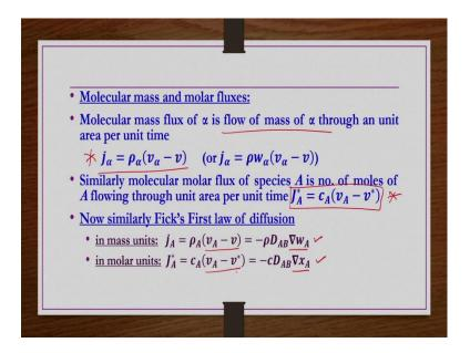
Molecular mass and molar fluxes. Molecular mass flux of  $\alpha$  is a flow of mass  $\alpha$  through an unit area per unit time. So that means,  $j_{\alpha} = \rho_{\alpha}(v_{\alpha} - v)$  that we have already seen.
