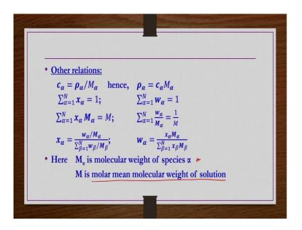
Other relations amongst this  $c_{\alpha} \rho_{\alpha}$  etcetera are provided here which are all well known to us, ok.  $M_{\alpha}$  is nothing but the molecular weight of species  $\alpha$  here whereas, M is the molar mean molecular weight of solution ok. It is not the molecular weight of one component, but the molar mean molecular weight of the solution whatever number of components are there. So, that should be considered.
