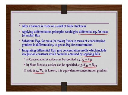
After a balance is made on a shell of finite thickness what we do? We apply differentiation principles and would get differential equation for mass flux or molar flux, right. Then substitute equations for mass flux or molar fluxes in terms of concentration gradient in differential equations to get an equation for the concentration. We when we solve these problems we can easily understand.
