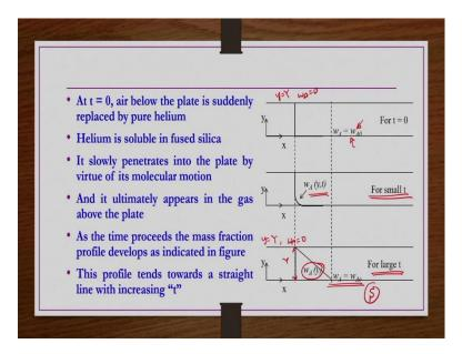
So, whatever we have discussed in the previous slide have been shown pictorially. So, at t = 0 helium has been introduced at the bottom of the plate fused silica horizon plate. So, the very first layer within the fused silica whatever is there that very first layer now helium is there at t = 0 that concentration in terms of mass fraction we are writing  $w_{A0}$ .
