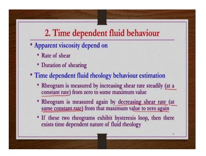
Now, after reaching some maximum value of shear rate rheogram is again measured by decreasing shear rate from that maximum value to zero value, but at the same constant rate at the same constant rate. Whatever rate you increase the shear rate to reach the maximum shear rate information or maximum shear rate value at the same rate you have to decrease the shear rate to come back to zero shear rate value.
