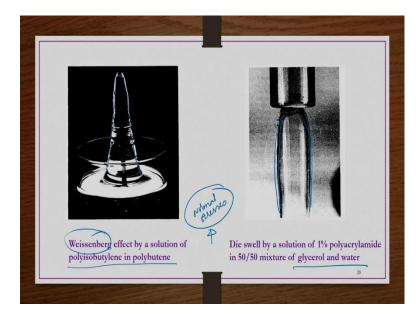
The material is climbing along this rod of the steerer. So, this is known as the Weissenberg effect of a solution of a polyisobutylene propylene. This is first reported by the scientist Weissenberg. Similarly die swell so, you can see the material when it is release so, and then it is swelling slightly right.
