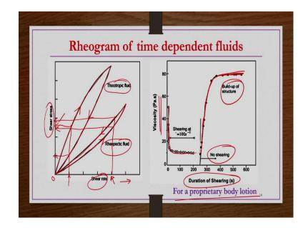
Now, rheogram of time dependent fluids as I already mentioned shear stress versus shear rate information you have to get for a you know for an increasing shear rate. Let us say increasing shear rate from 0 to some maximum value of shear rate you are increasing right.
