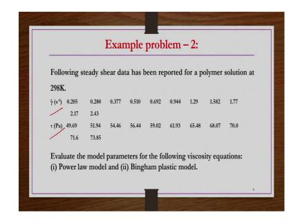
So, we take another example problem. Following study shear data has been reported for a polymer solution at 298 Kelvin. So,  $\dot{\gamma}$  is given in  $s^{-1} \tau$  is given in Pascal right. The question is evaluate the model parameters for the following viscosity equations power law model and then Bingham plastic model.
