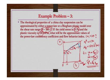
So, example problem number 3. The rheological properties of a china clay suspension can be approximated by either a power law or a Bingham plastic model over the shear rate range of 10 to 100  $s^{-1}$ . If the yield stress is 15 pascals and a plastic viscosity is 150 millipascal second. What will be the approximate values of the power law consistency coefficient and then flow behaviour index?
