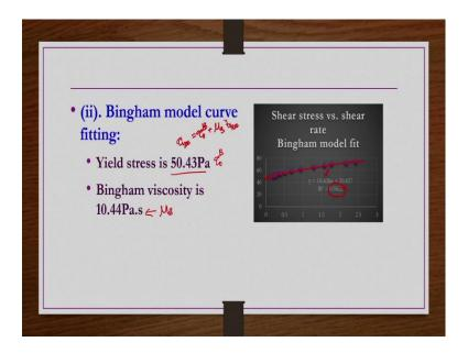
So, next part is that the same data we have to fit using Bingham model curve fitting. So, Bingham model curve fitting what we have?  $\tau_{yx} = \tau_0^B + \mu_B(\dot{\gamma}_{yx})$  that is it. So, if you plot it linearly you get a straight line like this.
