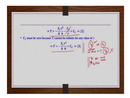
So, the same equation is written here again. So, the  $\,$ C must be 0 in this case because this temperature cannot be infinite for any value of r. And then if you substitute r=0 that is at the centre you this equation is going to produce the infinite value that is not acceptable. So,  $C_1$  must be 0. So, the final simplified temperature is this one right.
