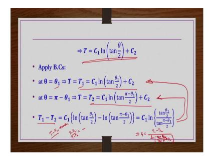
Now this even  $C_2$  we have to find out using the boundary conditions that we are having. The same temperature, expression is written again here. At  $\theta = \theta_1$ ,  $T = T_1$  that is given. So,  $T_1 = C_1 \ln \left( \tan \frac{\theta_1}{2} \right) + C_2$  right. At  $\theta = \pi - \theta_1$   $T = T_2$  that is also given.
