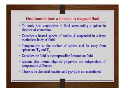
So, heat transfer from a sphere to a stagnant fluid. So, the purpose is to study the heat conduction in fluid surrounding a sphere in absence of convection because we are taking infinitely bounded stagnant Newtonian fluid. Since it is stagnant there will not be any convection. So, consider a heated sphere of radius R suspended in a large motionless body of fluid right. Temperatures at the surface of sphere and far away from the sphere are  $T_R$  and  $T_\infty$  respectively.
