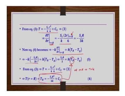
So, from equation number 3 we are finding out  $\frac{\partial T}{\partial r}$  because we have to find out  $-k\frac{\partial T}{\partial r}$ . So,  $\frac{\partial T}{\partial r}$  from equation number 3 is  $-\frac{S_C}{k}\frac{2r}{6}$  and then this  $\frac{\partial T}{\partial r}$  we are finding out at r = R that is at this surface. So, you substitute r = R then you get  $-\frac{S_CR}{3k}$ .
