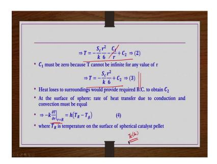
So, heat losses to surroundings would provide required boundary condition to obtain  $C_2$ . So, what are the heat losses that we have to find out? At the surface of sphere rate of heat transfer due to conduction and convection must be equal in order to find out the new boundary condition to get this  $C_2$ . So, we have to find out rate of conduction at the surface as well as the rate of convection at the surface to get a final boundary condition.
