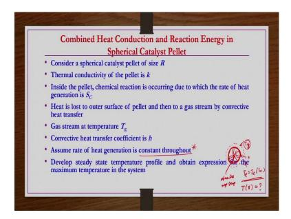
So, now, combined heat conduction and reaction energy in spherical catalyst pellet. So, that is the last problem that we are taking in this class ok. So, let us say this statement. Consider a spherical catalyst pellet of size R. Thermal conductivity of the pellet is k. Inside the pellet chemical reaction is occurring due to which the rate of heat regeneration is S<sub>C</sub>.
