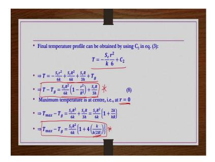
So, now, this C<sub>2</sub> you can substitute in equation number 3, which is the final temperature distribution  $T = -\frac{S_C}{k} \frac{r^2}{6} + C_2$ , in place of C<sub>2</sub> we can write  $\frac{S_C}{k} \frac{R^2}{6} + \frac{S_CR}{3h} + T_g$ . So,  $T - T_g = \frac{S_C}{k} \frac{R^2}{6} + \frac{S_CR}{3h} + \frac{S_C$
