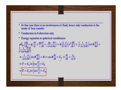
In this case there is no involvement of fluid, hence, only conduction is the mode of heat transfer. Conduction would also be there only in  $\theta$  direction, it will not be there in r and  $\phi$  direction according to schematic given. And then energy equation in spherical coordinates we have to simplify since steady state.
