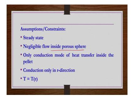
So, assumptions constraints, steady state problem we are taking, negligible flow inside porous sphere so, that we can take only conduction in general. Because inside the porous structure whatever the catalyst pellet you take inside the porous structure in general these reactants whether the gases or liquid reactants whatever are there they move they are moved from one location to the other location primarily because of the diffusion.
