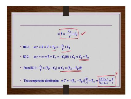
So, this is the temperature profile that we got. Now, we will obtain these constant  $C_1$ ,  $C_2$ . At r = R  $T = T_R$ . So,  $-\frac{c_1}{R} + C_2 = T_R$ . And then at  $r = \infty$ ,  $T = T_\infty$  that is  $-\frac{c_1}{\infty}$  that is  $0 + C_2$  so; that means,  $C_2 = T_\infty$  we get.
