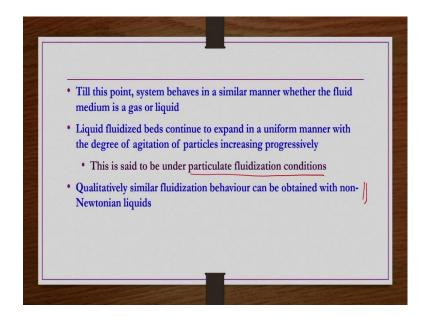
Till this point, system behaves in a similar manner whether the fluidizing medium is gas or liquid. So, the till that point where the pressure drop start becoming constants. So, that point we called as a minimum fluidized conditions. The point at which the pressure drop start becoming constant even if you increasing the velocity volumetric flow rate. So, that point we call it as a point of incipient fluidization right.
