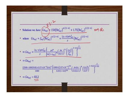
So, this is the equation that we have here in this equation Galileo number is given by this one. After simplifying substituting  $Re_{mf}^*$  and then simplifying what we get? Galileo number we got this expression. Now here in this equation when you substitute all these numbers. So, then you get Galileo number is 83.2; this 80 through; 83.2 you substitute here and then solve this equation for  $Re_{mf}^*$ .
