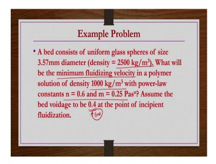
So, a bed consists of uniform glass spheres of size 3.57 mm diameter density of particle is given this one. What will be the minimum fluidizing velocity in a polymer solution of density? Fluid density is given this one,  $\rho$  is given this one, and then fluid is a power law fluid with these constants. Assume the bed voidage is 0.4 at incipient
