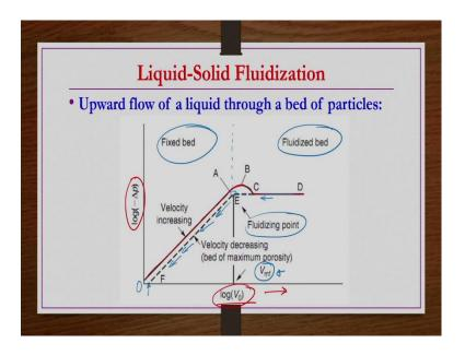
So, then obviously, it has to be upward flow, because upward flow only then it is possible that the fluidization of the particle is taking place right.
