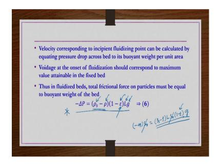
So, velocity corresponding to incipient fluidization point can be calculated by equating the pressure drop across the bed to its buoyant weight per unit area. So, voidage at that; at the onset of fluidization should be correspond to the maximum value attainable in the fixed bed, but minimum value in the case of a fluidized bed.
