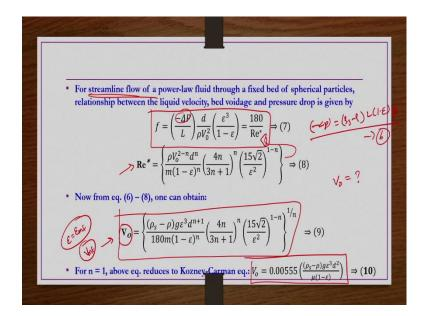
Then for streamline of flow of power law fluid through a fixed bed of spherical particles relation between the liquid velocities, bed voidage and pressure drop; we have already calculated in the previous lecture. And then that is given by this expression right.
