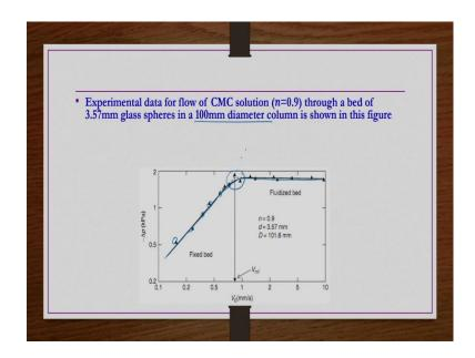
So, one example we take a CMC solution 0.9 and then it is pass through a bed of 3.57 mm glass spheres and then packing A has been done in 100 mm diameter column. Then the experiments have been carried out whatever the  $-\Delta P$  versus  $V_0$  information is there that has been plotted on a log-log scale.
