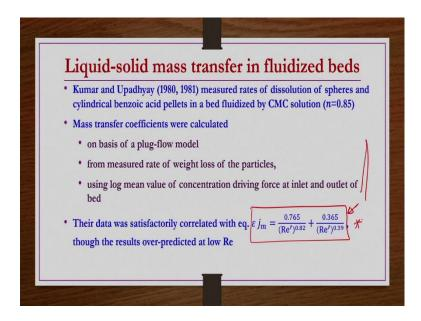
So, liquid-solid mass transfer in fluidized beds, here also very limited you know studies are available. Kumar and Upadhyay measured rates of dissolution of spheres and cylindrical benzoic acid pellets in a fluidized bed by CMC solution of only n value 0.85.
