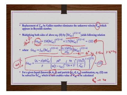
So, what we do? A replacement of  $f_{mf}$  by Galileo number eliminates the unknown  $V_{mf}$  which appears in the Reynolds number for that what we do? In the equation number previous equation number  $f_{mf} = 150/Re_{mf}^* + 1.75$  you are multiplying both sides by  $\left(Re_{mf}^*\right)^{2/(2-n)}$ .
