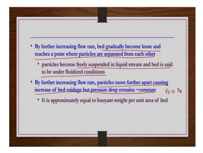
By further increasing the flow rate what happened? Bed gradually becomes loose and reaches a point where the particles are separated from each other and then particles become freely suspended in liquid stream and bed is said to be under fluidized conditions.
