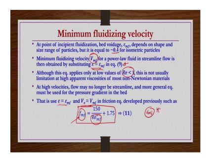
So, minimum fluidization velocity at the point of incipient fluidization bed voidage  $\varepsilon$  mf depends on shape and size and; shape and size range of particles, but it is equals to approximately 0.4 for isometric particles in general. Minimum fluidization velocity
