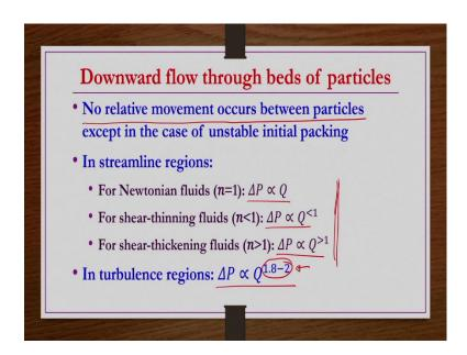
If the initial packing is not properly stable; not have not been you know properly vibrated and shaken before the packing then that means, the initial packing is unstable. So, under such conditions you know there will not be any relative movement of the particles if the flow is downward.
