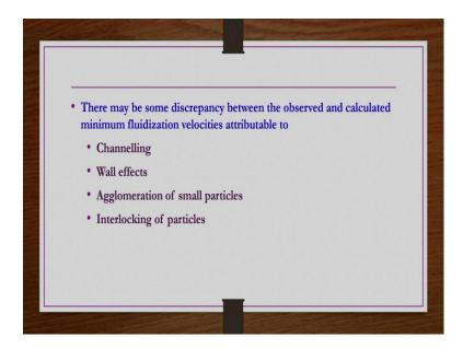
So, there may be some discrepancies obviously, between the observed and calculated minimum fluidization velocities, because the same regions are there for  $-\Delta P$  versus  $V_0$  curves also. These are channeling wall effects, agglomeration of small particles, and then interlocking of particles if the particles are having like needle like shape etcetera.
