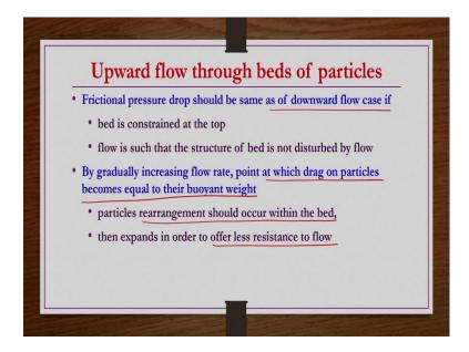
So, now we see the same details again here. So, upward flow through beds of particles the frictional pressure drops should be same as of the downward flow case if under two conditions; one is if the bed is constrained at the top also by a closing perforated plate or the velocity is low such a way that the rearrangement of particle is not taking place; or there will not be any relative movement of the particles if the bed is not constrained at the top. These two conditions.
