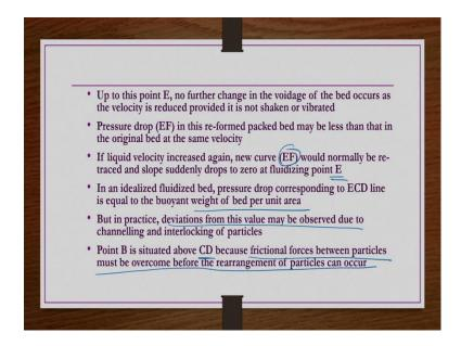
Up to this point E, no further changes in the voidage of the bed occurs as the velocity is reduced provided it is not shaken or vibrated. Then a pressure drop EF in this reformed packed bed may be less than that in the original bed at the same velocity, because of the rearrangement of the bed. If the liquid velocity increased again new curve EF would normally be retraced and slope suddenly drops to zero at fluidizing point E.
