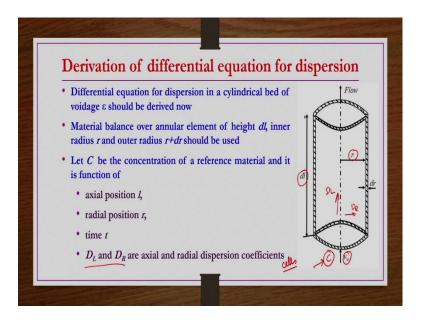
So, now this is the representation of such cells of same size and shape and then they are porous in nature. Shape we have taken cylindrical cell, because there packing we have done in a cylindrical column right. The height of this cell is dl, the inner radius of the cell is r, and outer radius of cell is r + dr. So, that thickness of the cell we can take as dr the material the fluid is entering at  $v_0$  velocity at the bottom and then leaving from the top ok.
