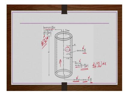
So, pictorially we write quantities that are entering here. So, the rate of material that is entering at the inlet because of the flow is this one  $2\pi r \, dr \, V_0 \, C$ .  $2\pi r \, dr$  is the cross section area of the cell through which the material is entering. And then  $V_0$  is the velocity at which entering, C is the concentration, this is because of the motion bulk motion ok.
