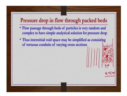
Flow passage through beds of particles is very random and complex to have simple analytical solution for a pressure drop. If you have a simple pipe you know we already have done the analysis, how to get you know pressure drop, velocity profile or volumetric flow rate velocity versus pressure drop calculations etcetera all those things we have already seen.
