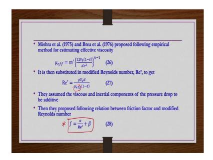
So, what we see? We see a few literature. So, Mishra et al and Brea et al proposed following empirical method for estimating the effective viscosity for a fluid flowing through packed beds that viscosity is given by this one. This is for the case of power-law fluids,
