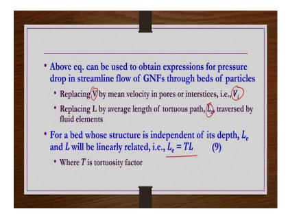
So, now this equation can be used to obtain expression for pressure drop in streamline flow of a generalized Newtonian fluids through beds of particles by replacing V by interstitial or the pore velocity or mean velocity in pores or interstitial spaces  $V_i$ . And then replacing L by average length of tortuous tortures path L<sub>e</sub>. And L<sub>e</sub> is nothing but T L; T is nothing but the tortuosity factor, ok
