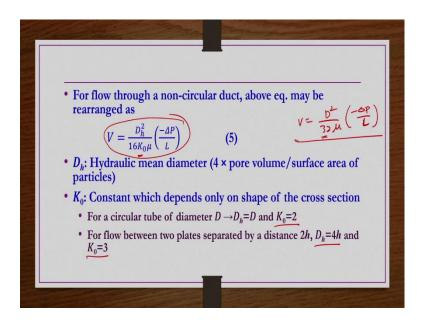
For flow through a non-circular duct above equation may be rearranged as this one ok. The previous equation whatever  $V = \frac{D^2}{32\mu} \left(\frac{-\Delta p}{L}\right)$  was there. This is for the circular column, tubes kind of thing you know Hagen-Poiseuille equation. But, the same equation if you derive for non-circular conduits you get this one. Here D<sub>h</sub> is nothing but hydraulic radius and then this constant K<sub>0</sub> depends on the shape; depends on the shape ok.
