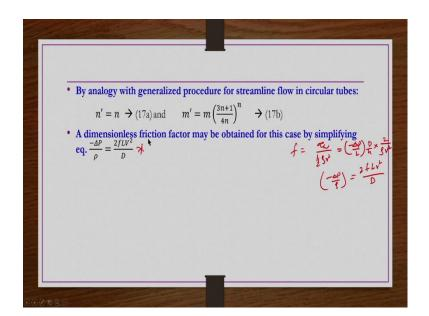
But, m' is  $m\left(\frac{3n+1}{4n}\right)^n$ . So, this m and n without primes they are the rheological parameters of the fluid whereas, n' and then m' are the characteristic parameter that are obtained from the packed bed by doing experiments and then getting the results volumetric flow rate versus pressure drop.
