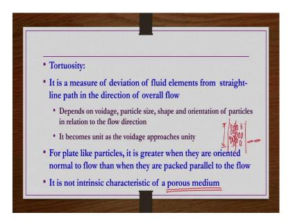
Let us say if the same way same needle like particles. If you packing like this parallel to the flow direction like this the same needle like particle, so then the distance that particle has to transfer it will be still higher than the height of the column, but it will be less than the case where these particles are oriented in the normal direction like this, ok.
