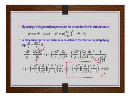
So, now in place of L we have to write L<sub>e</sub>, in place of V we have to write V<sub>i</sub>, in place of D we have to write D<sub>h</sub> for the packed bed. And then corresponding equations that we have already derived in previous slide we substitute here so then you get expression for f as this one;  $f = \left(\frac{-\Delta p}{\rho}\right) \frac{D_h}{2L_e V_i^2}$ .
