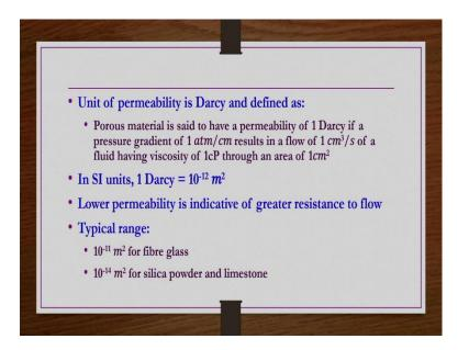
Units for the permeability is Darcy and then it is defined as Porous material is said to have a permeability of 1 Darcy if a pressure gradient of 1 atmosphere per centimeter results in a flow of 1 metre cube per second of a fluid having a fluid viscosity 1 centipoise through an area of 1 centimeter square.
