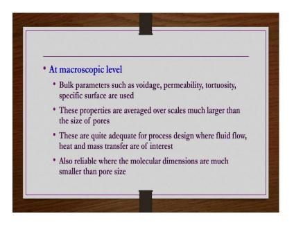
Other level is at macroscopic level. At macroscopic level it is very essential to do proper characterization of the porous material, because most of the transport phenomena problem that exist, in chemical engineering you know we use this macroscopic level characterization.
