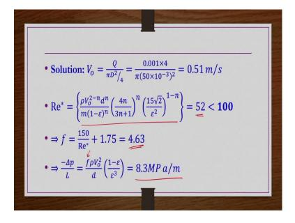
So, if you want to calculate Re<sup>\*</sup> you need V<sub>0</sub> that is you can get by  $\frac{Q}{\pi D^2/4}$ ; Q is given, D is given, column diameter is given. So, V<sub>0</sub> you get 0.51 metre per second, Re<sup>\*</sup> expression is this one. So now, here in this equation  $\rho$ , V<sub>0</sub>, D, n, m,  $\varepsilon$  everything is known, so when you substitute you get 52, so it is less than 100.
