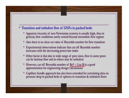
However, for non-Newtonian fluids usually apparent viscosity is higher. So, then in general you do not get very large Reynolds number flows, ok. Also there is no clear cut value of Reynolds number for flow transition in case of packed bed even for the Newtonian case. So, same is valid for non-Newtonian case.
