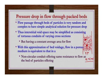
But, having a constant average area for flow which is as same as the case of you know real packed bed. With this approximation of bed voidage flow in porous media is equivalent to that in non-circular conduit offering same resistance to flow as a bed of particles offering.
