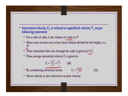
So, interstitial velocity  $V_i$  is related to the superficial velocity  $V_0$ , how it is? It is related like  $V_i = V_0/\epsilon$ , how it is that we see now. For a cube of side 1 the volume of voids is  $\epsilon l^3$ voids or cube if you have a particle is a cube cubical shaped let us say the particle that you are taking it is a cubical shape, then its volume is  $l^3$  if the side of cube is 1.
