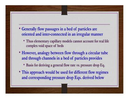
So, generally flow passages in a bed of particles are oriented or interconnected in an irregular manner that we know. Thus elementary capillary models cannot account for real life complex void space of the beds in general.
