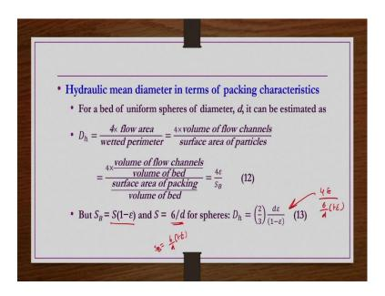
So, hydraulic mean diameter in terms of packing characteristics we have to find out. For a bed of uniform spheres of diameter d it can be like  $D_h = 4$  multiplied by flow area divided by the wetted parameter. So, flow area is nothing but the volume of flow channels ok that is available and then wetted perimeter is nothing but the surface area of particles.
