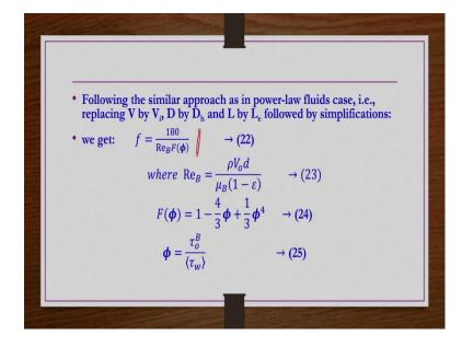
So, like that if you do and then follow the same analysis by replacing V by V<sub>i</sub> and D by D<sub>h</sub> and L by L<sub>e</sub> then do the similar calculation what we have done till now for the case of power-law fluid, then you get  $f = \frac{180}{Re_BF(\phi)}$  as a kind of friction factor for a Bingham plastic fluid flowing through packed beds.
