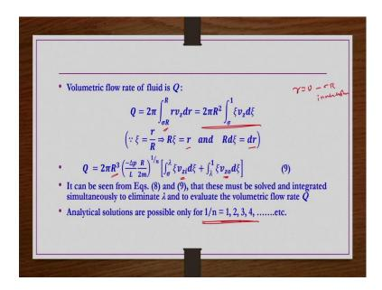
So, now volumetric flow rate then  $Q = 2\pi \int_{\sigma R}^{R} r v_z dr$  it is not 0 to R because 0 to R = 0 to  $\sigma$  R is an inner wall inner cylinder. So, where there is no flow, so that is the region  $\sigma$  R to R is the limiting condition.
