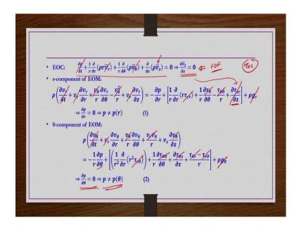
So, continuity equation if you have in cylindrical coordinates that is this one right. So, steady state this term is 0,  $v_r$  is not existing,  $v_r$  is not existing,  $v_r$  is not existing,  $v_r$  is existing and it is function of r only that way also this term is canceled out. But however, we can understand this one other way  $\frac{\partial v_z}{\partial z} = 0$ , because if  $\frac{\partial v_z}{\partial z}$  is existing, so then we can say fully developed flow conditions are existing.
