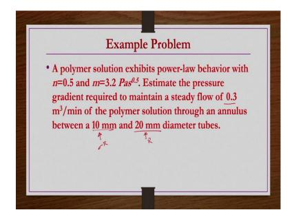
So, a polymer solution exhibits power-law behavior with n=0.5 m is equals to 3.2 pascal second power n. The estimate we have to estimate the pressure gradient required to maintain steady flow of 0.3 meter cube per minute, so Q expression is given. So, the annulus between 10 mm and 20 mm diameter tubes, so this is  $\sigma$  R this is R ok
