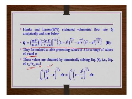
So that, and then Hanks and Larson evaluated volumetric flow rate analytically and is given by this expression, we are not going to derive this equation. So, this is the analytically the Hanks and Larson have obtained volumetric flow rate for this geometry, for the power law fluids right.
