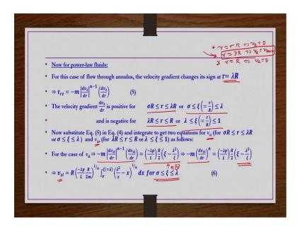
So, as per the geometry what we have? From  $r = \sigma R$  to  $r = \lambda R$  the velocity gradient you know it is a positive. Because at  $r = \sigma R$  we are having  $v_z = 0$ , at  $r = \lambda R$   $v_z = v_{z \text{ max}}$  right.
