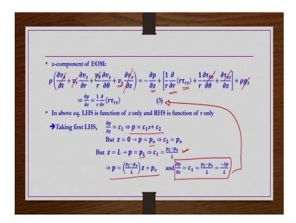
So, z component of momentum equation written here. So, because of the steady state this term is 0,  $v_r$  is 0,  $v_\theta$  is 0,  $v_z$  is existing but  $v_z$  is function of r only and then from the continuity equation we understand  $\frac{\partial v_z}{\partial z}$  is 0 right. Pressure we do not know, so let us keep it as it is.
