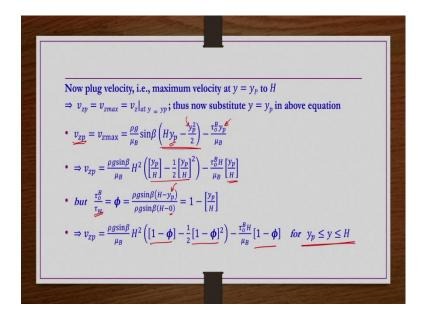
So, that  $v_{zp}$  you can get by substituting  $y = y_p$  in  $v_z$  expression that just we got. So, in the  $v_z$  here in place of y we have written  $y_p$ , here also in place of  $y^2$  we have written  $y_p^2$ , here also here also in place of y we have written  $y_p$  and then  $v_z$  is nothing  $v_{zp}$  right. So, now,  $v_{zp} = \frac{\rho g \sin \beta}{\mu_B}$ .
