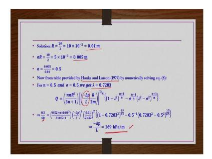
So, now we see the solution diameter of the outer wall or outer tube is given that is 20 mm, so its radius would be 10 mm, so that is 0.01 meters. Similarly diameter of inner tube is given as 10 mm, so its radius would be a 5 mm. So,  $\sigma$  R would be 0.005 m because diameter
