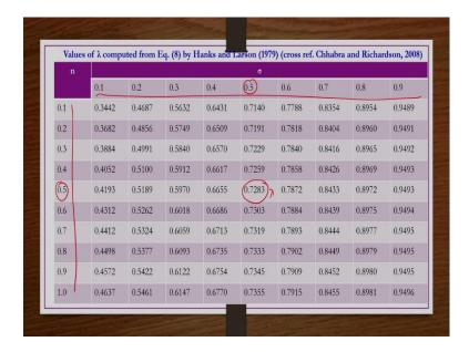
So, that  $\lambda$  values are tabulated here right. For different n values and then different  $\sigma$  values given here you know the corresponding  $\lambda$  values are given here right. Let us say if n=0.5 and then  $\sigma$  is also 0.5. So, the  $\lambda$  value is 0.7283 right.
