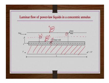
So, now we take another geometry; the another geometry that we are taking is concentric annulus ok; laminar flow of power law liquids in concentric annulus. So, this is the geometry, what we have? We have two cylinders, so one cylinder outer cylinder is having the radius R, another inner cylinder having the radius  $\sigma$  R right. So, these between these two cylinder there is a gap, annulus gap is there within that annulus gap what happened, the fluid is flowing the fluid is flowing.
