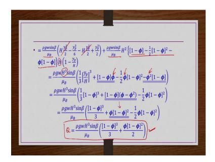
Now, volumetric flow rate we can get by integrating this  $v_z$  multiplied by w; dy w is nothing but the width of the fluid or the width of the fluid that is extended in the x direction. So,  $Q = \int_0^H v_z w dy$  and then now this  $v_z$  is having two components  $v_z$  as function of y to  $y_p$  point; 0 to  $y_p$  point and then  $v_{zp}$  from  $y_p$  to H point.
