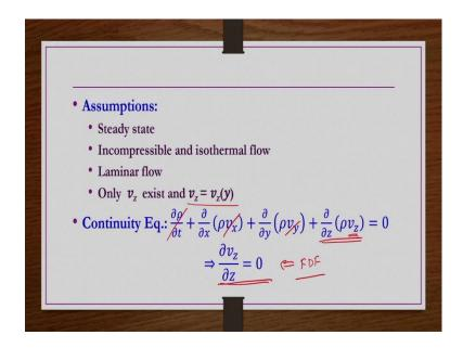
So, assumptions are the basically we are solving all these problems for steady laminar flow, incompressible fluid we are taking. And then temperature variations or the reactions mass transfer etcetera we are not taking right. And then in this geometry we have seen only  $v_z$  is existing that is function of y. Whereas, the  $v_x$  and then  $v_y$  are negligible or 0 or very small compared to the  $v_z$  that we can neglect them straightforward.
