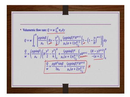
So, the volumetric flow rate  $Q = \int_0^H v_z w dy$ ; w is nothing but the width of the fluid in the x direction that we have seen in the geometry. So, this  $v_z$  expression we got this one already. And then if you integrate this one you get here for this place  $\frac{y^2}{2}$ , and then for this point you get  $\frac{y^3}{3}$  on integration. And then here this part you get y.
