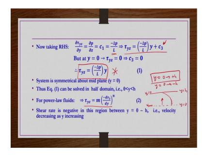
Now again  $\tau$ , now whatever the  $\frac{\partial p}{\partial z} = \frac{\partial \tau_{yz}}{\partial y}$  is there that equating to  $c_1$ . So now,  $c_1 = \frac{-\Delta p}{L}$ . That means,  $\tau_{yz}$  is nothing but  $\left(\frac{-\Delta p}{L}\right)y + c_3$ , get it on integration.
