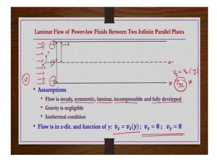
So, first we take a power-law fluid for this geometry. We are going to take Bingham plastic fluids as well. So, but whether it is power-law fluid or Bingham plastic fluids as long as the flow is the laminar symmetric one dimensional flow; then what we can have? We can
