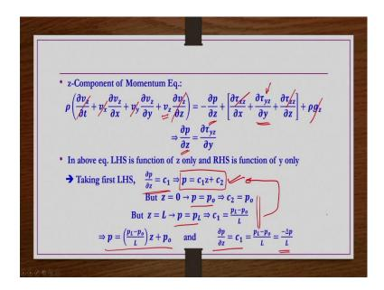
Now, z-component of momentum equation if you simplify. So, steady state term this is 0,  $v_x$  is 0,  $v_y$  is 0,  $v_z$  is existing, but it is not function of z it is function of y only. Why it is
