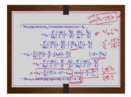
So, in the above equation that is in this equation wherever y value was there. So, we substituted  $h_p$  in the previous equation. In the  $v_z$  expression, in the  $v_z$  expression wherever y was there we are substituting  $h_p$  then we get  $v_{zp}$ . So, this is what we have.
