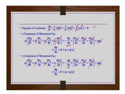
So, we are going to simplify the continuity equation right, then we are going to simplify the momentum equations. So, the geometries in Cartesian coordinates. So, the continuity equation in Cartesian coordinate is given here. So, this is the continuity equation that we have already derived in the Cartesian coordinate. So, it is an incompressible as well as steady flow.
