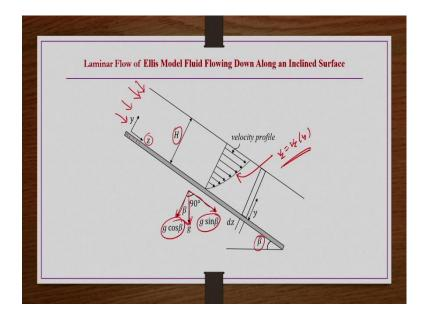
So, let us say we have an inclined surface like this. So, this is the inclined surface right. So, which is inclined to the horizontal axis at an angle  $\beta$ . So, there is a material is coming in and then flowing down here because of the gravity, right. The thickness of the material that is flowing down is hok. Inclined surface on which the material is flowing; that inclined surface flow direction we are taking z the other direction we are taking y.
