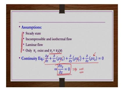
We are taking the steady state, incompressible and isothermal flow conditions, laminar flow only  $v_z$  is existing and then  $v_z$  is function of y. This material whatever is flowing down it is very thin actually. The thickness of the material is very thin, within that thin layer of the material how the velocity profile is varying? So, for such thin layer of the material that is flowing down. So, it is only one component is going to be predominant other components are going to be 0.
