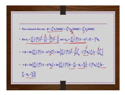
So, volumetric flow rate  $Q = \int_0^h v_z(2wdy)$  that is what we have, right from the geometry. But now  $v_z$  is having,  $v_{zp}$  between y = 0 to  $h_p$  and then  $v_z$  from between  $y = h_p$  to h. So, this  $v_{zp}$   $v_z$ ; we already got in the previous slides like this. So now, we substitute them here and then integrate.
