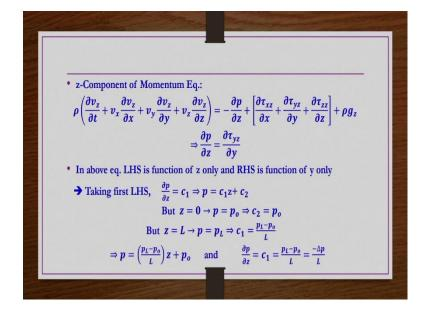
So, the simplification of z component of momentum equation is also going to be same exactly like a power-law case, because the geometry is same constraints are same; flow constraints are same. So, the pressure distribution whatever we got for the power-law case the same thing is valid here also.
