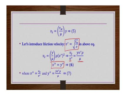
Now, this equation what we do? We try to introduce frictional velocity or we are just trying to non-dimensionalize it. Usually, velocities are being non-dimensionalized using the free stream velocities or upcoming you know inlet velocity condition whatever in general, but here the velocity profile we are developing towards the wall, towards the wall only it is not for the entire cross section area of the pipe. It is towards the wall, close to the wall only we are developing.
