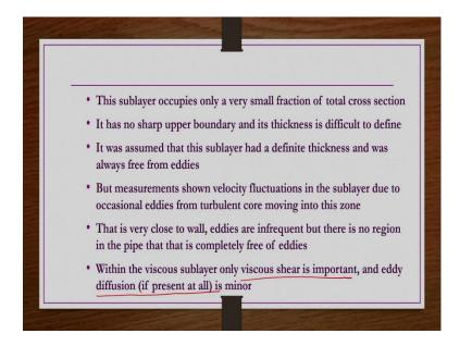
So, this sub-layer occupies obviously very small fraction of total cross section area. The  $y_L$  is very very  $y_L$  thickness,  $y_L$  whatever is there that is very small. It has no sharp upper boundary and its thickness is difficult to define in general. And then it was assumed that this sub-layer had a definite thickness and was always away from eddies at layer before having you know sophisticated advanced measurement techniques.
