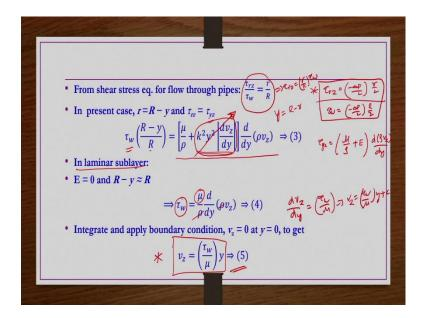
So, now shear stress equation for flow through pipes, what we have developed? When we are deriving the velocity profiles for the laminar flow through pipes, what we have developed;  $\tau_{rz}$  is nothing but  $\left(\frac{-\Delta p}{L}\right)\frac{r}{2}$  this is what we have seen. And then from here we get  $\tau_{w} = \left(\frac{-\Delta p}{L}\right)\frac{R}{2}$  this is what we have seen.
