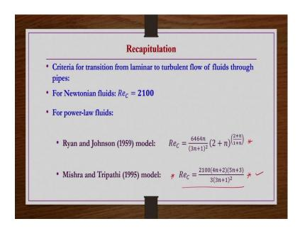
In the previous class, we have seen criteria for transition from laminar to turbulent flow of fluid through pipes. So, if the fluid is Newtonian, so then we already know that it is its critical Reynolds number for transmission of flow from laminar to turbulent is 2100. Whereas, what is that for the case of power-law fluids what is that critical Reynolds number for the case of viscoplastic fluids, etcetera, how to find out them, we have seen, right.
