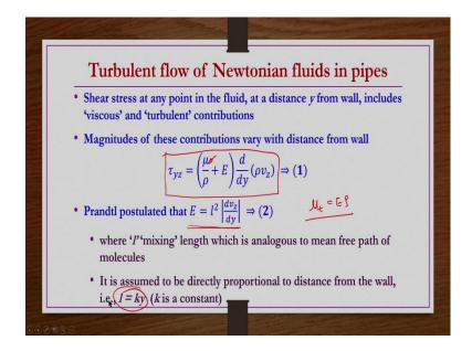
So, turbulent flow of Newtonian fluids in pipes that we take as a basis, so that it will be easy for us to move on to the power-law fluids once we have the basics of the Newtonian fluids. So; obviously, shear stress at any point in the fluid, at any distance y from the wall includes viscous and turbulent contributions because the flow is turbulent flow here. So, magnitude of these contributions vary with distance from wall. So, we need to have an expression for the shear stress.
