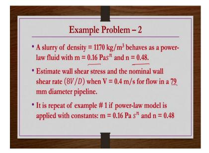
So, now we take another example problem. So, a slurry of density 1170 kg per meter cube behaves as a power-law fluid with m = 0.16 pascal second power n and n = 0.48 as its constants, right.
