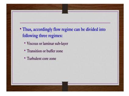
One is the laminar or viscous sub-layer which is at the wall which is close to the wall of the pipe. Another one is the turbulent region which is at the center central core of the pipe or the central most of the central core of the pipe cross section is under turbulent conditions.
