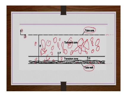
So, now, what we have? We have a pipe the tube. So, center axis of the tube is this top line. We have taken only half of the side of the tube, half cross section only we are we are taking two-dimensional and then we are out of this two-dimensional only, we are out of this 2D pictorial representation also, we are taking only lower half of the pipe.
