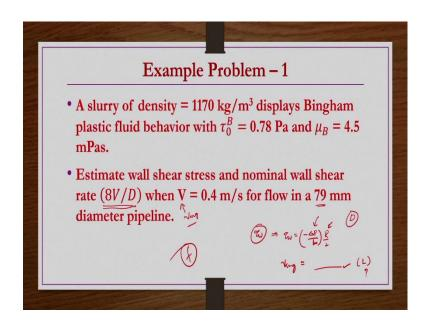
Example 1, a slurry of density 1170 kg per meter cube, this displays Bingham plastic fluid behavior with  $\tau_0^B = 0.78$  pascal and  $\mu_B = 4.5$  millipascal seconds. Estimate wall shear stress and nominal wall shear rate when V = 0.4 meter per second for flow in a 79 mm diameter pipeline.
