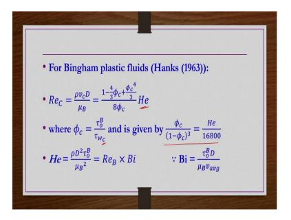
Then, coming to the viscoplastic fluids, under the category of Bingham plastic and then Herschel-Bulkley fluids we have two different models. One is the Hanks model which is for the Bingham plastic fluids, where critical Reynolds number has been reported as function of Hedstrom number and then  $\phi_c$  value.  $\phi_c$  is nothing but the  $\phi$  at critical Reynolds number, ok.  $\phi$  is nothing but  $\tau$ ,  $\frac{\tau_0}{\tau_{vv}}$  that we know, ok.
