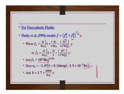
Then, we have also seen for a viscoplastic fluids how to find out the friction factor if the flow is under transitional or the turbulent flow conditions. So, Darby, what they have proposed? They have proposed friction factor, the overall friction factor is having two components that is the friction factor because of the laminar flow conditions and then because of the turbulent conditions.
