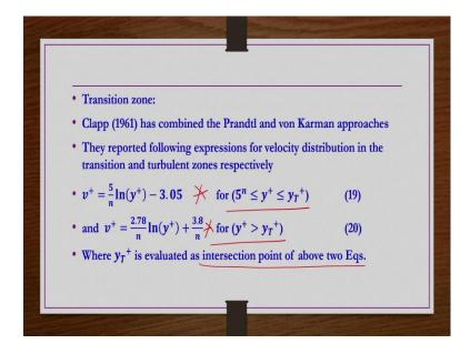
So, for the transition zone finally, the Clapp combined Prandtl and von Karman approaches, and they reported following expression for the velocity distribution for the transition and turbulent regions. This is for the transition region and this is for the turbulent region, right, where  $y_T^+$  in this equation you know you have to evaluate as intersection point of about two equations, ok. Most of them are empirical, ok.
