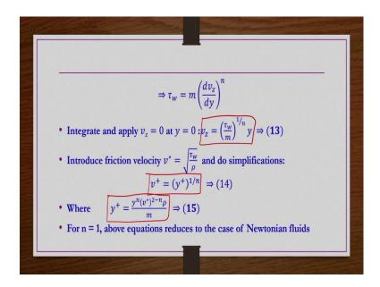
Now, again, we can do the integration and then apply the boundary condition y=0, at y=0,  $v_z=0$ , then we get  $v_z=\left(\frac{\tau_w}{m}\right)^{1/n}y$ . Now, here again if you apply frictional velocity  $v^*=\sqrt{\frac{\tau_w}{\rho}}$  in order to non-dimensionalize this above equation and then do some simplification, what you get? You get  $v^+=(y^+)^{1/n}$ .
