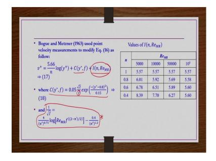
Then, Bogue and Metzner, they used velocity measurements to modify equation number 16 because velocity measurement if you are going to use directly to get the velocity profile expressions empirically, so that is going to be more reliable rather than using Q versus  $-\Delta p$  expression.
