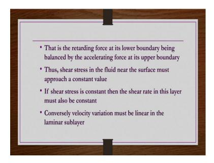
So, consequently whatever the net shear force acting on any element of fluid in this zone must be negligible, that is the retarding force at its lower boundary being balanced by the accelerating force at its upper boundary. So, thus, the shear stress in the fluid near the surface must approach a constant value. It is not one single constant value. It is very small. The change is very small.
