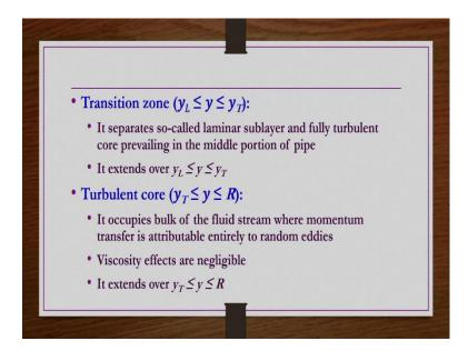
So, transition zone it extends between  $y_L$  to  $y_T$ . It separates the so called laminar sub-layer and then fully turbulent core. Whereas, the turbulent core is extend from  $y_T$  to R value that is towards the center of the axis. It occupies bulk of the fluid stream where momentum transfer is attributable entirely to random eddies. And then viscosity effects are negligible, right. So, it extends between  $y_T$  to R values.
