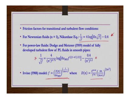
Then, friction factors also we have obtained. Friction factors for the transitional and turbulent flow conditions in smooth pipes, right. If it is Newtonian fluid then we know that Nikurdse equation for friction factor is this one, right. But what is if the fluid is power-law fluid? Then we have according to Dodge and Metzner. They have developed similar equation which is similar to the Newtonian case and then that is given by this one, right.
