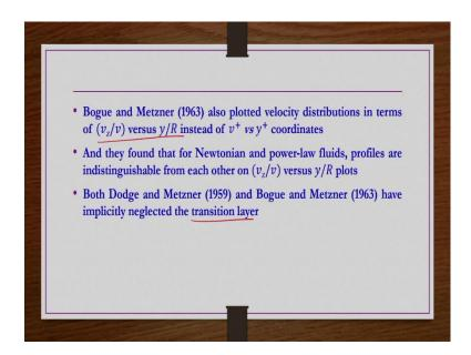
Finally, Bogue and Metzner also plotted this velocity distribution rather plotting them in terms of  $y^+$  versus, rather plotting the velocity distribution in terms of  $v^+$  versus  $y^+$  only. They have also plotted  $v_z/v$  versus y/R as well. And then, they found when they plotted  $v_z/v$  versus y/R there is no distinguishable difference between Newtonian and power-law fluid velocity profiles, ok.
