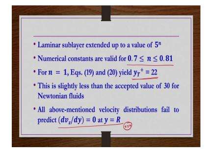
So, finally, what we understand laminar sub-layer extended up to a value of  $5^n$  according to Clapp, and then these values numerical constants whatever are provided in their analysis they are valid between narrow range of n between 0.7 to between 0.7 and 0.81, for n = 1  $y_T^+$  they are getting approximately 22. But it has to be 30, if you are comparing with the Newtonian counterparts. So, then you know slightly lesser value, ok.
