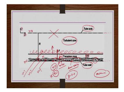
Why it is? Because, so at the tube wall what we have in general? We have a no slip condition; that means, the very first layer attached to the tube wall is having velocity 0, right. So, even the velocity at the center turbulent core is you know very high velocity, but at the wall the very first layer of the fluid attached to the wall is having 0 velocity, right. So, irrespective of what is the other velocity at the center of the pipe, ok.
