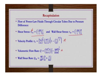
So, for the case of Power-law fluids we obtain the shear stress expression as this one  $\tau_{rz} = \left(\frac{-\Delta p}{L}\right)\frac{r}{2}$  that is shear stress linearly varying with the radial coordinate r ok. If you wanted to know the maximum shear stress that is at wall. So, then you substitute r = R in this equation then you will get  $\tau_w = \left(\frac{-\Delta p}{L}\right)\frac{R}{2}$ .
