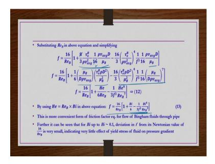
In the next step what we do? We write  $Re_B = \frac{\rho v_{avg} D}{\mu_B}$  here and then here also, then what you do? We combined these terms such a way that we have  $\frac{1}{6}$ , here because 8 1's are 8 2's are and then 3 2's are 6 we get here.
