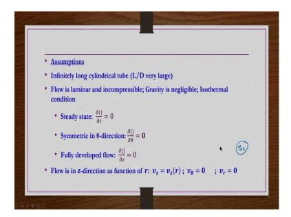
So, now assumptions for this flow also exactly same as we have done for the previous two cases. Because geometry flow nature everything is same except the rheology of the material is changing. So, we have infinitely long cylindrical tube L/D is very large so, that fully developed flow is there.
