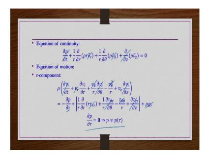
So, this term is  $0 \text{ } v_r$  is not existing,  $v_\theta$  is not existing and then fully developed flow. So,  $\frac{\partial}{\partial z}$  of any flow variable is 0. So, then continuity is maintained. Then equation of motion r component of equation of motion, it is given here. So, steady state this term is 0,  $v_r$  is 0,  $v_\theta$  is 0 symmetry.
