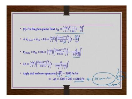
So, for the Bingham model  $v_{zp}$  we just found this expression right. So, now here  $v_{zp}$  is given as  $0.6 - \Delta p$  is not given we have to find out and then r is given or d is 40 mm. So, r is 20 mm that is given  $\mu_B$  is given as 150 milli pascal second. So, that is 0.15 pascal second and then  $\frac{R_p}{R}$  is nothing, but  $\frac{\tau_0^B}{\tau_w}$  we just have seen in the derivation right. So, that we are writing.
