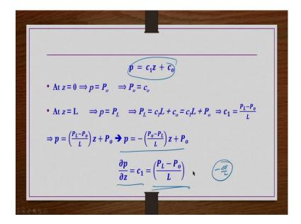
Now we apply the boundary condition at z = 0,  $p = P_0$ . So,  $c_0 = P_0$  at z = L,  $p = P_L$ . So,  $c_1$  we get  $\left(\frac{P_L - P_0}{L}\right)$ . So, when you substitute this  $c_1$  and  $c_0$  in this expression we get  $p = -\frac{\Delta P}{L}z + P_0$  where whereas,  $-\Delta P$  is nothing, but whatever this  $-P_0 - P_L$  ok.
