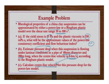
So, rheological properties of a material is given and then it has been found that either power law nature or Bingham plastic model can be you know used to represent that particular materials rheology when shear rate is between 10 to 100 second inverse. The rheological behaviour is such a way that you can use either power law model or Bingham model for that fluid if shear rate is 10 to 100 second inverse.
