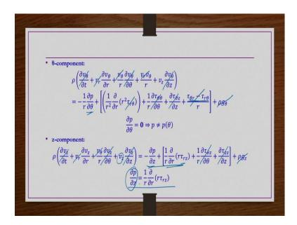
So,  $\theta$  component of momentum equation given here, here also we apply the constraints. So, steady state this term is 0,  $v_r$  is not existing,  $v_\theta$  is not existing symmetry. So, this term is 0,  $v_r v_\theta$  both are 0 and then fully developed flow. So,  $\frac{\partial}{\partial z}$  of anything is 0, pressure we cannot say we do not have any generalized boundary conditions anything.
