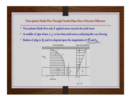
So, viscoplastic fluids through circular pipes due to pressure difference the pictorially the same thing whatever I have explained is given here ok. Viscoplastic fluids flow only for applied stress exceeds the yield stress, at middle of pipe where  $\tau_{rz}$  is less than yield stress, solid plug like core flowing between r = 0 to  $r = R_p$ .
