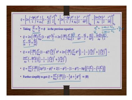
So, what we do? Now here we substitute in this case first case we substitute 0 to  $R_p$  limits, second case that is second and third terms we substitute the limits  $R_p$  to R. Then what we get? That is what we write and then further what we write? We also write  $\frac{R_p}{R}$ .  $\frac{R_p}{R}$  is nothing but  $\frac{\tau_0^B}{\tau_w}$  that we can write as  $\phi$ . Because what is  $\tau_0^B$ ?
