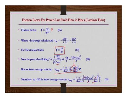
So friction factor how we can define? We can define like a dimensionalize wall shear stress that is wall shear stress non-dimensionalized using the kinetic energy  $\frac{1}{2}\rho v^2$ . Because this friction factor is essential when the fluid is under motion ok. So, this  $f = \frac{\tau_w}{\frac{1}{2}\rho v^2}$  is the definition that we can have. So, then now this f friction factor we have to find out for the case of power law fluids.
