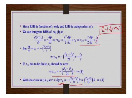
So,  $\frac{\partial p}{\partial z} = c_1 = \frac{-\Delta p}{L}$  that is what we can write. Now what we can do? Whatever the  $\frac{\partial p}{\partial z} = \frac{1}{r}\frac{\partial}{\partial r}(r\tau_{rz})$  equation was this by simplifying the z component of momentum equation. So,
