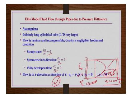
So; that means, whatever previous lecture that we have taken a circular tube infinitely long cylindrical tube right. So, that is L/D ratio is very large. So, then we have taken the only
