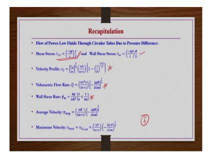
So, we have a recapitulation of that one in the previous class we have seen the flow of power law fluids through circular tubes due to pressure difference if it is taking place. So, how to obtain the velocity profile how to obtain the volumetric flow rate how to obtain the average and maximum velocity etcetera those things we have discussed right.
