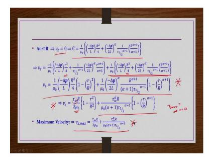
So, this c constant is this one when you substitute r = R in the previous equation then  $v_z$  will become 0 and then corresponding c is this equation. And then that c we are substituting in this  $v_z$  expression  $v_z = -\frac{1}{\mu_0} \left(\frac{-\Delta p}{L}\right) \frac{r^2}{4} + \frac{1}{\tau_{1/2}} \left(\frac{-\Delta p}{2L}\right)^{\alpha} \frac{r^{\alpha+1}}{\alpha+1} + c$  in place of c this is coming out.
