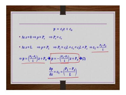
So, what are the boundary conditions? At z = 0 p = p<sub>0</sub>. So, c<sub>0</sub> should be P<sub>0</sub> and at z = L p is = P<sub>L</sub>. So, that P<sub>L</sub> = c<sub>1</sub> L + c<sub>0</sub> then c<sub>1</sub> we get  $\frac{P_L - P_0}{L}$ ; that means, p = c<sub>1</sub> is  $\frac{P_L - P_0}{L} + z + P_0$ . So, the same thing we can write  $P_L - P_0$  we can write  $\frac{-P_0 - P_L}{L}$ . So, that p =  $\frac{-\Delta p}{L} + z + P_0$ .
