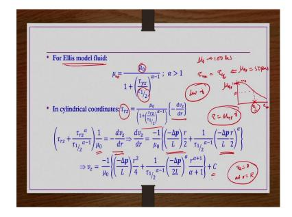
So, now after this point we are going to bring in the effect of the fluid rheology. So, for Ellis model fluid apparent viscosity is nothing but this is apparent viscosity. At the beginning itself, we have a you know made a you know generalization that if it is a non-Newtonian fluid then whether you specifically write apparent viscosity or not it is apparent viscosity because viscosity changes with shear rate ok.
