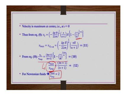
Now, anyway and that is average velocity. If you wanted to find out the maximum velocity; velocity is going to be maximum at the center of the circular pipe that we have taken. So, then we have to substitute in the velocity profile distribution r = 0 in the velocity profile distribution equation whatever we derived that is equation number 8 if you substitute r = 0 then you get maximum velocity.
