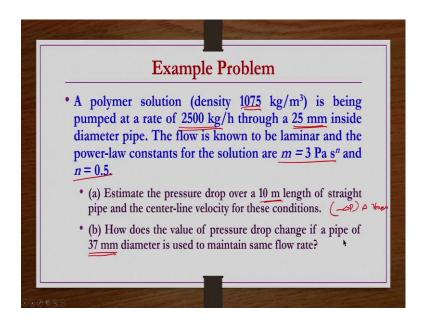
So, before winding up this class we will take a simple example problem. So, there is a polymer solution of certain density is being pumped at a certain mass rate through a pipe of certain diameter and then flow is known to be laminar and power law and the power law constant for this fluid whatever the power law fluid is there that rheology is you know represented by the power law of nature.
