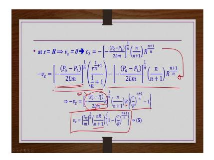
So, this is the  $c_3$ . Now, this  $c_3$  you are going to substitute in the minus  $v_z$  is equals to this particular term and then plus  $c_3$  was there in place of plus  $c_3$  this is the term that we got right.
