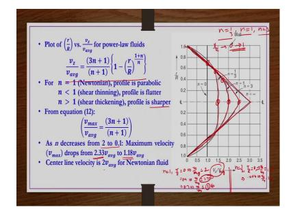
So, this is what we are taking. So, for that we are plotting  $\frac{r}{R}$  versus  $\frac{v_z}{v_{avg}}$ . So,  $\frac{v_z}{v_{avg}}$  that equation number 10 the just now we had, that is  $\frac{v_z}{v_{avg}}$  we had  $\frac{3n+1}{n+1} \left\{ 1 - \left(\frac{r}{R}\right)^{\frac{1+n}{n}} \right\}$ .
