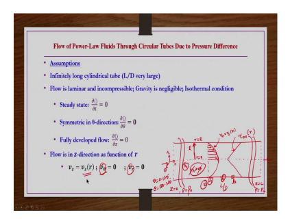
That is we have a circular tube we are having which is having a very large you know L/D ratio that is you know a length is very large compared to the diameter; compared to the diameter of the circular tube right.
