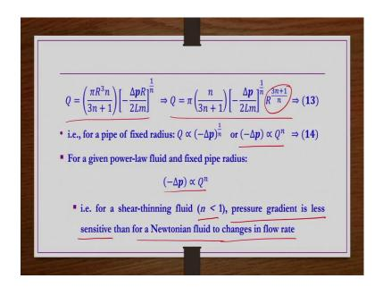
So, now we see a few more details because whatever the volumetric flow rate versus  $\Delta$  p that is important from a engineering applications point of view, that information now we are going to analyze for a power law fluids here in this case.
