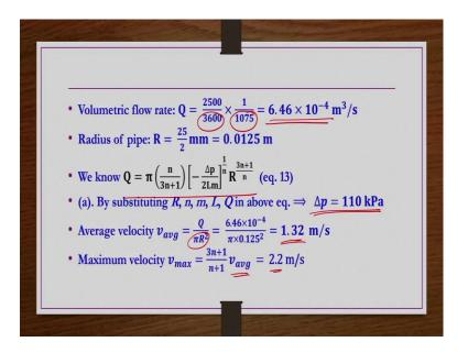
2500 kg per hour. So, per hour we have written 3600 seconds and then dividing by density 1075 kg per meter cube. So, then volumetric flow rate you get 6.46 multiplied by  $10^{-4}$  cube per second.
