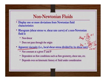
So, they display one or more deviation from Newtonian fluid characteristics as just now explained a few slides before. Then rheogram or shear stress versus shear rate curve of a non-Newtonian fluid it can be non-linear or it does not pass through the origin it is possible and then normal stress differences may not be 0 for non-Newtonian fluids.
