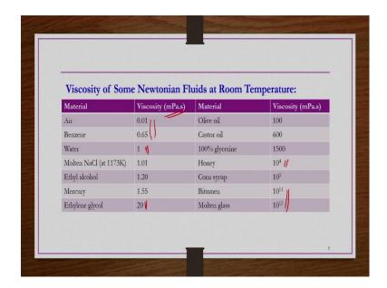
So, that is not true at all. So, if you see these examples here. See now this air, benzene, water, molten NaCl, ethyl alcohol, ethylene glycol, olive oil, honey, bitumen etcetera for all these materials viscosity is shown here, viscosity is shown here in mPa.s. You can see the material are having the viscosity as low as 0.01 mPa.s, 1 mPa.s, 20 mPa.s, 10<sup>4</sup> mPa.s, 10<sup>11</sup>, 10<sup>15</sup> mPa.s.
