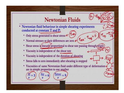
Newtonian fluid behaviour in simple shearing experiments conducted at constant temperature and pressure only stress that you find, only stress that you get in such kind of fluids is the only shear stress, only stress generated is shear stress. And then whatever the normal stresses; normal stresses are also possible because of the flow viscous flow.
