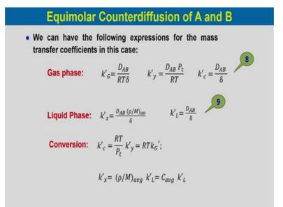
Then we can have the following expression for the mass transfer coefficient in this case. Gas phase we will get k G dash would be equal to D AB by R T into delta, k y dash would be equal to D AB P t by R T and k c dash would be D AB by delta.
