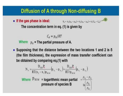
Now, if we consider the gas phase is ideal in that case, the concentration term in equation one which is this the concentration term C A we can write as p A by R T, the partial pressure of component a divided by R T. So, in that case p A is the partial pressure of component A. Now, suppose that the distance between the two locations A and 1 and 2 is delta that is the film thickness.
