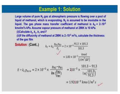
So, we can calculate capital k Y would be equal to k G p B 1 into p B 2 by P t. So, if we substitute this would be equal to 1.83 into 10 to the power minus 3 kilomole per metre square second into the driving force delta Y. F is equal to k G P BLM. So, if we substitute we can calculate P BLM and then if we substitute over here it would be equal to 2 into 10 to the power minus 5 and it is 1.92 into 10 to the power minus 3 kilomole per metre square second.
