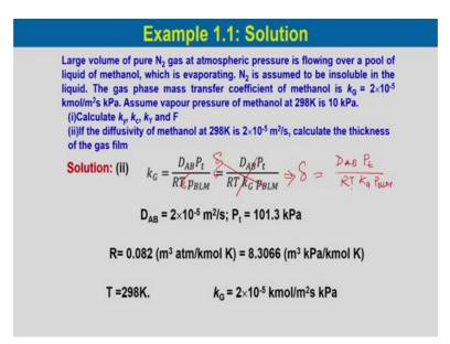
So, F is calculated and we need to calculate the thickness of the gas film for k G as we know it is D AB P t by R T delta, delta is missing over here delta and from here we can write, if we rearrange delta would be equal to D AB P t by R T k G p BLM.
