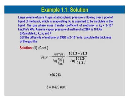
P BLM as we have soon earlier p BLM we can calculate for in this case it is 96.213. So, we can calculate delta using the earlier equations which is equal to 0.425 millimetre.
