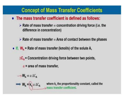
The mass transfer coefficient is defined as the rate of mass transfer as we know is proportional to the concentration driving force that is the difference in concentration and also the rate of mass transfer is proportional to the area of contact between the phases.
