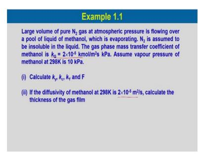
Now, let us take an example large volume of pure nitrogen gas at atmospheric pressure is flowing over a pool of liquid of methanol, which is evaporating. Nitrogen is assumed to be insoluble in liquid. The gas phase mass transfer coefficient of methanol which is given k G is 2 into 10 to the power minus 5 kilomole per metre square second kilopascal.
