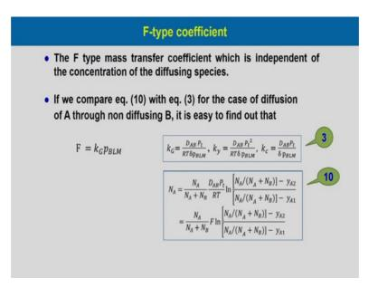
The F type mass transfer coefficient which is independent of the concentration of the diffusing species and if we compare equation 10 with equation 3 for the case of diffusion of A through non diffusing B, it is very easy to find out F is equal to k G p BLM and this is the equation 3 and 10. So, we can from there if we compare we can write F would be equal to k G p BLM.
