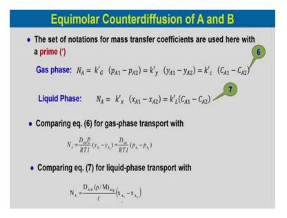
Now, the set of notations for mass transfer coefficient used in case of equimolar counter diffusion of a and b. So, if we considered equimolar counter diffusion here we have defined the mass transfer coefficient with a sign of prime. So, like in gas phase, we can write N A would be equal to k G dash into the partial pressure driving force p A 1 minus p A 2 which is equal to k y dash into the mole fractions driving force that is y A 1 minus
