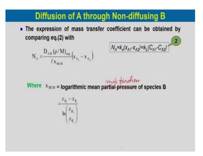
So, the expression of mass transfer coefficient can be obtained by comparing equation 2 with this equation; equation 2 in the liquid phase with the other equation in case of the diffusion that is N A would be equal to D AB rho by M average divided by 1 x BLM into x A 1 minus X A 2. In this case x BLM it would be logarithmic mean of mole fraction of component B not partial pressure mole fraction of species B which is x B 2 minus x B 1 divided by ln x B 2 by x B 1.
