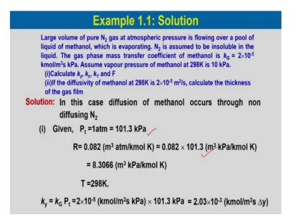
Now, in this case the diffusion of methanol occurs through non diffusing nitrogen. So, the first thing it is given that the pure nitrogen is diffusing at atmospheric pressure. So, the total pressure P t is 1 atmosphere which is 101.3 kilopascal. Now, R is known to us is 0.082 metre cube atmosphere per kilomole Kelvin which is we can write in terms of the metre cube kilopascal kilomole Kelvin in this unit.
