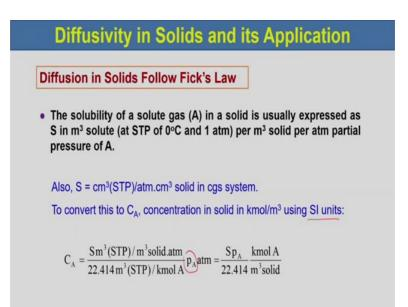
So, the solubility term of a solid gas A in a solid is usually expressed as S in metre cube solute at STP of 0 degree centigrade and 1 atmosphere pressure per metre cube of solid per atmosphere partial pressure of A.
