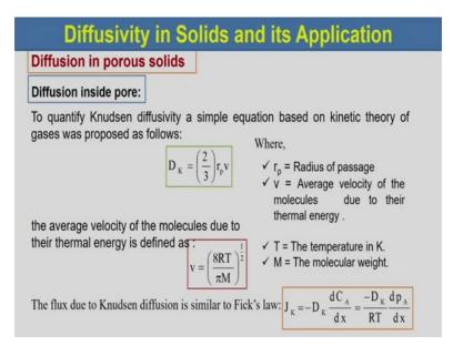
Now, to quantify Knudsen diffusivity, a simple equation based on kinetic theory of gases was proposed as follows. That is D K would be equal to 2 by 3 into r p into v where r p is the radius of the passage and v this the average velocity of the molecules due to their thermal energy.
