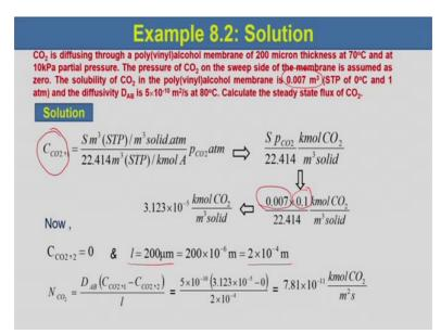
So, we can write C carbon dioxide that is concentration of carbon dioxide at side 1 is equal to S metre cube STP by metre cube solid into atmosphere divided by 22.414 metre cube STP per kilo mole A into p CO 2 atmosphere.
