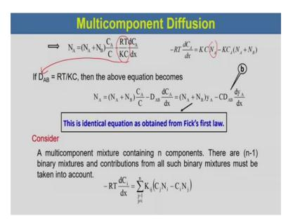
So, from this now if we rearrange we can write flux N A this one would be equal to N A plus N B into C A by C minus R T by K C into d C A d x. Now if we consider D AB would be equal to R T by K C then this equation we can write. So, this part is D AB. So, then we can write N A would be equal to N A plus N B, C A by C minus D AB D C A D x which would be equal to N A plus N B C A by C each.
