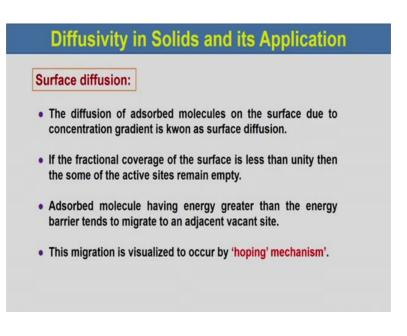
Now, another thing is the surface diffusion. The diffusion of adsorbed molecules on the surface due to concentration gradient is known as the surface diffusion.
