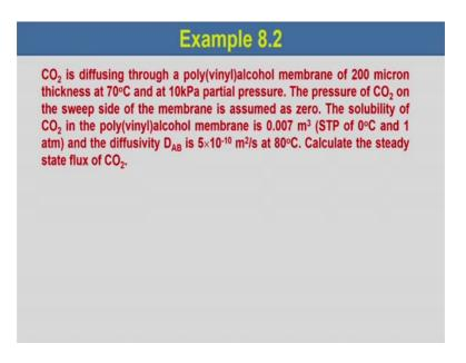
Now, let us consider another example, carbon dioxide is defusing through a polyvinyl alcohol membrane of 200 micron thickness at 70 degree centigrade and at 10 kilo Pascal partial pressure.
