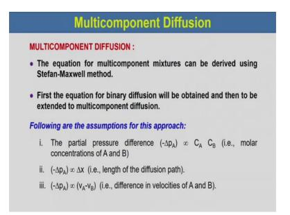
Multi component diffusion: in this case the equation for multi component mixture can be derived using Stefan Maxwell method. First the equation for binary diffusion will be obtained and then to be extended to the multi component diffusion.
