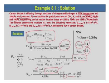
So, the flux equation which we have derived is for carbon dioxide over here is N CO 2 would be equal to C into DCO 2 mixture divided by 1 into 1 n 1 minus Y CO 2 at 1 divided by one minus Y CO 2 at 0. Now, if we consider ideal gas then C would be equal to P t by R T the system is at atmospheric pressure 100 kilo Pascal.
