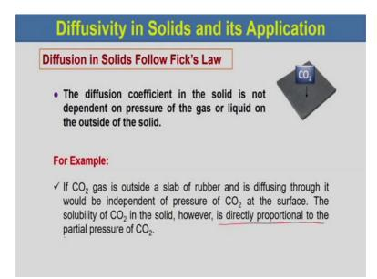
Now, diffusion in solid follow Fick's law. The diffusion coefficient in the solid is not dependent on pressure of the gas or liquid on the outside of the solid. For example, if
