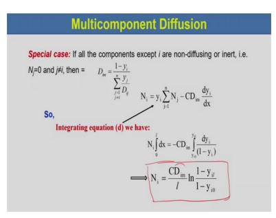
Now, if we considered a special case, if all the components except i are non-diffusing or inert. So, only i is diffusing species or other components are non diffusing or inert that is N j would be equal to 0 and j not equal to i, then D i m would be equal to 1 minus y i divided by summation over j is equal to 1 j not equal to i to n y j by D i j. So, integrating equation d we have this is equation d N i is equal to y i summation over j is equal to 1 to n N j minus C D i m d y i by d x.
