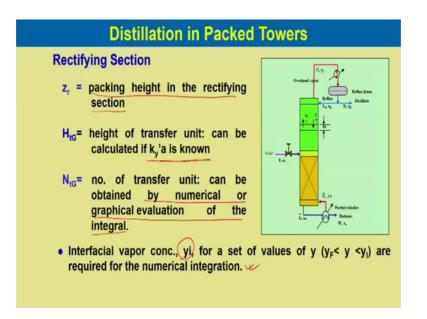
Now, z r is the packing height in the rectifying section and H tG is the height of the transfer unit and can be calculated if k y dash a is known. N tG is the number of transfer unit and can be obtained by numerical or graphical evaluation of the integral. Interfacial vapour composition that is yi as we have done before in case of absorption, for a set of values of y y F less than y less than y 1 are required for the numerical integration.
