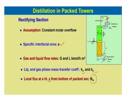
Now, we have two sections above the feed locations is the rectifying sections and below the feed location is the stripping section. Now assumptions over here is constant molal overflow and specific interfacial area is a. So, unit of a is meter square per meter cube of packing, gas and liquid flow rate G and L in kilo mole per hour meters cube, liquid and gas phase mass transfer coefficient k x dash and k y dash. Now local flux at height z from bottom of the packed section we can define by N A.
