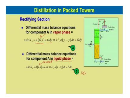
Now if we do the differential mass balance equation for component A in the vapour phase we can write a into dz into N A would be equal to d G y which is equal to G into dy which is equal to k y dash a into y i minus y into dz which is equal to G dy. So, since G is constant as we have considered constant molar overflow. So, this we can write G into d y, k y dash a is the individual mass transfer coefficient in the gas phase.
