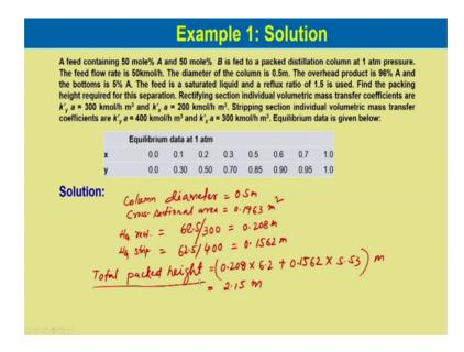
Now H G in the rectifying section is equal to 62.5 divided by 300 which is about 0.208 meter and stripping section height of transfer unit in the stripping section is about 62.5 divided by 400 so which is about 0.1562 meter.
