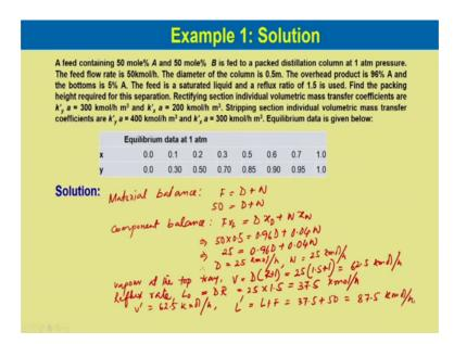
Now let us do the material balance. Overall material balance is F is equal to D plus W F is given 50 which is equal to D plus W. Now component balance on A it would be F x F would be equal to D x D plus W x W. Now if we put F this 50 into 0.5 would be equal to 0.96 D plus 0.04 W. So, from here we can write 25 would be equal to 0.96 D plus 0.04 W.
