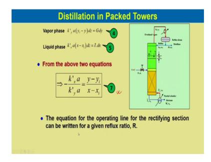
Now, vapour phase equations 4 as we have obtained k y dash a y i minus y into dz is equal to G into dy, liquid phase equations we have obtained k x dash a x minus x i dz is
