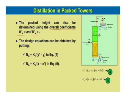
The packed height can also be determined using the overall coefficient that is capital K x a dash and capital K y dash a. The design equations can be obtained by putting N A is equal to K y dash into y star minus y in equation 4 and N A is equal to K x dash x minus x star in equation 5.
