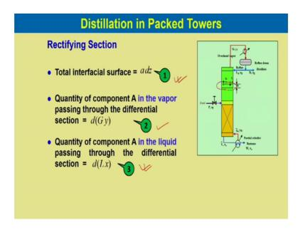
So, now the total interfacial surface would be a into dz. So, if we consider a differential area dz differential sections dz the total interfacial surface would be a into dz which is shown in equation 1. Now quantity of component a in the vapour passing through the differential sections this sections dz would be d G y which is shown in equation 2. Now quantity of component A in the liquid passing through the differential section should be d L into x so which is shown in equation 3.
