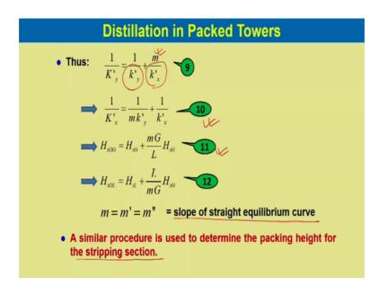
Thus 1 by K y capital K y dash would be equal to 1 by k y dash plus equal to 1 by small k y dash plus m by small k x dash here capital K y dash is the overall gas phase mass
