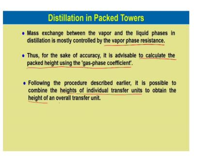
Now mass exchange between the vapour and the liquid phases in distillation is mostly controlled by the vapour phase resistance. Thus, for the sake of accuracy it is advisable to calculate the packed height using gas phase coefficient. Following the procedure described earlier it is possible to combine the height of individual transfer unit to obtain the height of an overall transfer unit.
