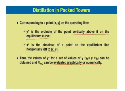
Corresponding to a point x, y on the operating line we can obtain y star is the ordinate of the point vertically above it on the equilibrium curve and x star is the abscissa of a point on the equilibrium line horizontally left to x, y. Thus the values of y star for a set of values of y which is y F less than y less than y i can be obtained and N tOG can be evaluated graphically or numerically.
