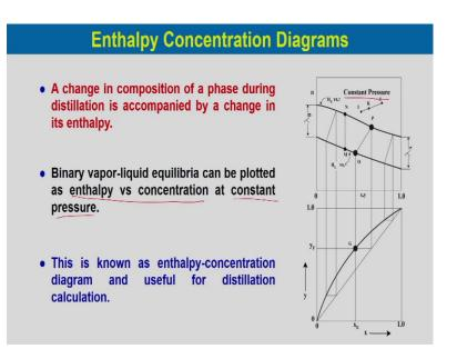
A change in composition of a phase during distillation is accompanied by a change in enthalpy. So, binary vapour liquid equilibria can be plotted as enthalpy versus concentration at constant pressure. So, this is a enthalpy concentration diagram at constant pressure. And that is why it is known as enthalpy concentration diagram and it is no very much useful for the distillation calculation.
