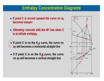
So, instead of this curve chord you will get a straight line. If the points C is moved upward the curve on x y becomes steeper. So, as you take it off upward direction as long as possible slope of the curve would become steeper and ultimately it will coincide with the 45 degree diagonal. So, when this point C would be taken to the infinite enthalpy. If point C is on the H v y curve the curve on the x y will become a horizontal straight line.
