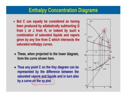
But this C can equally be considered as having been produced by adiabatically subtracting G this any point G from I and we would obtain this point C or it can be also considered adiabatically removing J from K and we would obtain the composition C. So,
