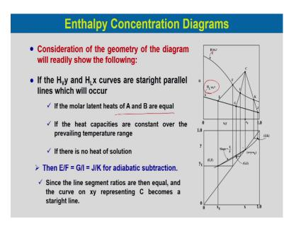
Now, if we considered the geometry of this diagram, which would readily show the following if the H v y and H L x curves are straight parallel lines which would occur when the molar latent heat of A and B are equal. So, this two curves this is H v y or H G y and H L x curves would be straight parallel line and if the molar latent heats of A and B are equal if the heat capacities are constant over the prevailing temperature range.
