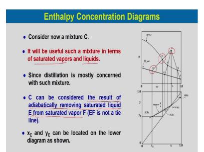
Now, if we consider another mixture say C over here. It will be useful such a mixture in terms of saturated vapours and liquid. Since distillation is mostly concerned with such mixture. So, it would be very much useful in terms of the saturated vapour or saturated liquid the mixture of that if the C point we can consider that way. C can be considered the result of adiabatically removing saturated liquid E from saturated vapour F.
