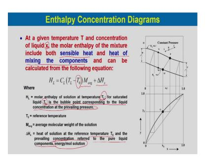
Now, at a given temperature T and concentration of liquid x, the molar enthalpy of the mixture will include the sensible heat and the heat of mixing of the components. So, any
