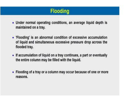
Now, we will discuss flooding. So, under normal operating condition an average liquid depth is maintained on a tray the flooding is an abnormal conditions of excessive accumulation of the liquid and simultaneous excessive pressure drop across the flooded tray.
