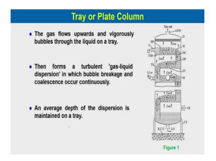
The gas flows upward and vigorously bubbles through the liquid on a tray. So, through the perforation the gas goes up and then, there is intimate contact in each tray between the gas and liquid, then forms a turbulent gas liquid dispersion in which bubble brakes and coalescence occurs continuously.
