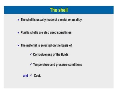
The shell is usually made of metals or an alloy ah. The materials of construction anyway we learn in another know course or another subjects. So, here we will mostly just highlight what are the materials used, plastic shells are also used sometimes. The material is selected on the basis of corrosiveness off the fluids temperature and pressure conditions and the cost.
