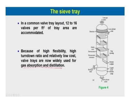
In a common valve tray layout 12 to 16 valves per square feet of tray area are accommodated and because of high flexibility high turn down ratio and relatively low cost valve trays are now widely used for gas absorption and distillation. So, these kind of trays are now widely used.
