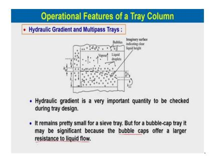
Hydraulic gradient is also very important quantity to be checked the tray design it remains pretty small for a sieve tray, but for a bubble cap tray it may be significant because the bubble caps offer a larger resistance to liquid flow. So, if the resistance is much higher in case of bubble cap tray. So, hydraulic gradient is also important over here, so, because that will severely affect the tower performance.
