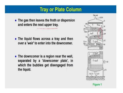
The gas then leaves the froth or the dispersion and enters the next upper tray. The liquid flows across a tray and then, over a weir to enter into the down comer. The down comer is a region near the wall separated by a down comer plate. You can see over here down comer plate in which the bubble get disengaged from the liquid.
