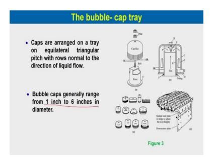
Caps are arranged on a tray on equilateral triangular pitch with row normal to the direction of the liquid flow. Bubble caps generally range from 1 inch to 6 inches in diameter.
