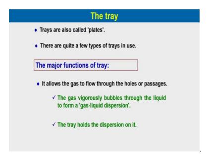
Trays are also called plates. So, either we can call it tray columns or plate columns. There are quite a few types of trays in use. Major function of tray is basically it allows the gas to flow through the holes or passages. So, the tray will allow the gas to pass through the holes on the tray. The gas vigorously bubbles through the liquid to form a gas liquid dispersion.
