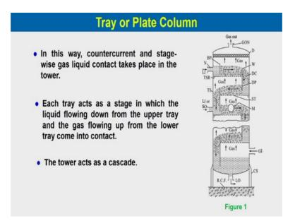
In this way counter current and stagewise gas liquid contact takes place in the tower. Each tray acts as a stage in which the liquid flowing down from the upper tray and the gas flowing up from the lower tray come in contact ok. The tower acts as a cascade because you have multiple tray and the vapour and liquid flows from tray to tray.
