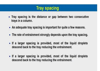
Now, the tray spacing; tray spacing is the distance or gap between the consecutive tray in a column. An accurate tray spacing is important for quite a few reasons.
