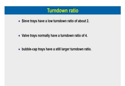
So, turndown ratio for sieve trays have a very low turndown ratio of about 2 for sieve trays, for valve trays normally have a turndown ratio of 4 and bubble cap tray have a still larger turndown ratio.
