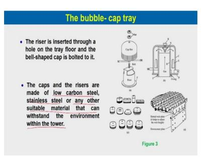
The riser is inserted through a hole on the tray floor and the bell shaped cap is moulded to it. Now, the cap and the riser are made of low carbon steel. So, here its materials of construction usually is low carbon steel or stainless steel or any other suitable materials that can withstand the environment within the tower. So, depending on the application the materials maybe changed.
