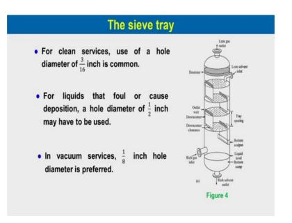
For clean services we use of hole diameter of 3 by 16 inch is common, very common 3 by 16 inch. For liquid that foul or cause deposition hole diameter of half inch maybe may have to be used. So, if the liquid which will know may clot or foul the tray holes, then in that case the larger size holes may be used in vacuum services one-eighth inch hole diameter is preferred.
