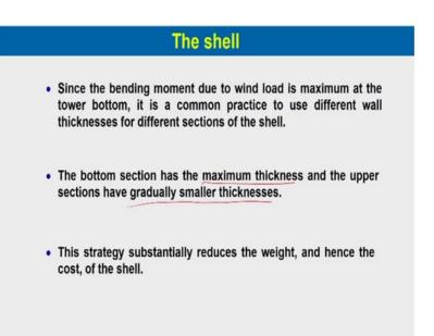
Since the bending moment due to wind load is maximum at the tower bottom, it is a common practice to use different wall thickness for different sections of the shell. So, depending on the bending moment or due to the wind load and several other accepts the thickness of the sections or of the wall, of the tower maybe different.
