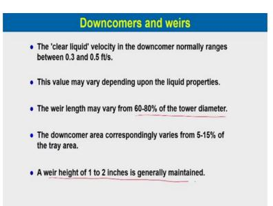
The clear liquid velocity in the down comer normally ranges between 0.3 to 0.5 feet per second. This value may vary depending upon the liquid properties. The weir length may vary from 60 to 80 percent of the tower diameter. So, as we said the tower diameter is generally upto say 10 metre in case of the industrial towers.
