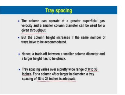
The column can operate at a greater superficial gas velocity and a smaller column diameter can be used for a given throughput, but the column height increases if the same number of tray have been accommodated. Hence a trade off between a smaller column diameter and a larger height has to be struck.
