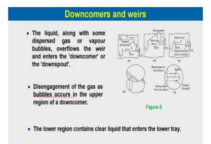
The liquid along with some dispersed gas or vapour bubbles overflows the weir and enters the down comer or the downspout. So, what happens when the liquid entered into a tray, it flows horizontally and then, you have a vertical movement of the gas through the perforation.
