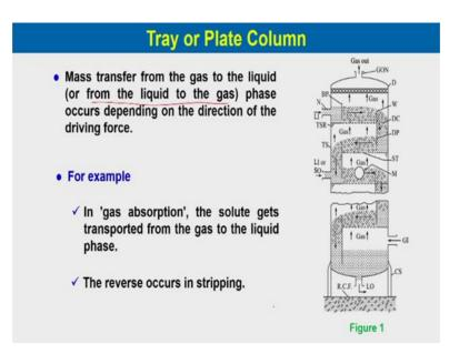
Mass transfer from the gas to the liquid phase or from the liquid to the gas phase occurs depending on the direction of the driving force. So, both the way it is possible for absorption; the solute from the gas mixtures transfer from the gas phase to the liquid phase whereas, for striping or desorption solute from the liquid phase transferred to the gas phase.
