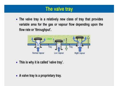
Now, we will discuss the valve tray. The valve tray is a relatively new class of tray that provides variable area for the gas and vapour floor depending upon the flow rate or throughput you can see over here there is a normal vapour which is coming to this and then, you have a tray, then there is a particular height of liquid it maintains. When vapour flow rate is low, opening is less. When vapour flow rate is more, opening is more. Then this is why it is called a valve tray.
