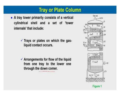
A tray tower primarily consist of a vertical cylindrical shell and a set of tower internals. This tower internal includes tray or plates on which the gas liquid contact occurs. So, for each plate or tray the gas and liquid comes in intimate contact arrangement for flow of liquid from one tray to the lower one through the down comer. So, through down comer the liquid which is know from the inlet, it goes to the down comer and it comes down to the next plate.
