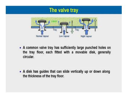
A valve tray is preparatory tray and a common valve tray has sufficiently large punched holes on the tray floor each fitted with a movable disk. Generally circular disk a disk has guides that can slide vertically up or down along the thickness of the tray floors.
