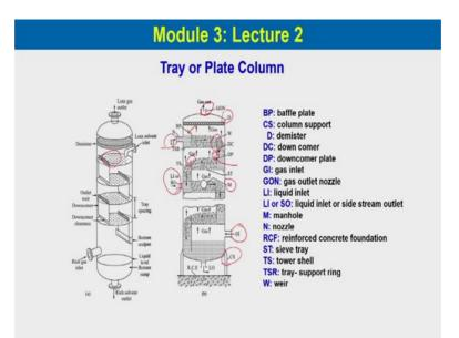
So, let us start with our tray or packed column. You can see the this is a typical look of tray column as you can see in this column you have the different terms used over here already written over here BP represents the baffle, baffle plate over here and we have column support which is over here, then we have demister which is over here and then down comer DC is over here where the liquid comes down. We will discuss more about it down comer, then down comer plate.
