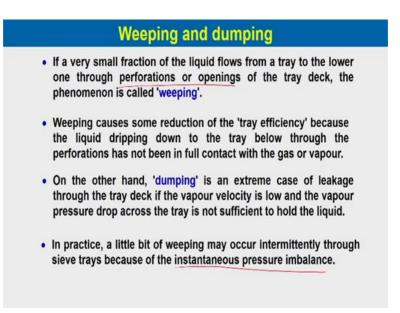
Weeping and dumping if a very small know fractions of the liquid flows from a tray to the lower one through perforation or opening of the tray deck the phenomenon is called weeping.
