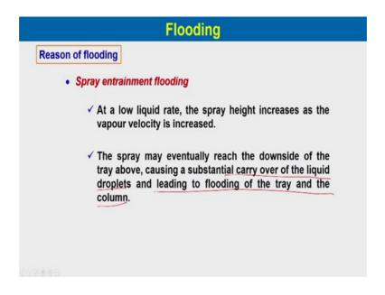
So, one of them is spray entrainment flooding. So, at a very low liquid rate as we said when you have a very low liquid rate, the spray height increases as the vapour velocity is increased. The spray may eventually reach the downside of the tray above causing a substantial carryover of the liquid droplets and leading to the flooding of the tray and the column.
