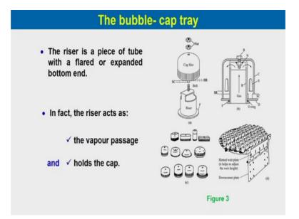
The riser is a piece of tube with a flared or expanded bottom end, so, you can see here. So, the bottom is a little expanded are flared. It is a know tube like arrangements and then the riser acts as the vapour passage and holds the cap. So, this riser when you put you know cap over here when there is a flow from the bottom, so cap will go up and the opening from the riser will also go up. So, the vapour will go out. It controls the vapour passage and it also holds the know cap over it.
