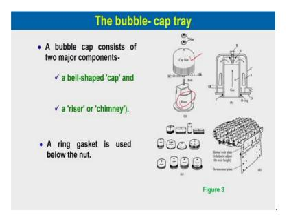
There are different kind of trays and now we will discuss on the bubble cap tray. The bubble cap tray consist of two major components. One is know cap slot a bell shaped cap
