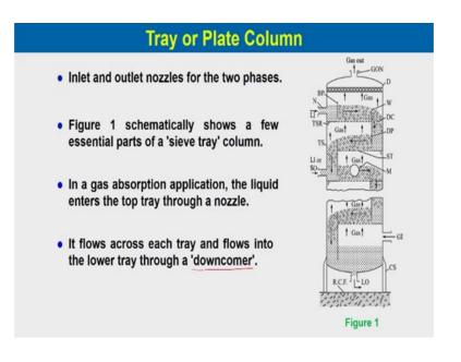
Inlet and outlet nozzles for the two phases nozzles are provided for the two phases. For the two phases the figure 1 which you can see over here schematically such a few essential part of a sieve tray columns in gas absorption application, the liquid enters at the top tray through a nozzle. Here it flows across each tray and flows into the lower tray through a down comer as we have discussed before.
