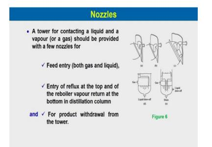
Now, nozzles a tower for contacting a liquid and a vapour or a gas should be provided with a few nozzles for feed entry both gas and liquid and then entry of reflux at the top and the reboiler vapour return to the bottom in a distillation column. So, and also for product withdrawal from the tower, so, for this places we need to have a nozzle at different locations.
