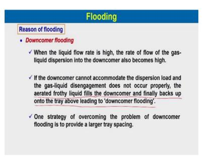
Another is the down comer flooding. So, when the liquid flow rate is high the rate of flow of the gas and liquid dispersion into the down comer also becomes high. So, because of high gas flow rate there will be know vigorous mixing in a particular column and there will be large number of bubbles and which will be carried by the liquid towards the down comer.
