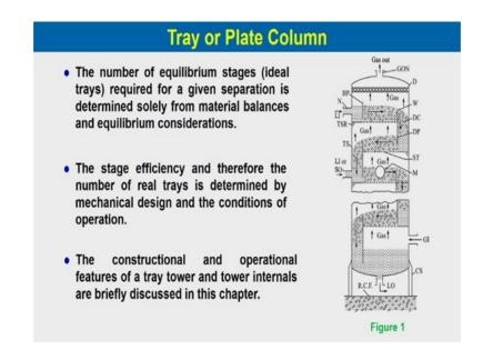
So, it acts as a cascade. The number of equilibrium stages or we call it ideal stages or trays required for a given separation is determined solely from the material balance and equilibrium consideration, the stage efficiency and therefore, the number of real trays is determined by mechanical design and the conditions of operation. The construction and the operational feature of a tray tower and the tower internals are briefly discussed in this on lecture.
