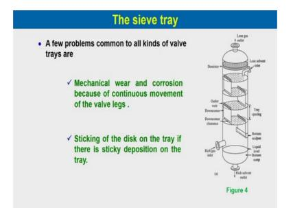
And there are few problems in case of sieve tray we usually encountered so which is also happens not only valve tray, but there are also for different sieve trays as well mechanical wear and corrosion because of continuous movement of the valve legs and sticking of the disk on the tray, if there is a sticky deposition on the tray. So, sometimes because of this there is a sticking of the disk, it may malfunction the know valve tray. (Refer Slide Time: 20:59)
