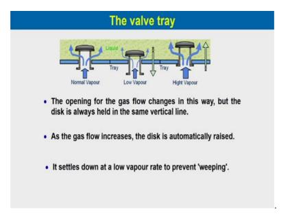
The opening for the gas liquid changes in this way, but the disk is always held in the same vertical line. As the gas flow increases, the disk automatically rises. It settle down at low vapour rate at know to prevent weeping. Weeping means the liquid drops which
