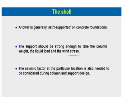
A tower is generally skirt-supported on concrete foundation. As you have shown you on the figure there is skirt-foundation or support which is made of concrete. So, to keep the tower the support should be strong enough to take the column weight, the liquid load and the wind stress. Generally the columns are very tall close to 50 metre in the height. The seismic factor at the particular location is also needed to be considered during column and support design.
