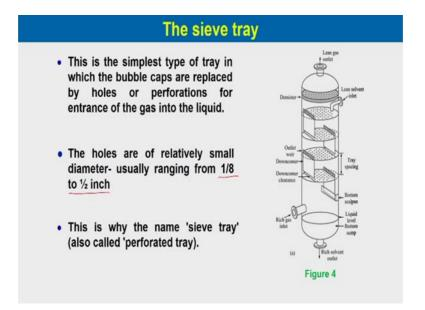
Now, we will discuss about the sieve tray. In this figure you can see this is the simplest type of tray in which the bubbles caps are replaced by holes or perforations for entrance of the gas into the liquid.
