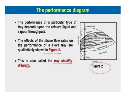
Now, let us see the performance diagram ah. Here you can see the know how the column can perform under different vapour rate and the liquid rate. The performance of a particular type of tray depends upon the relative liquid and the vapour throughput. The effects of the phase flow rate on the performance of a sieve tray are qualitatively shown in this figure over here figure 2. This is also called a tray stability diagram.
