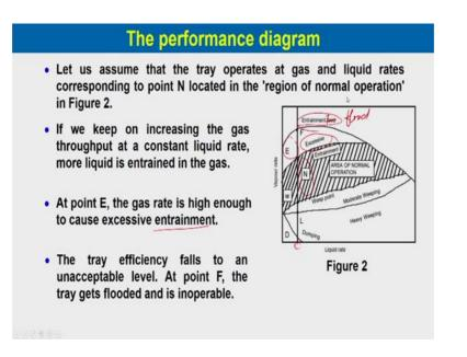
Now, let us assume that the tray operates at gas and liquid rates corresponding to point N. So, at this location in the region of normal operations, so we call it normal operation
