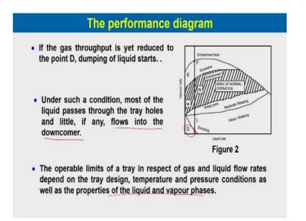
If the gas throughput is yet reduced to point D, dumping of liquid starts, ok. So, in this region so dumping will start. Under such a condition most of the liquid passes through the tray holes and little if any flows into the down comers. So, all the liquids which will come from the top tray will pass through the perforation and it will fall down directly without any flows or little flows through the down comer.
