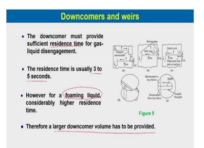
The down comers must provide sufficient residence time for gas liquid disengagement, so that the clear liquid will come to the next stage. The residence time is usually 3 to 5 seconds; however for a forming liquid considerably higher residence time is there.
