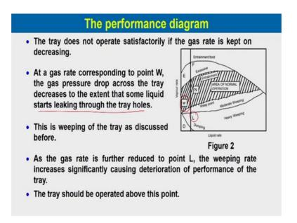
The tray does not operate satisfactorily if the gas rate is kept on decreasing. Now, if we also decrease the gas rate what happens let us see. At a gas rate corresponding to point W over here, the gas pressure drop across the tray decreases to the extent that some liquid start leaking through the tray holes. If that is happens, then we have a weeping. This weeping of the tray as discussed before will happen as the gas rate is further reduced to point L over here.
