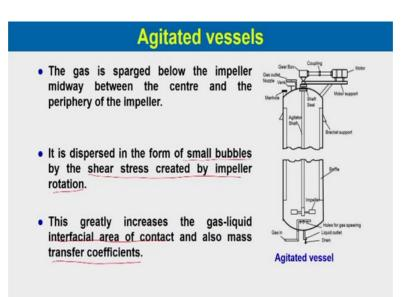
The gas is sparged below the impeller midway between the centre and the periphery of the impeller. So, the liquid which is coming over here which is kept inside the container and then gas is passed through it.
