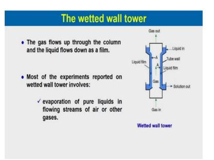
The gas flows up through the column and the liquid flows down as a film, most of the experiments reported on the wetted wall tower involves evaporation of the pure liquid in flowing streams of the air or other gases.
