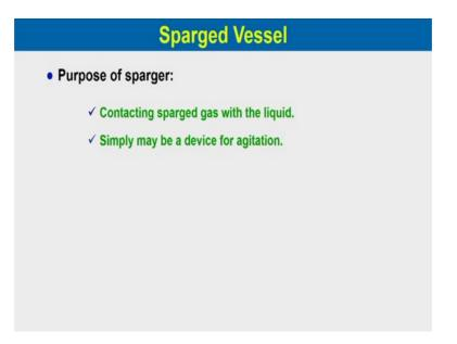
Purpose of the sparger it is no well known fact that we need to have a good contact between the gas and liquid phase. So, contacting sparged gas with the liquid that is the purpose of the sparger sparger and simply it may be used a device for agitation. So, agitations simply help or not only to increase the no surface area, but also improve the mass transfer rate and also the heat transfer rate. So, to do that these are the no major purpose for the use of sparger.
