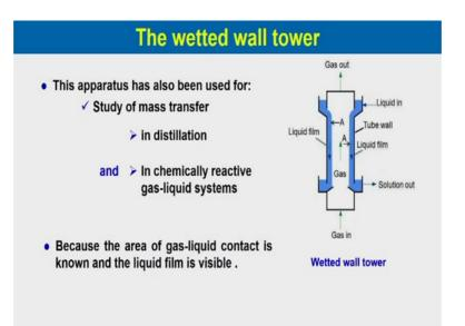
The apparatus has also been used for study of mass transfer in distillation and also in chemically reactive gas liquid systems. So, because the area of gas liquid contact is known and the liquid film is visible. So, you can see the liquid film and you can do the your study whether there is ripple formation, if you wanted to run in the no in the laminar region.
