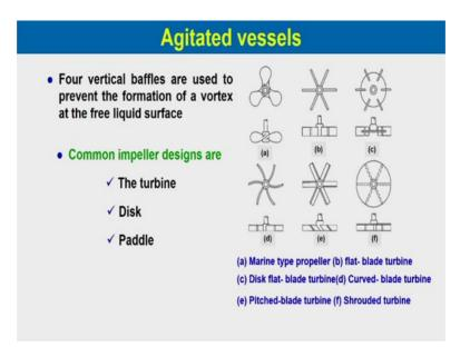
Now, in this case as we have said there are different types of impeller design, you can see four vertical baffles are used to prevent the formation of the vortex at the free liquid surface, you have seen the no baffles which are used now the you can see over here the common impeller design which are given over here. So, one is marine type propeller a, then flat blade turbine, disk flat blade turbine, curved blade turbine, pitched blade turbine and shrouded turbine.
