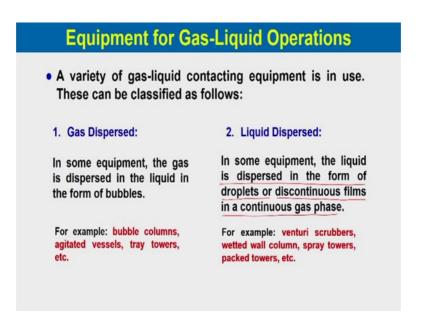
A variety of gas liquid contacting equipment is in use, this can be classified as follows. One is gas dispersed: in some equipment the gas is dispersed in the liquid in the form of bubbles like, bubble columns, agitated vessels, tray towers in this case liquid flows through the column, but gas is bubbled through the liquid. So, it is called the gas dispersed.
