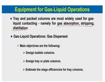
Tray and packed columns are most widely used for gas liquid contacting namely for gas absorption, stripping and distillation. So, for this three applications tray or plate columns and packed columns are widely used. Gas liquid operation: so, gas dispersed the main objective are the following: here the design of bubble column design of tray or plate columns and estimate the stage efficiency for tray columns.
