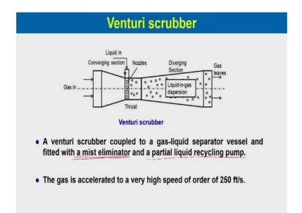
A venturi scrubber coupled to a gas liquid separator vessel and fitted with the mist eliminator and a partial liquid recycling pump. So, what happens no after the gas liquid intimate contact happens or mass transfer happened there will be a separator we need where, you need to separate the no the between the two phases. And also you need to have a mist eliminator after that and then a partial liquid which will be no come can be recycled back.
