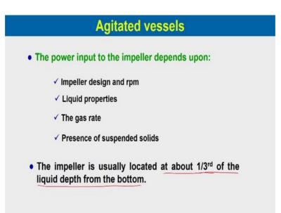
The power input to the impeller depends upon the following factors, one is impeller design and rpm; then liquid properties liquid mainly viscosity density of the liquids will depend on the no the power required for the impeller. Then the gas rate, presence of suspended solids the impeller is usually located at about one third of the liquid depth from the bottom. So, this is a typical design a one-third of the liquid depth from the bottom of the agitator.
