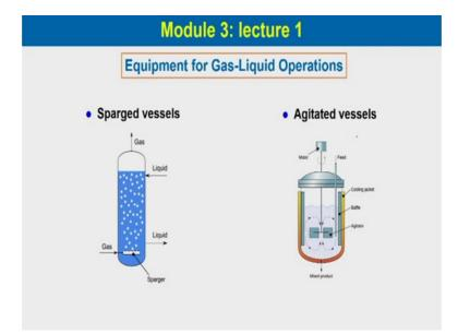
In lecture 1, we will show you different batch and the continuous mode of contact equipments which are used for this gas liquid systems, one of them is sparged vessels. So, you can see in this case the gas enters at the bottom and liquid enter at the top and there is an intimate contact enter inside the column so that the mass transfer happens from either from the gas phase to the liquid phase or from the liquid to the gas phase.
