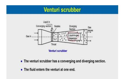
Now, another is venturi scrubber as we have no introduced at the beginning, the there is a gas inlet in the converging section and then there is a throat of the nozzle and where the liquid enters through the nozzles and then there is an intimate contact in the diverging section the gas liquid dispersion. Liquid in gas dispersion; the venturi scrubber has a converging and diverging section the fluids enters the venturi at one end.
