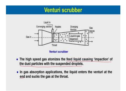
The high speed gas atomizes the feed liquid causing the impaction of the dust particles with the suspended droplets. So, if you have a dust particles, it will cause infections of the dust particles with the suspended droplets.
