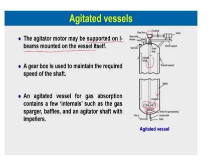
The agitator motor may be supported on ibeams mounted on the vessel itself. So, you can see it has to be no mounted somewhere or supported with ibeams mounted on the vessel itself. And then a gearbox is used to maintain the required space of the shaft over here which is already discussed, then an agitated vessel for gas absorption contains a few internals such as the gas sparger baffles and an agitator shaft with impeller.
