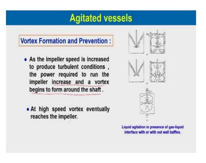
Vortex formation and prevention? So, you can see if you have only impeller there will be vortex formation and there will not be very good no agitation inside the liquid. So, as the impeller speed is increased to produce turbulence turbulent conditions the power required to run the impeller increase and a vortex begins to form around shaft, at high speed vortex eventually reaches the impeller.
