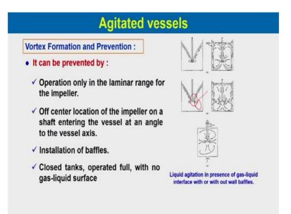
It can be prevented by different ways, one of them operation only in a laminar range for the impeller, but if you run the impeller in the laminar range then although it will not create the vortex, but the intimate no mixing between the gas and liquid will not enhance much. Off center location of the impeller on a shaft entering the vessel at an angle to the vessel axis.
