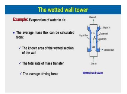
Like evaporation of water in air that is in case of humidification the average mass flux can be calculated from the known area of the wetted section of the column. So, so, as it is known thus the it is a film which is falling on the internal surface and this column can be made glass so, that you can see from the outside the no the film and you can control the flow rate and you can operate in the laminar as well as in the turbulent region.
