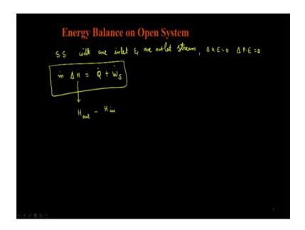
It will be m dot times delta H is going to be equal to Q dot plus W s dot. This delta H again stands for H of the outlet stream minus H for the industry. This is the energy balance on an open system at steady state condition with one inlet and one outlet
