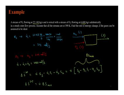
The first example says, we have a stream of nitrogen flowing at a certain flow rate and oxygen flowing as well and these two streams I have a stream of nitrogen and another stream of oxygen and what we get out is a stream of air or mixture of these two compounds. And we are interested in assuming the or sorry, we are interested in calculating the rate of entropy change for this particular process, right.
