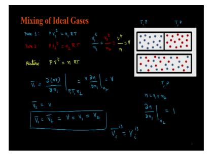
So, let us look at a example what exactly we mean by an ideal gas mixture over here, we have two gases which are separated by a wall in between. And at some time T equal to 0, we decide to remove this wall and then the gases are going to mix freely. Before mixing, we have pure species 1 and the P V t relationship for this pure species 1 is P 1 sorry, P V 1 t is n 1 R T.
