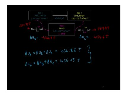
So, the trick then for these processes is to be able to come up with a path which can actually change the existing path to ones involving either a constant pressure or a constant volume process, so that I can use the information on C p and C v and calculate the necessary quantities. So, that is a quick demonstration of how I can use the specific heat capacity values for simple cases. With that we end todays lecture.
