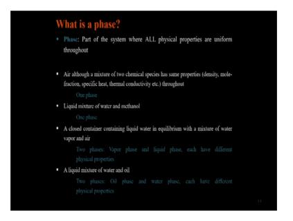
When we say number of phases what exactly is a phase? Phase is that part of the system with all the physical properties are uniform throughout. Physical properties such as density, mole fraction, thermal conductivity, viscosity whatever physical properties that might come to your mind all of them; it is not exclusive, we have to have it is exhaustive list all the physical properties need to be uniform throughout the part of the system we are calling as a single phase.
