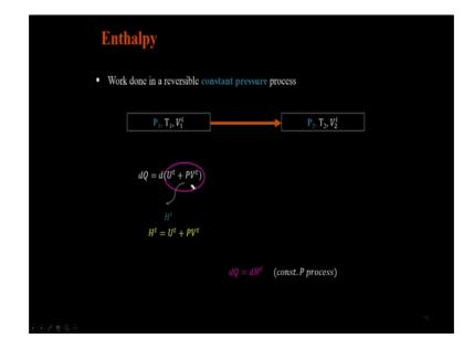
These processes are so important that we tend to give a particular, we assign a particular variable to this quantity U plus PV, we call it as enthalpy H right or in this case the total enthalpy H t, so U plus PV is often represented by the variable H or enthalpy. And in case of a constant pressure process then of course dQ is going to be equal to d H. And this quantity H will also have the same units as internal energy, so it will be in Joules.
