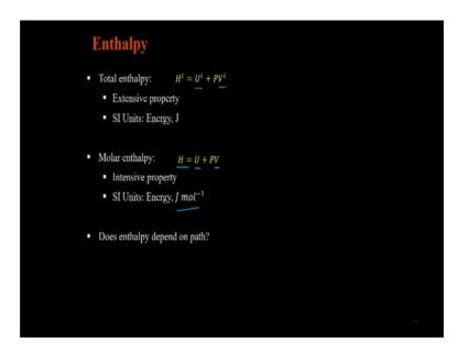
I can write a molar internal energy. So, instead of the total internal energy I can write the molar quantities H and then it will be related to the molar internal energy U and the molar volume V. So, instead of the total volume and total internal energy, if I write the expression for molar enthalpy it will be in terms of molar internal energy and the molar volume the units accordingly are going to be Joules per mole.
