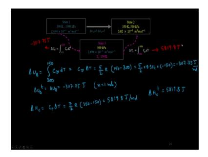
So, at state 3, once I choose the temperature pressure and volume, the temperature I can calculate to be a 150 Kelvin. So, now, I have all the steps sorted out, I also know the temperatures, I can write the expressions for delta U B and delta H c the temperatures are known, I just have to calculate the integral values.
