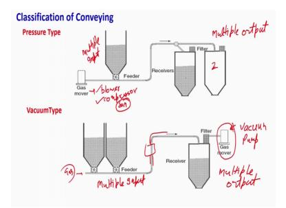
Now, one can do the same operation under the pressure or under the vacuum, we have already discussed that. So, suppose if you are want to do it under the pressure, so there is a gas mover. Gas mover can be it suppose you are doing the dilute phase transfer it can be blower. Gas mover is nothing but it can be blower, it can be compressor. And if needed even the fan, but fan is very, very difficult because the pressure generated by the fan is very very low.
