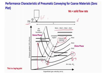
Now, to verify again many people have plotted this for different mass flow rate or different solid flow rates. So, if you see that W 1, W 2, W 3, W 4 is the solid flow rate different solid flow rate which is being operated W 4 is maximum if you see this and W 1 is minimum. Now, this is whatever I told you that this is only because of the air. If suppose there is no flow no solid flow is there only air is flowing inside the pipeline and
