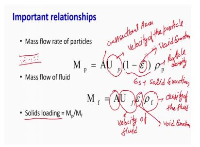
Now, we can also derive these things with the formula by writing the basic equations. So, what we can write here is that the first thing is that what will the mass flow rate of the particle. So, the mass flow rate of the particle can be given by this equation, where A is nothing but the cross sectional area, area. U p is nothing but the velocity of the particle; and epsilon is nothing but the void fraction. So, 1 minus epsilon will show you that this
