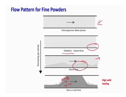
Now, the flow of fines as I said that the particle size also matters, so why it matters because the flow of fines and flow up the coarse particles are different. And the flow regimes for the fines is also different and flow regime in the case of the course particle is different. So, some of the regimes you will not see in the coarse particles, which you can see in the fine and some of the regimes you will not see in the fine particles, which you can see in the coarse.
