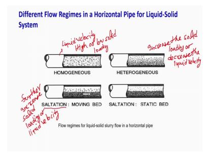
So, now first let us discuss about the hydraulic conveying which we say that liquid solid system. So, in a liquid solid system suppose if I have to convey the solid from one location to another location what will happen if the liquid velocity is high and solid fraction is lower. So, you can see that these curves whether the liquid velocity you are keep on reducing or solid loading you are keep on increasing.
