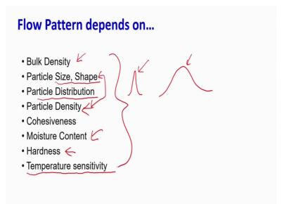
Now, the flow pattern inside you just not only depend on the velocity or the solid loading, it also depends on the many other factor and that again make the system more complicated and difficult to operate and design. The first thing which also matters is the bulk density that the solids which we are transporting, what is the density of that and what is the bulk density of the solid, we have already defined the bulk density.
