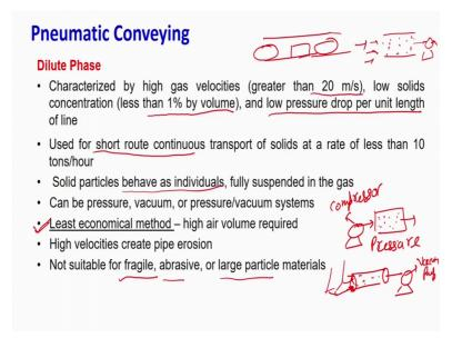
So, the whole pneumatic conveying as I said that dilute phase and dense phase is being divided in two parts. One is the dilute phase conveying; another one is the dense phase conveying. As the name suggests dilute phase conveying and we have already discussed it that the dilute phase conveying means the overall discrete phase fraction is very, very less.
