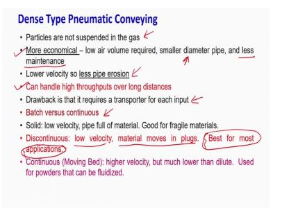
So, this is pneumatic conveying. As I said that you are seeing kind of particles are being suspended in the gas. So, it is not like any particles are being suspended; it will move in form of the dunes or in form of the slug or in form of the moving bed. So, particles are no more suspended in the gas phase that is called the dense phase. It is more economical, because now you require less air volume, and you are transferring more amount of the solids.
