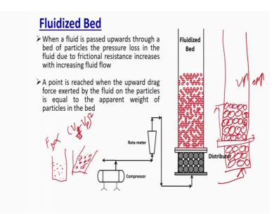
So, what is fluidized bed? The fluidized bed is nothing, but which is like a packed bed what we do there is a column in which we packed the solids, initially and then we pass the solid this gas or liquid or fluid I will say. The fluid is passed from the bottom towards
