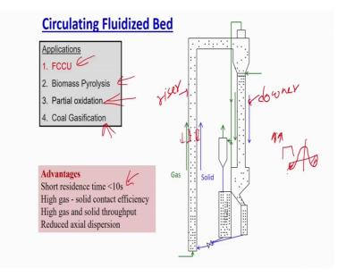
Then the last class is circulating fluidized bed where I said that what happen the particle entrainment rate is very high. So, it goes outside you have to catch the particle and put it back now this is very very important class of the rate can the fluidize bed and any fast reaction where the chances of the cooking is high where the kind of you want a properly controlled on the heat and mass transfer we use this kind of a bed.
