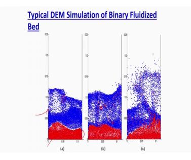
And, this is some typical DEM simulation we have performed in our lab and we have seen this is the red particle is heavier, blue particle is lighter you see initially the only both the particles are say fluidizing, but they are forming a clear cut interface, very small particles of the blue you can see inside here very small fraction of the solid you can see inside here if you keep on increasing the velocity some of the solid diffuses inside.
