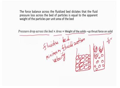
Now, as I said that the force balance across the bed actually states that the fluid pressure loss across the bed is equal to the apparent weight of the particle apparent weight of the bed and that is actually if per unit area if you will do if you do the force balance; then what you will happen you will see that that the pressure drop across the bed multiplied by the area.
