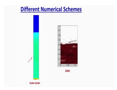
Then, different numerical schemes are being used as I said that because this is a dynamics governed this is depends on the bed behaviour is going to depend largely on the hydrodynamics in several kind of approach can be used to model this you can use different experimental method different modelling method you can use Euler-Euler in which you assume that both the fluid and the solids are in continuum.
