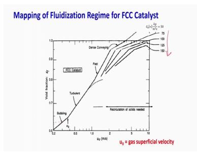
Then for FCC which is very critical actually people have plotted it again for the different velocity and the some numbers is given that if you keep on increasing the velocity. So, like you can see the bubbling fluidized bed occurs at a velocity of say 0.3 meter per second superficial gas velocity and at that case if you see that the bubble fraction or the void fraction is in the range of 0.65. So, it means you will have around 35 percent of the solids.
