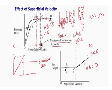
Now, the thing is as I said that if you keep on increasing the velocity what will happen in the packed bed reactor you will find some of this curve. So, this a curve. So, what will happen in the packed bed reactor if you keep on increasing the velocity the frictional losses is going to be increased and frictional pressure drop is going to increase. It means you keep on increasing the pressure drop.
