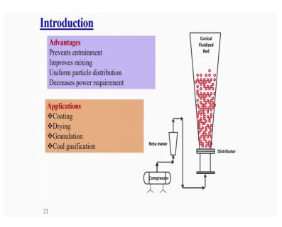
Now, another class of the fluidized bed which is being used widely in the industry is the conical fluidized bed. Now, this kind of a bed is being used for very coarse particles. If suppose I have a very coarse particle a particle say if I have to fluidize a tennis ball how to fluidize it we have minimum fluidization velocity will be very very high.
